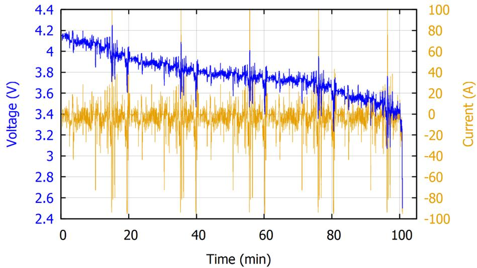
Figure 3: Total voltage and periodically repeated drive cycle current versus time, a full discharge.
