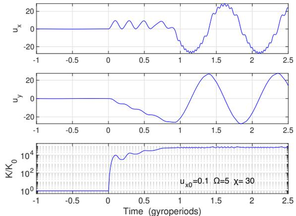
**Figure 2.** Acceleration of a particle in the bulk heating region (marked as ' $F_2$ ' in the colormap) with initial velocity  $u_{x0} = k_x r_c = 0.1$ ,  $u_{y0} = 0$  by wave  $\Omega = 5$  and  $\tilde{\chi} = 30$ . The wave is switched on at  $t = 0$ . Panels show velocity components  $u_x$ ,  $u_y$ , and the kinetic energy ratio  $K/K_0$ . Energy increase by a factor of  $10^4$  is achieved within half of the wave period, or 1/10 of the gyroperiod.
