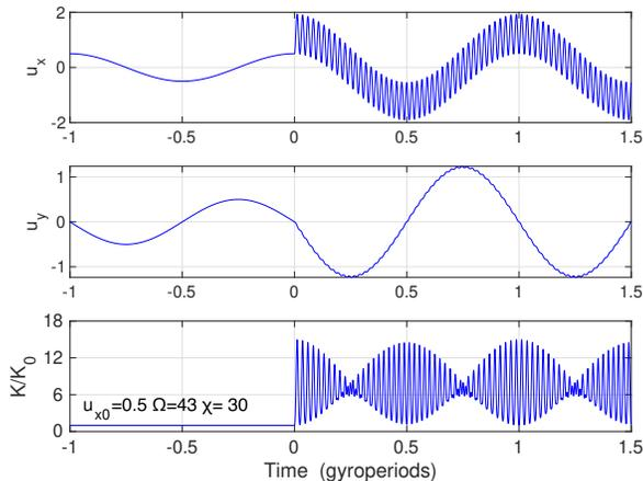
**Figure 4.** Acceleration of a low energy particle with  $u_{x0} = 0.5$  by a lower hybrid wave  $\Omega = 43$ ,  $\tilde{\chi} = 30$ . A proton is accelerated by a factor of 6 within 1/40 of the gyroperiod. The position in the colormap is marked as ' $F_4$ '.
