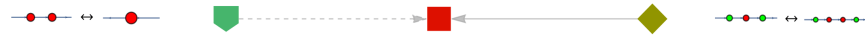
Figure 51: The proof graph corresponding to the proof of the lemma obtained by applying the X-spider fusion rule (S1) in order to fuse the phase- \beta X-spider from Alice's Bell measurement with the phase- \beta X-spider from Bob's classically-correlated corrections. Here, pointed light green boxes represent axioms, light orange circles represent substitution lemmas (i.e. instances of resolutions/factorings), and dark green diamonds represent hypotheses. Solid lines represent substitutions and dashed lines represent derived inference rules.
