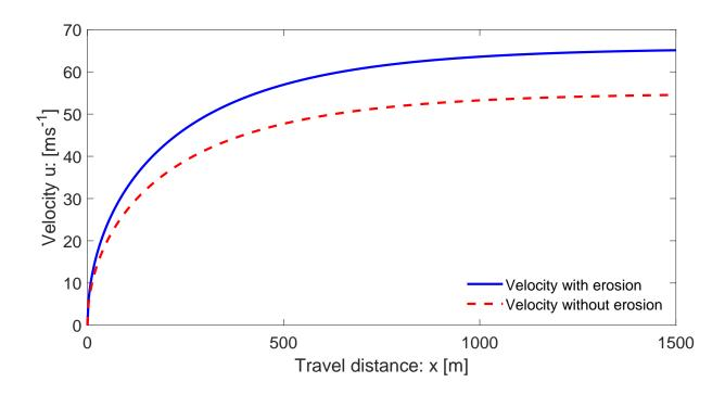
Figure 3: Evolution of the landslide velocity as a function of travel distance with and without erosion given by (24). Erosion enhances the landslide velocity and thus its mobility.
