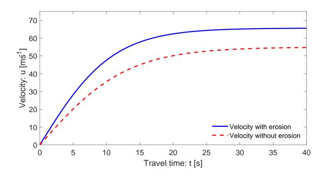
Figure 1: Time evolution of the landslide velocity with and without erosion given by (19). Erosion enhances the landslide velocity and thus its mobility. With erosion, the steady state velocity is higher and is reached earlier than the same without the erosion. This is due to the erosion-induced gain in momentum that increases the instantaneous velocity for which the drag takes shorter time to bring the motion to the steady-state, but with higher value.
