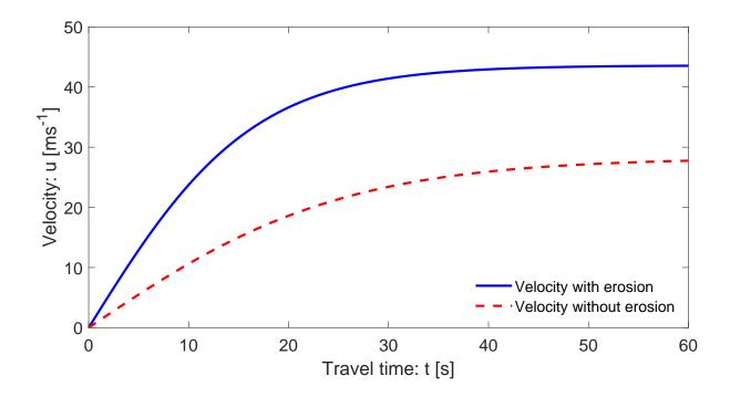
Figure 2: Time evolution of velocity with and without erosion for dry landslide given by (19). The landslide velocity, and thus its mobility, is largely enhanced by erosion.
