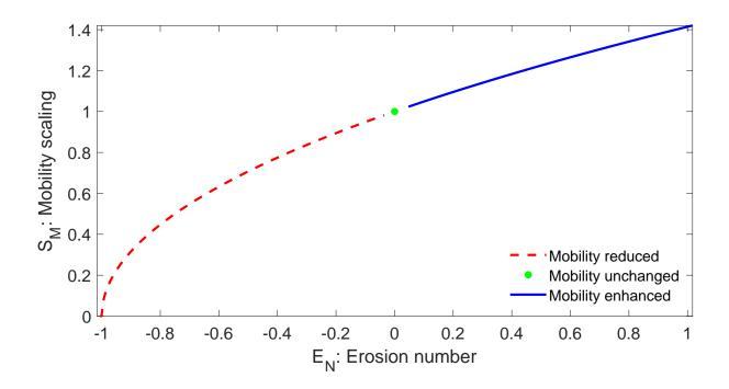
Figure 4: Non-linear dependency of the mobility scaling  $S_M$  on the erosion number  $\mathcal{E}_N$  given by (25) and (27). Three distinct mobility regimes are indicated.
