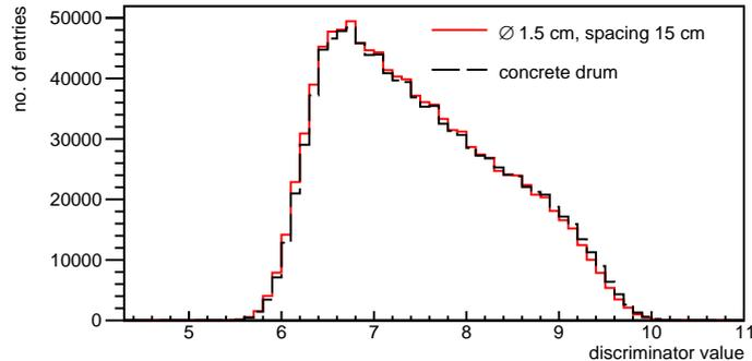
Figure 4: Discriminator distributions for a concrete block and a concrete block with single grid, where the bars' diameter was 1.5 cm.
