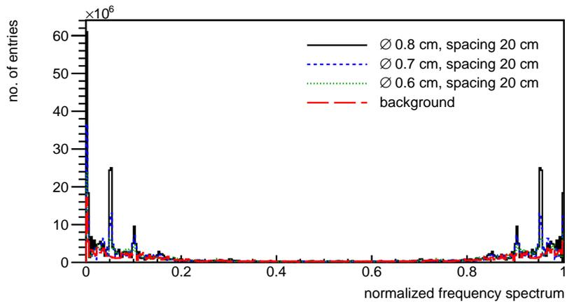
Figure 23: Normalized frequency spectrum for a reinforcement made of 6, 7 or 8 mm diameter bars and spacing of 20 cm. Time of data taking was increased to two weeks.
