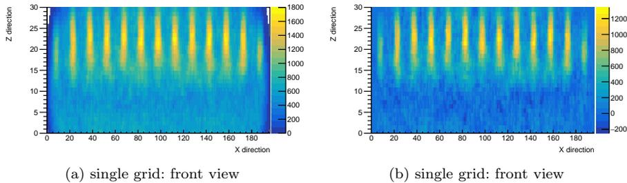
Figure 5: Result of the reinforcement imaging before (left) and after background subtraction (right) for a single grid using 1.5 cm diameter bars.
