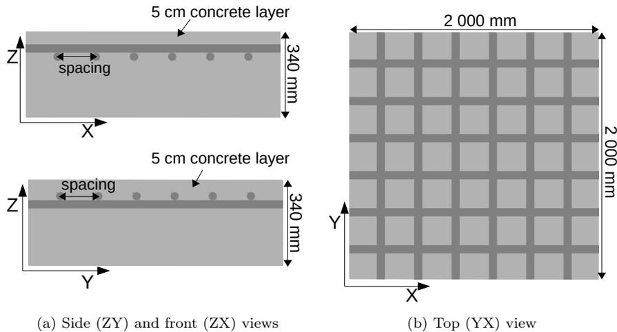
Figure 2: A schematic drawing of the concrete block used in the simulations. Inside, two layers of reinforcement bars, forming a single grid were placed.
