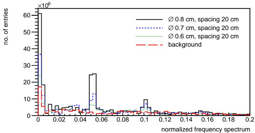
Figure 24: Zoomed, normalized frequency spectrum for a reinforcement made of 6, 7 or 8 mm diameter bars and spacing of 20 cm. Time of data taking was increased to two weeks.
