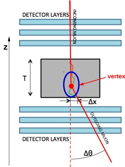
Figure 3: Incoming and outgoing muon tracks are reconstructed with RPCs. On their basis, the vertex is determined.
