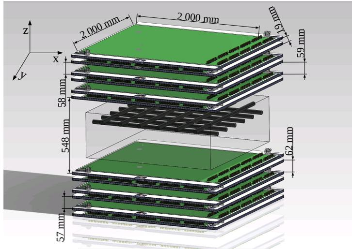
Figure 1: Schematic drawing of the simulated setup. RPCs are above and below the concrete block. Inside the concrete block a reinforcement grid is placed.
