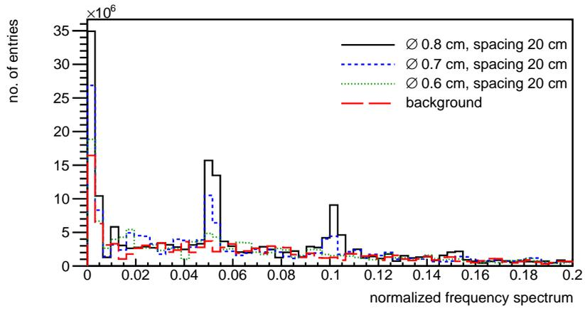
Figure 22: Zoomed, normalized frequency spectrum for a reinforcement made of 6, 7 or 8 mm diameter bars and spacing of 20 cm.
