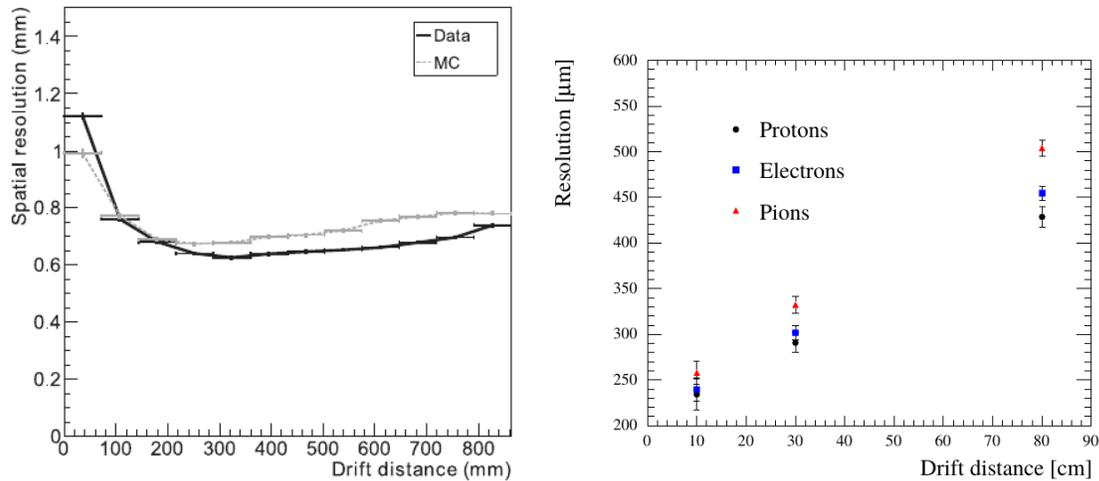
Figure 5.16: Left: spatial resolution of the vertical TPCs in ND280 with beam events. Right: spatial resolution obtained with a prototype of resistive Micromegas module on a test beam of 0.8 GeV positrons, pions and protons for different drift distances. Figures taken from ref. [150] and ref. [149].
