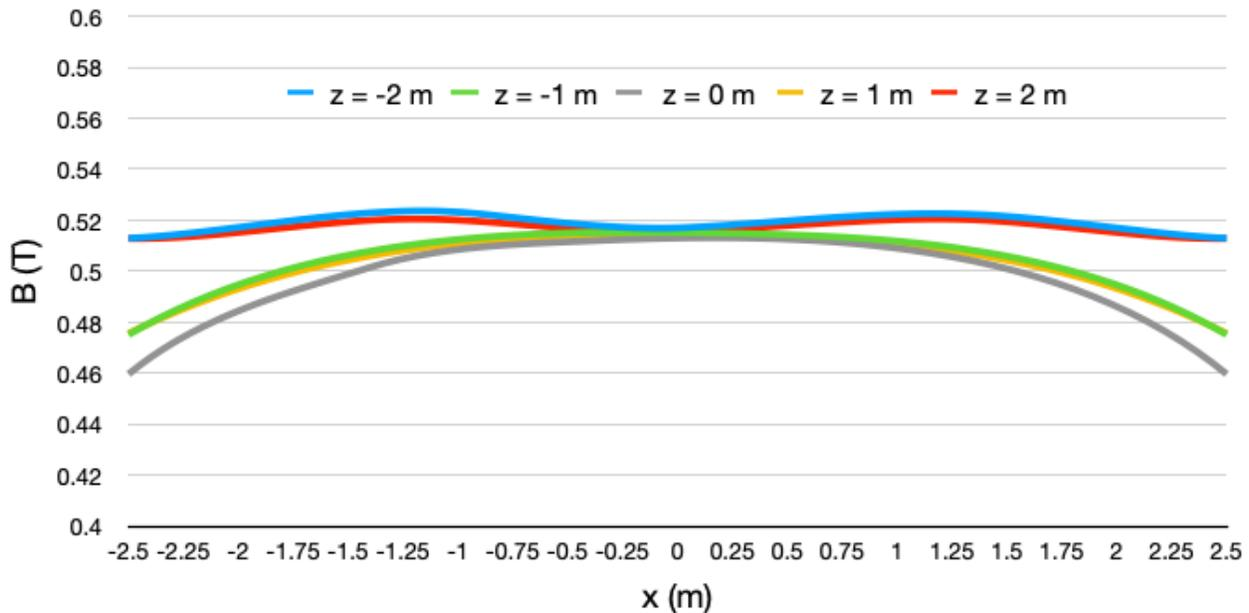
Figure 3.12: Field map for SPY along the axis of the solenoid ( $x$ ). The field is shown for different positions in the horizontal plane, ranging from  $z = -2$  m, in SAND direction, towards  $z = 2$  m, in LArTPC direction. Noticeably there is a small asymmetry due to the asymmetric distribution of iron in the yoke.
