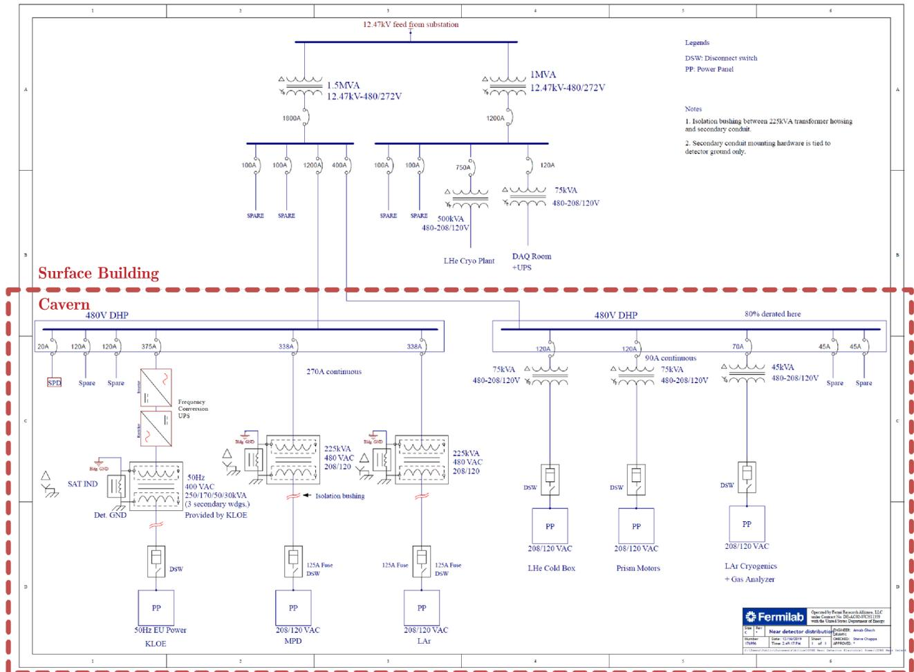
Figure 8.19: DUNE ND detector power distribution diagram.
