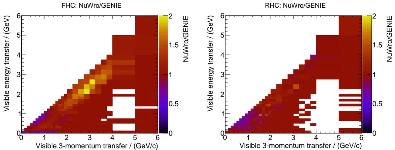
Figure 3.29: Left: Ratio of NuWro-reweighted HPgTPC  $\nu_\mu$  (FHC) sample to GENIE sample for all reconstructed events. Right: Ratio of NuWro-reweighted HPgTPC  $\nu_\mu$  (RHC) sample to GENIE sample for all reconstructed events. Bins with  $< 100$  true MC events are not filled.
