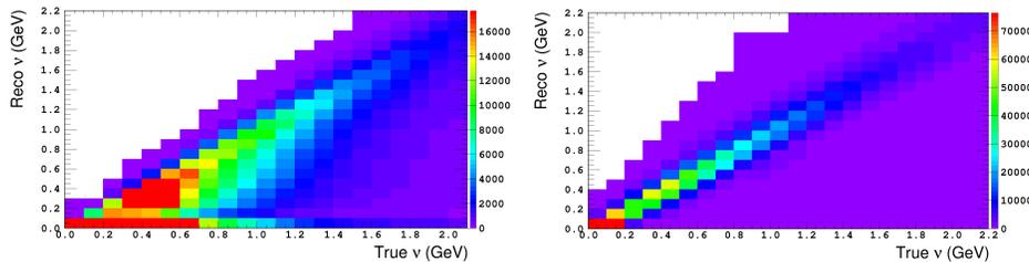
Figure 5.27: The reconstructed versus true  $\nu$  in 3DST.  $\nu$  is defined as the energy carried by all the particles except the charged lepton. The left figure shows the case where neutrons are not detected, while the right figure corresponds to the case where all the neutron energy is reconstructed via ToF.
