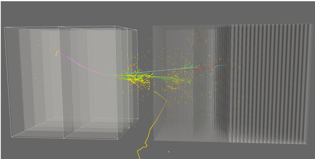
Figure 2.28: Example simulated event for a 7 GeV  $\nu_\mu$ -argon CC interaction, in which particles not contained in the ArgonCube 2×2 exit downstream, and are seen in the repurposed MINERvA detector components. Energy deposits are color-coded according to the particle type:  $\pi^\pm$  — blue;  $\mu^\pm$  — purple;  $e^+$  — green;  $e^-$  — yellow; proton — red; recoiling nuclei — black. The event vertex was randomly placed inside the active volume of the 2×2 Demonstrator module.
