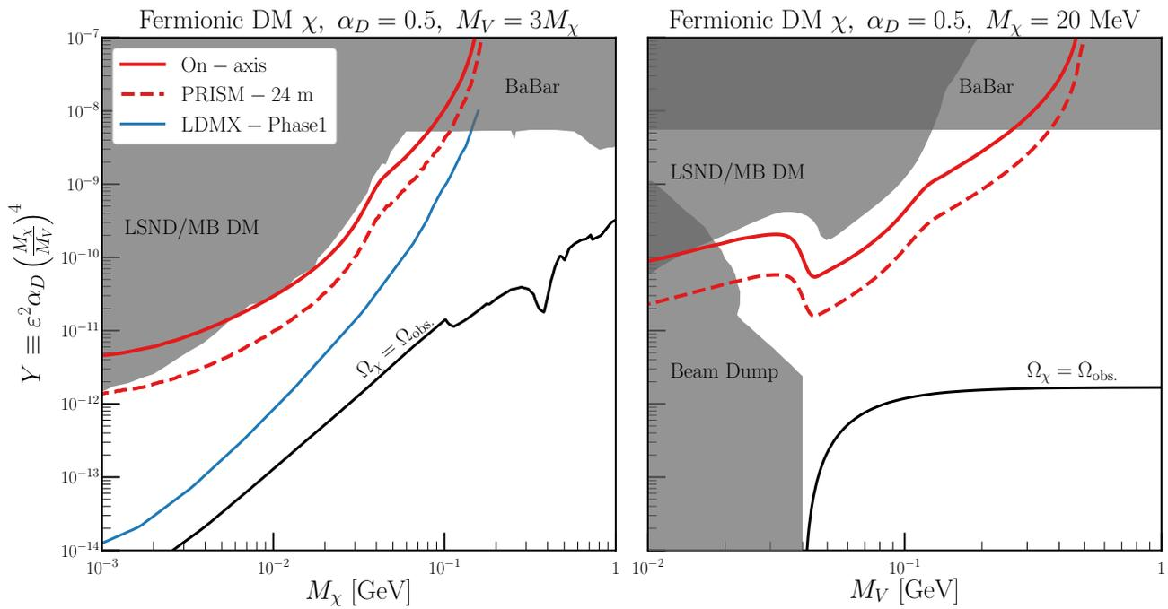
Figure 7.2: Expected DUNE On-axis (solid red) and PRISM (dashed red) sensitivity using  $\chi e^- \rightarrow \chi e^-$  scattering. We assume  $\alpha_D = 0.5$  in both panels, and  $M_V = 3M_\chi$  ( $M_\chi = 20$  MeV) in the left (right) panel, respectively. Existing constraints are shown in grey, and the relic density target is shown as the black line. We also show for comparison the sensitivity curve expected for LDMX-Phase I (solid blue) [241].
