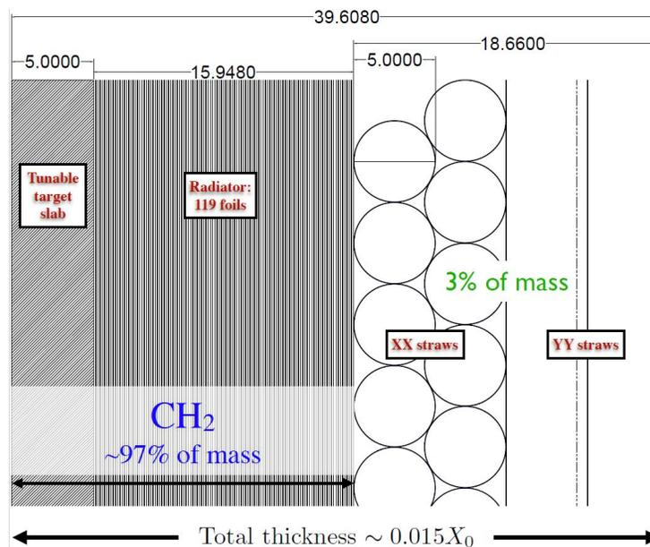
Figure 5.13: Drawing of a compact STT module including three main elements (left to right): (a) a tunable polypropylene  $\text{CH}_2$  target; (b) a radiator with 119 polypropylene foils for  $e^\pm$  ID; (b) four straw layers XXYY (beam along  $z$  axis and B field along  $x$  axis). Some of the radiator foils are replaced with thin carbon targets.
