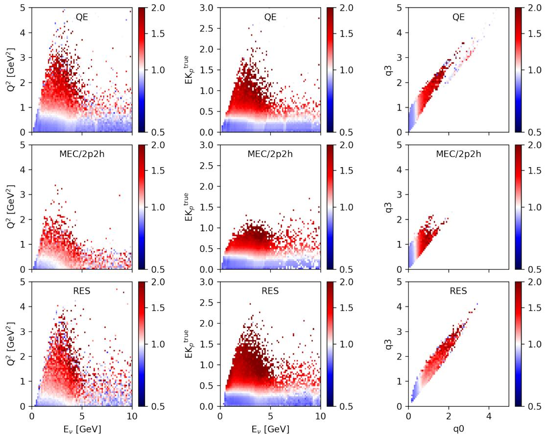
Figure 4.7: FHC event weights binned in interaction mode and three pairs of true kinematic variables: true neutrino energy vs  $Q^2$  (left); true neutrino energy vs true proton kinetic energy (middle); and  $q_0$  vs  $q_3$  (right).
