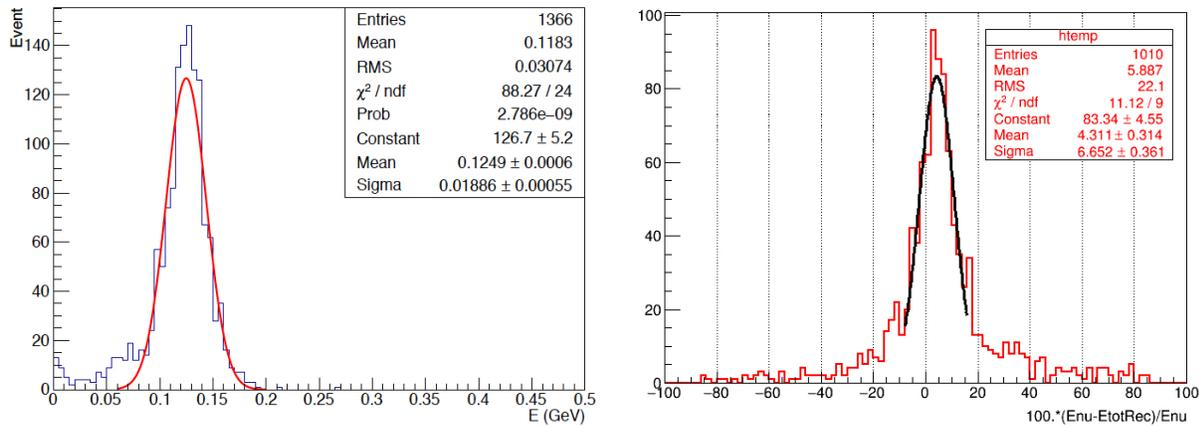
Figure 5.7: Left:  $\pi^0$ 's invariant mass computed using the ECAL information for  $\nu_\mu$  CC interactions with one  $\pi^0$ . Right: Reconstructed neutrino energy in  $\nu_\mu$  CC events using ECAL information.
