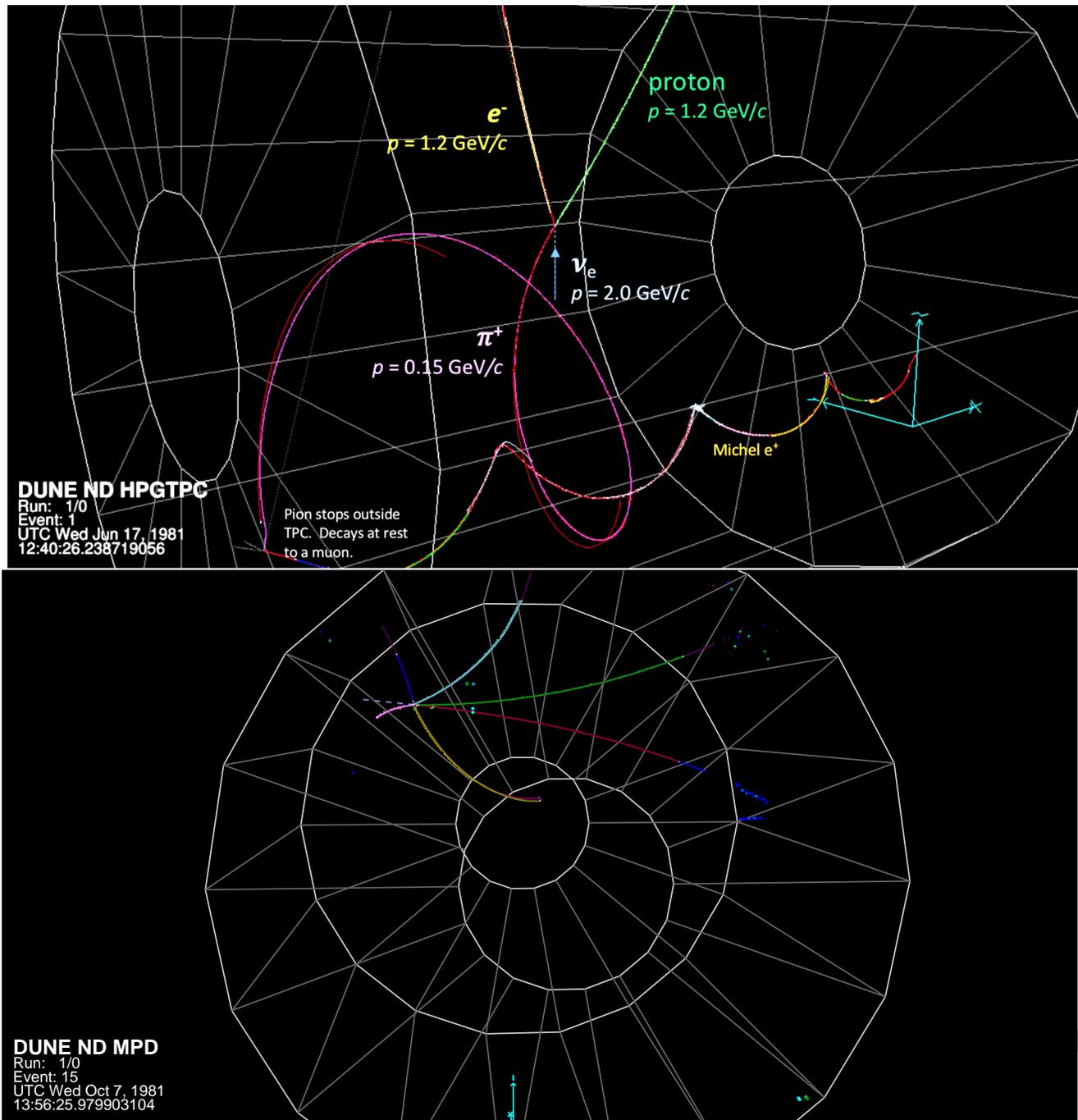
Figure 3.18: (Top) Track-reconstructed  $\nu_e$  CC event in the HPgTPC, simulated and reconstructed with GARSoft. The annotations are from MC truth. (Bottom) Track-reconstructed  $\nu_\mu$  CC event with five protons.
