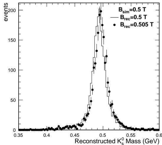
Figure 3.17: The invariant mass distribution for reconstructed  $K_s^0 \rightarrow \pi^+ \pi^-$  decays. The  $K_s^0$  were generated as single particle events inside the HPgTPC and then reconstructed in GARSoft with an efficiency of about 33%. The kaon mass ( $m_{K_0} = 497.6$  MeV according to the PDG) is well reproduced by the mean of the distribution, and a 1% bias in the magnetic field (and therefore also in the momentum) results in a clear shift of the mean.
