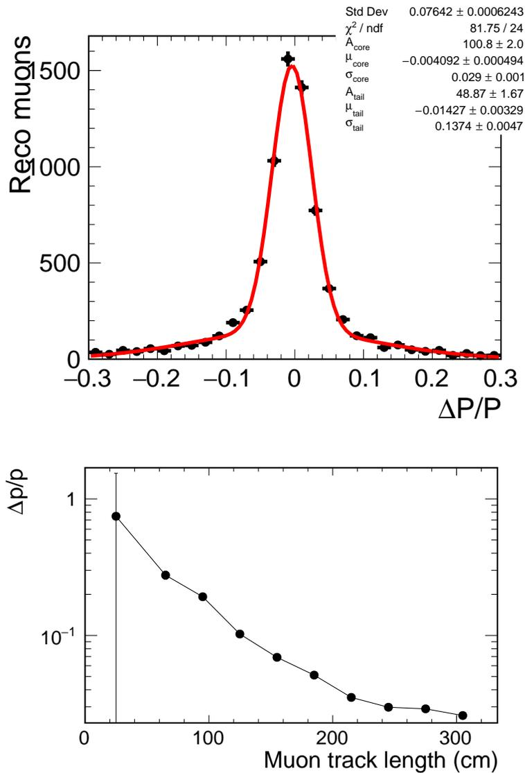
Figure 3.23: Top: the momentum resolution for reconstructed muons in GArSoft, in a sample of  $\nu_\mu$  CC events. The events were generated using the LBNF flux. The Gaussian fit to the central core of the  $\Delta p/p$  distribution, containing 2/3 of events, has a width of 2.7%. The tails are well described by a 12% resolution. Bottom: The momentum resolution as a function of track length.
