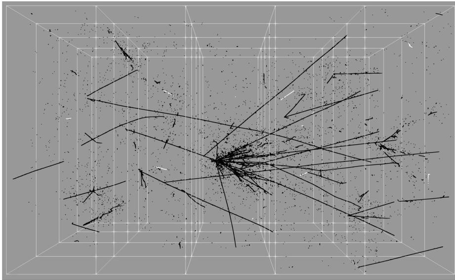
Figure 2.20: A beam spill in ND-LAr. Fast-neutron induced recoiling proton tracks, with an energy threshold greater than  $\sim 10$  MeV, are shown in white. The black tracks are all other energy deposits sufficient to cause charge collected at the pixel planes.
