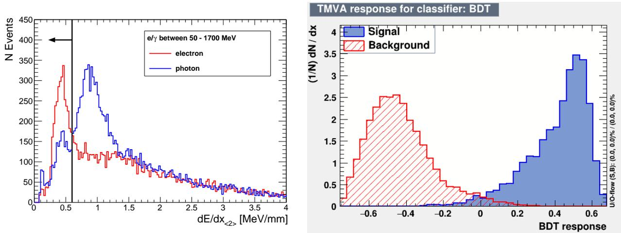
Figure 3.37: On the left:  $e/\gamma$  discrimination using  $\frac{dE}{dX}$  in the two first planes of the ECAL. On the right, BDT classifier output separating 1 GeV/c positrons (signal) and protons (background).
