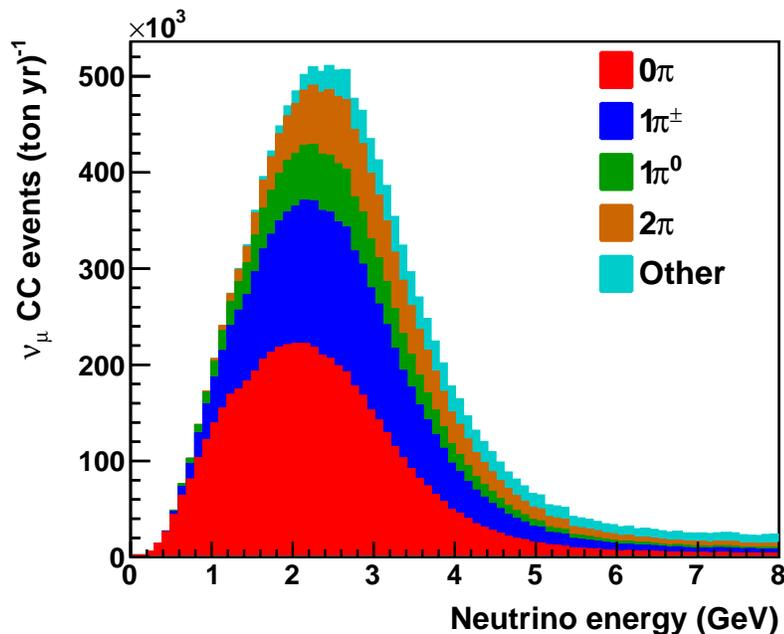
Figure 6.5: CC  $\nu_\mu$  event rates on argon by interaction type expected in the DUNE ND. The simulation corresponds to  $1.97 \times 10^{21}$  protons on target in the forward horn current mode (one spill per second for a year).
