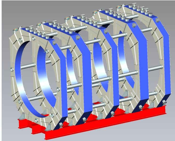
Figure 3.13: 5-coil Helmholtz concept for ND-GAr superconducting magnet.
