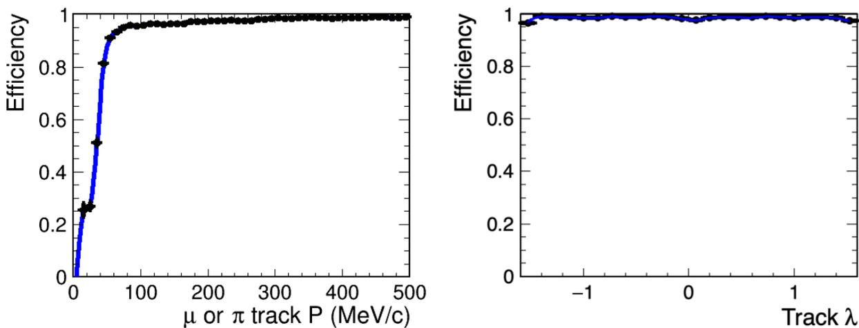
Figure 3.19: (Left) The efficiency to find tracks in the HPgTPC as a function of momentum,  $p$ , for tracks in a sample of Generates Events for Neutrino Interaction Experiments (GENIE) events simulating 2 GeV  $\nu_\mu$  interactions in the gas, using GArSoft. (Right) The efficiency to find tracks as a function of  $\lambda$ , the angle with respect to the center plane, for tracks with  $p > 200$  MeV/ $c$ .
