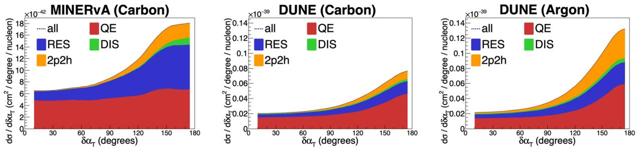
Figure 6.10: Differential cross section in the transverse boosting angle,  $\delta\alpha_T$ , as defined in Equation 6.15, for MINERvA (left) and for argon (right) in ND-GAr. The middle plot is for a carbon detector with the acceptance of ND-GAr to separate the detector design from the nucleus for the comparison.
