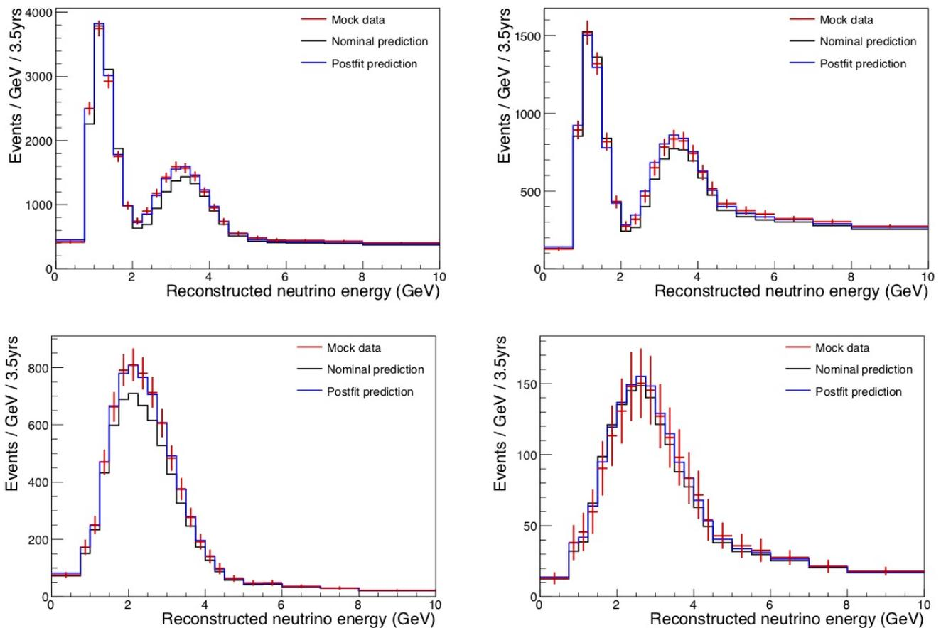
Figure 4.9: Predicted distributions of reconstructed neutrino energy for selected  $\nu_\mu$  (top) and  $\nu_e$  (bottom) events, in FHC (left) and RHC (right) beam modes in 7 years. The black curve shows the nominal GENIE prediction, the red points are the mock data samples, and the blue curve is the post-fit result, where systematic and oscillation parameters are shifted to match the mock data. The ND spectra match the pre-fit prediction by construction and are not shown.
