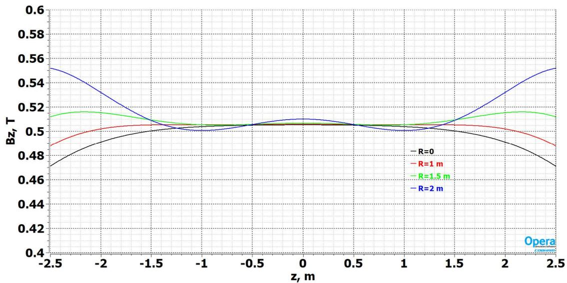
Figure 3.14: Field map of the 5-coil Helmholtz superconducting magnet along the  $z$  axis. The colors represent different radii from the center line. The horizontal scale shows the position along the symmetry axis of the magnet (called  $z$  here). The vertical scale shows the component of the magnetic field in the direction of the symmetry axis.
