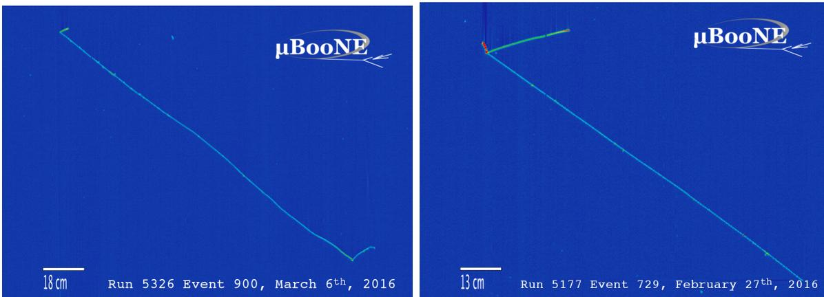
Figure 6.6: Event displays from the MicroBooNE liquid argon detector, showing the excellent ability to distinguish  $CC0\pi$  (left) and  $CC1\pi^\pm$  (right) charged-current  $\nu_\mu$  scattering events
