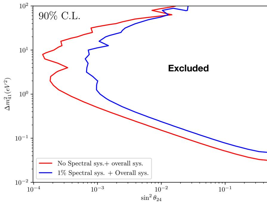
Figure 7.8: The 90 % CL DUNE ND-only  $\theta_{24}$  exclusion regions when including normalization systematics, but no spectral shape systematics (red curve), and when including normalization and shape systematics. Both curves were computed using the GLOBES toolkit assuming a 3+1 model with one sterile neutrino. For reference, the projected DUNE limits significantly exceed the current limits from MINOS [266] and IceCube [267] over much of the  $\Delta m_{41}^2$  range.
