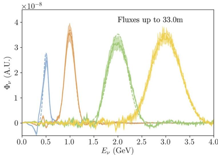
Figure 4.20: Linear combinations of ND  $\nu_\mu$  off-axis fluxes used to produce Gaussian incident neutrino energy spectra. These are shown for four different selected energies, each with a 10% width.
