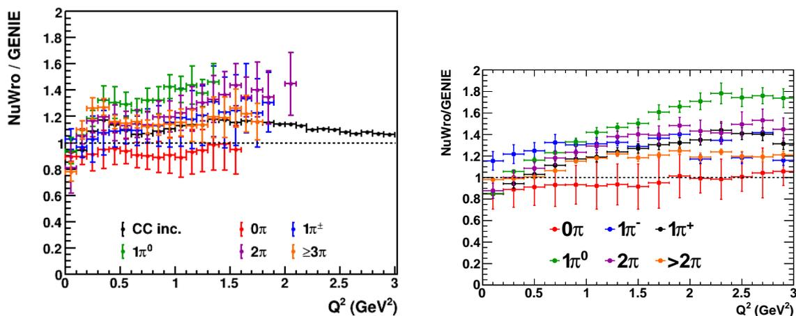
Figure 6.8: The ratio of the reconstructed  $Q^2$  distributions for  $\nu_\mu$  CC events for the NuWro and GENIE generators. Plots are shown for the ND-LAr (left) and ND-GAr (right), for final states including no pions (red),  $1\pi^\pm$  (blue),  $1\pi^0$  (green), 2 pions (purple) and 3 or more pions (orange).
