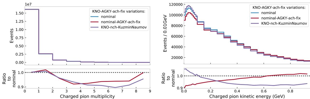
Figure 6.3: GENIE predictions for charged pion multiplicity (left) and kinetic energy (right) in the total CC  $\nu_{\mu}$  inclusive sample using the variations on AGKY's  $\langle n_{ch} \rangle$  described in the text.
