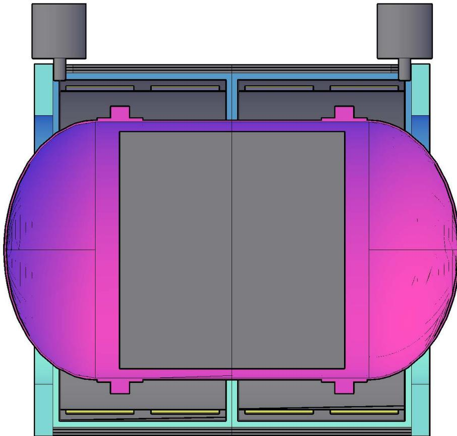
Figure 3.11: Solenoid arrangement for ND-GAr superconducting magnet.
