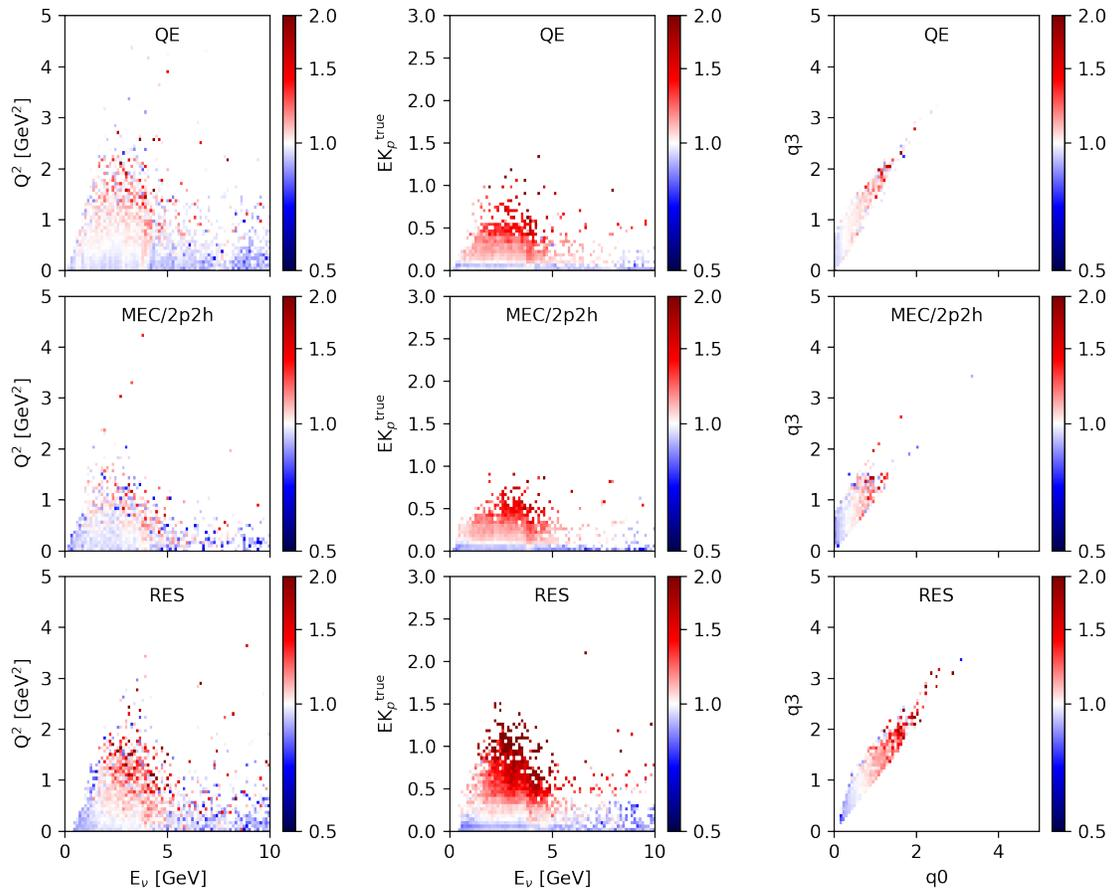
Figure 4.8: RHC event weights binned in interaction mode and three pairs of true kinematic variables: true neutrino energy vs  $Q^2$  (left); true neutrino energy vs true proton kinetic energy (middle); and  $q_0$  vs  $q_3$  (right).
