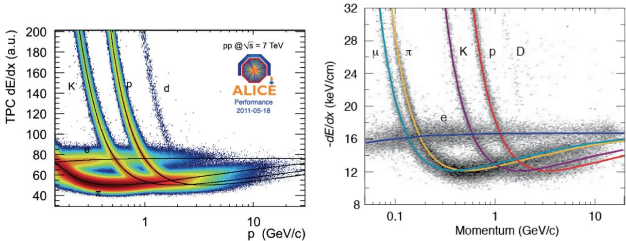
Figure 3.21: Left: ALICE TPC  $dE/dx$ -based particle identification as a function of momentum (from [116]). Right: PEP-4/9 TPC (80:20 Ar-CH<sub>4</sub>, operated at 8.5 Atm, from [115])  $dE/dx$ -based particle identification.
