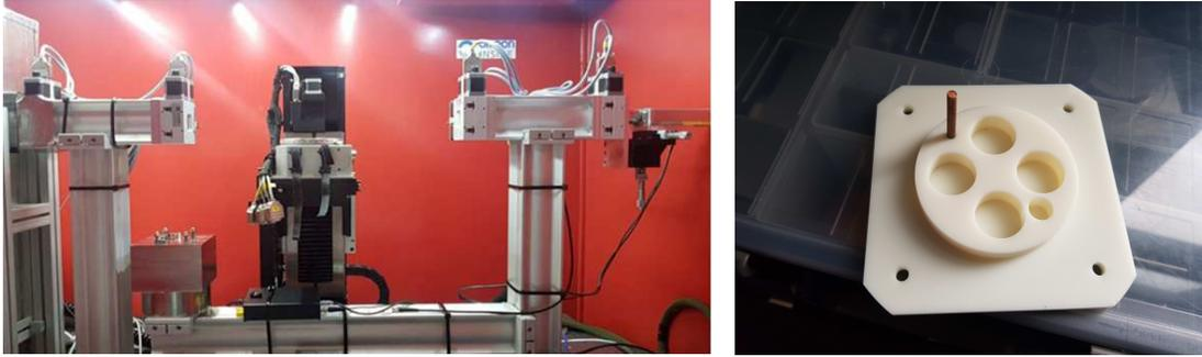
Figure 7: (a) Scanner setup and (b) support specimen for the cylinders of different materials.
