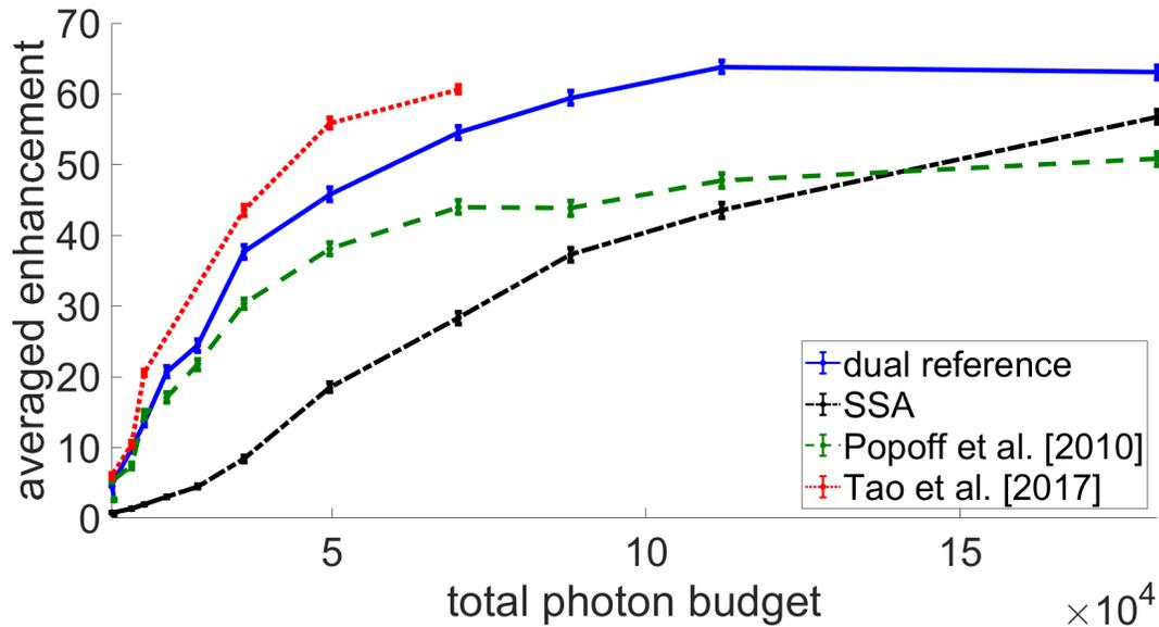
Figure 4: The measured averaged enhancement versus the total photon budget for dual reference algorithm (blue solid curve), SSA (black dash-dot curve), Popoff et al. [10] (green dash curve), and Tao et al. [12] (red dot curve). Bars represent the standard error of the measurement set.
