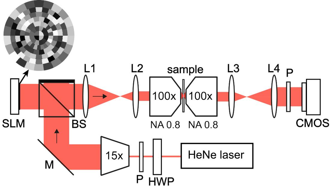
Figure 2: Schematic of the experimental setup. HWP, half-wave plate; M, mirror; BS, 50% non-polarizing beam splitter; P, polarizer; CMOS, complementary metal oxide semiconductor camera; L1, L2, L3 and L4, lenses with focal length of respectively 200 mm, 75 mm, 75 mm and 150 mm. The inset shows a random wavefront displayed on the modulating segments of the SLM.
