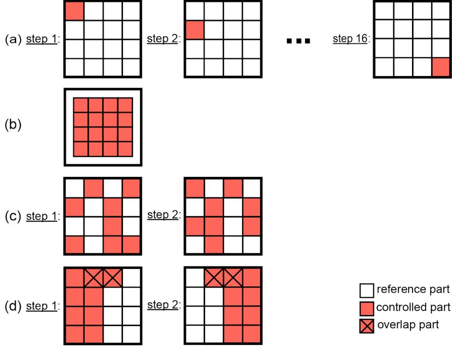
Figure 1: Feedback based wavefront shaping algorithms. (a) Stepwise sequential algorithm: a single segment (in red) is controlled in every step. (b) Popoff et al. [2010] algorithm: always 65% of the SLM segments are controlled. (c) Tao et al. [2017] algorithm: in every step half of the segments are controlled. (d) Dual reference algorithm: First, a group of segments is modulated (in red), and in the second step the rest of the segments plus some overlap segments (crossed) are modulated.
