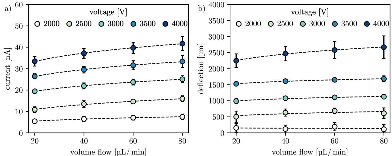
FIG. 4. Measured current (a) and deflection (b) as a function of the volume flow  $Q$  and the applied potential difference  $\phi$ . The silicone oil viscosity was 5 cSt and the KCl concentration of the spray 1 mM. Error bars represent the standard deviation of 5 measurements per datapoint. The dashed lines represent fit functions of the form  $y = ax^b$  to guide the eye.
