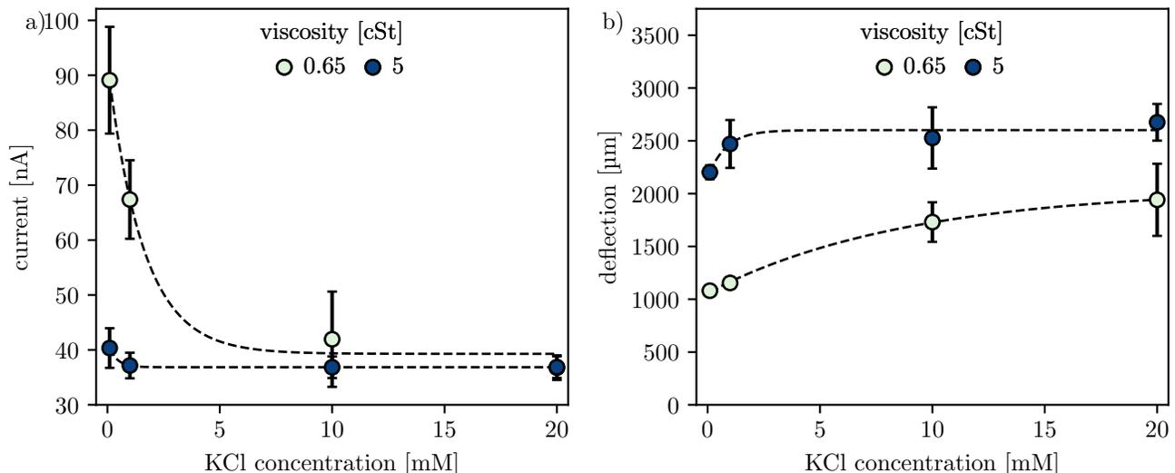
FIG. 6. Measured current (a) and interface deflection (b) as a function of the KCl concentration and the oil viscosity for a fixed volume flow of  $40 \mu\text{L min}^{-1}$  and a voltage of 4000 V. Error bars represent the standard deviation of 5 measurements per data point. The dashed lines represent exponential fit functions to guide the eye.
