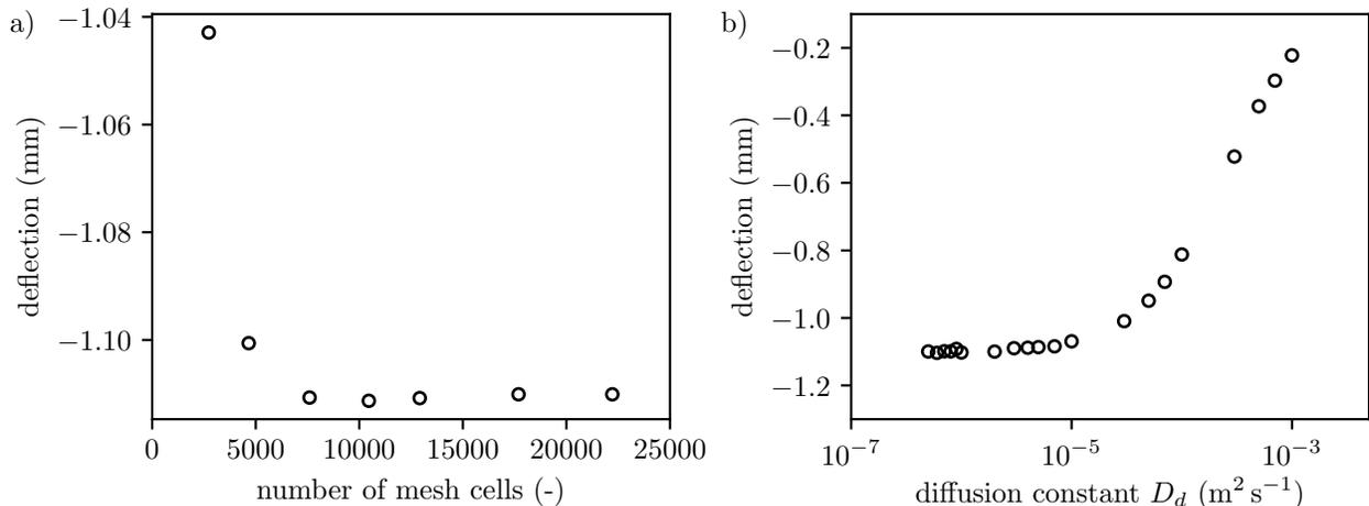
FIG. 10. Dependency of the solution on numerical parameters, expressed as the interface deflection as a function of these parameters. a) Influence of the number of mesh cells. b) Influence of the diffusion constant  $D_d$ .
