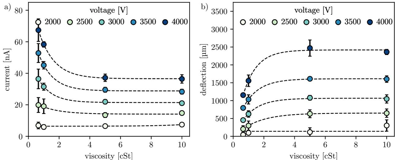
FIG. 5. Measured current (a) and deflection (b) as a function of the silicone oil viscosity and the applied voltage  $\phi$ . The volume flow was  $40 \mu\text{L min}^{-1}$  and the KCl concentration of the spray  $1 \text{ mM}$ . Error bars represent the standard deviation of 5 measurements per datapoint. The dashed lines represent exponential fit functions to guide the eye.
