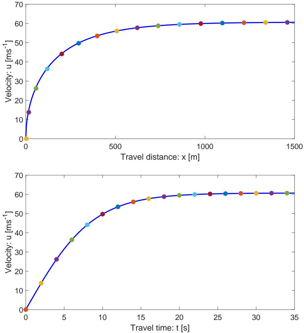
Figure 13: Spatial (top) and temporal (bottom) transportations of the initial velocity ( $u = 0$ ) of the landslide down the slope by the general solution system (39)-(40) as indicated by the star markings for times  $t = 0.0$  s, with 2.0 s increments. These solutions exactly fit with the space and time evolutions of the velocity fields for the mass point motions given by (8) and (11).
