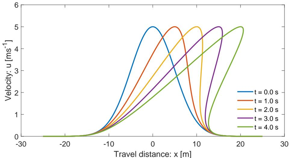
Figure 15: Recovering the Burgers’ shock formation and breaking of the wave by the solution system (39)-(40) of the new model (5) in the limit of the vanishing external forcing, i.e.,  $\alpha \rightarrow 0, \beta \rightarrow 0$ .
