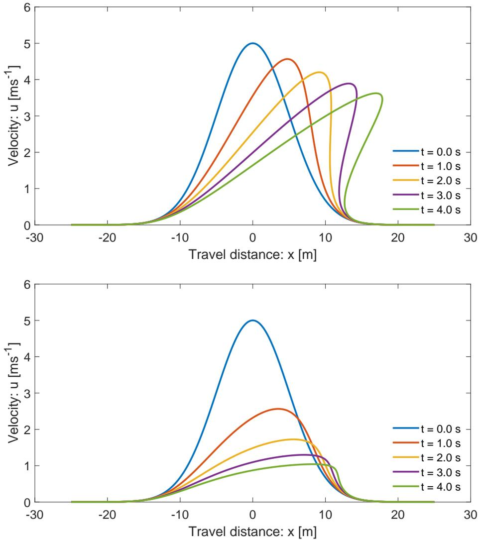
Figure 16: The control of the viscous drag on the dynamics of the landslide. The net driving force is set to zero, i.e.,  $\alpha = 0$ . The viscous drag has been amplified by one and two orders of magnitudes in the top ( $\beta = 0.019$ ) and bottom ( $\beta = 0.19$ ) panels, showing dampened or complete prevention of shock formation and wave breaking, respectively.
