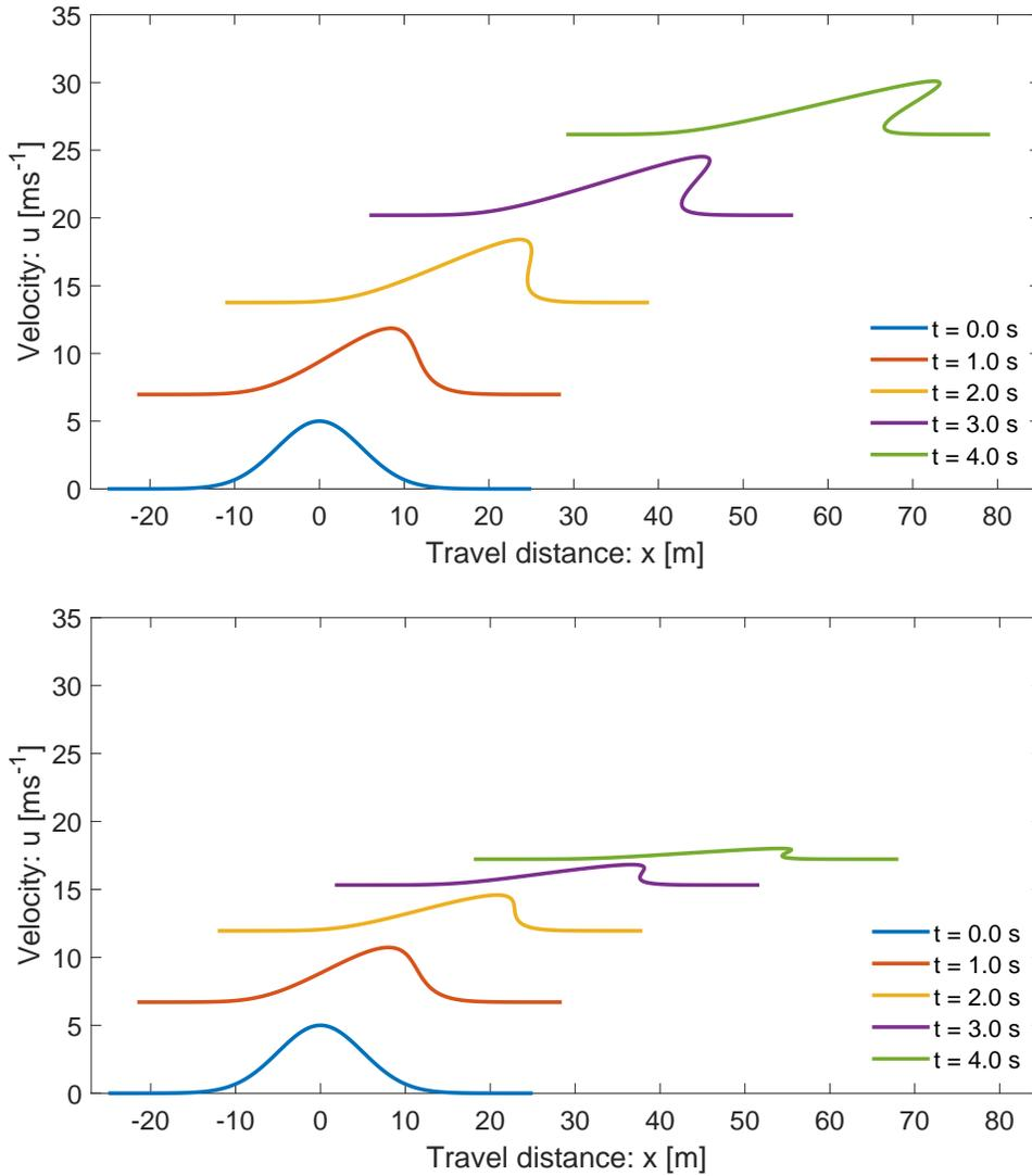
Figure 14: The breaking wave and folding as a landslide propagates down a slope. The top panel with drag  $\beta = 0.0019$ , while the bottom panel with higher drag,  $\beta = 0.019$ , which strongly controls the wave breaking and folding, and also the magnitude of the landslide velocity.
