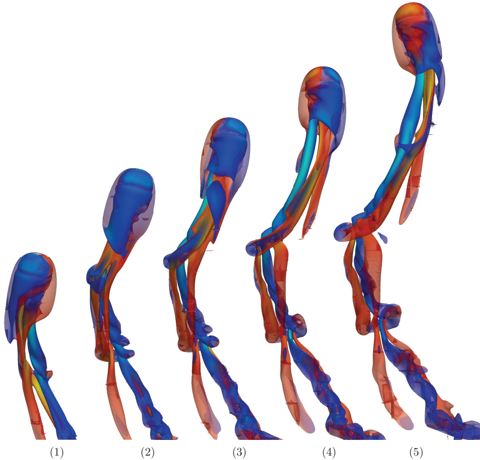
FIGURE 14 Case 15: Vortices behind a sphere of density ratio 0.05 at Ga = 500 . In frames 4 and 5 the three vortex threads delivering a constant torque to the ascending sphere are well visible. A Q criterion threshold of 10^{-10} is employed and coloring is done by normalized vorticity, which ranges between -10 (blue) and 10 (red). Lighter colors correspond to stronger magnitude.
