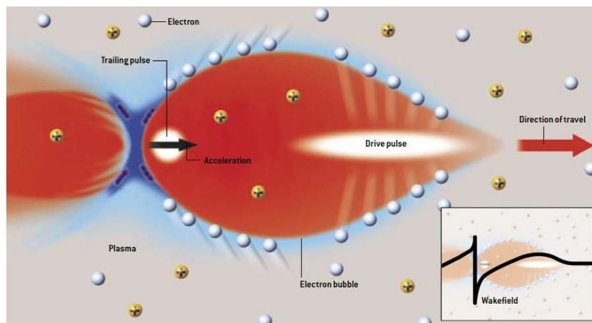
Fig. 5: Conceptual drawing of the plasma wakefield accelerator [19].
