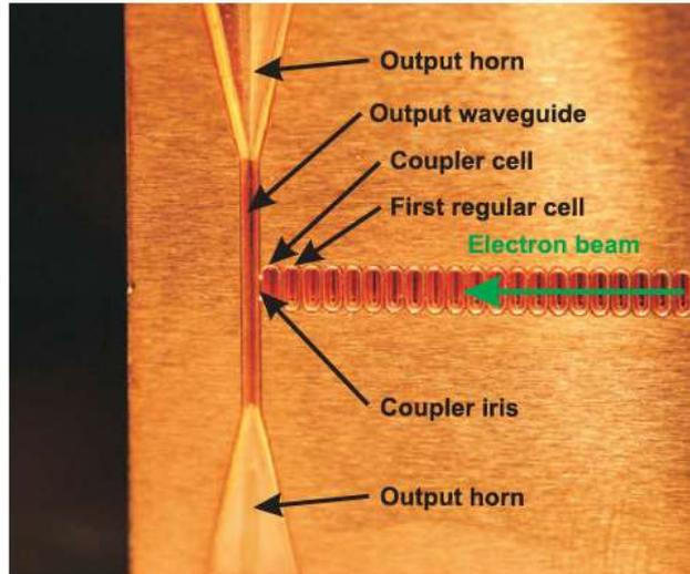
**Fig. 2:** The mm-wave traveling wave accelerating structure with detail of the output part, including coupler and output waveguides [8].
