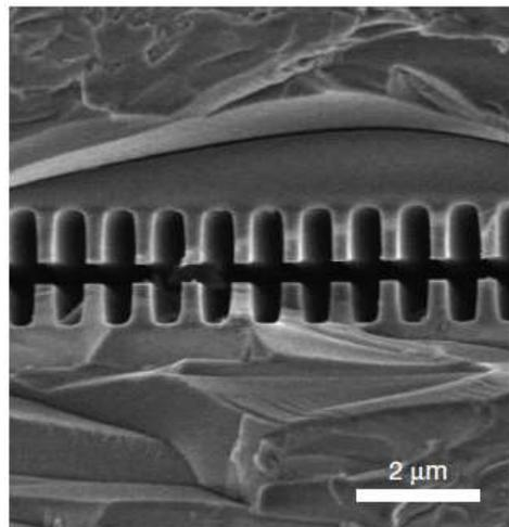
**Fig. 4:** Scanning electron microscope image of the longitudinal cross-section of a DLA structure [14].
