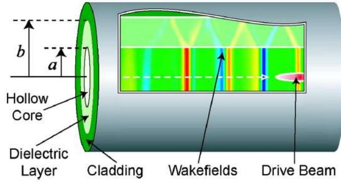
**Fig. 3:** Conceptual drawing of the dielectric wakefield accelerator (DWA) [12],  $a = 50 \mu\text{m}$ ,  $b = 162 \mu\text{m}$ .
