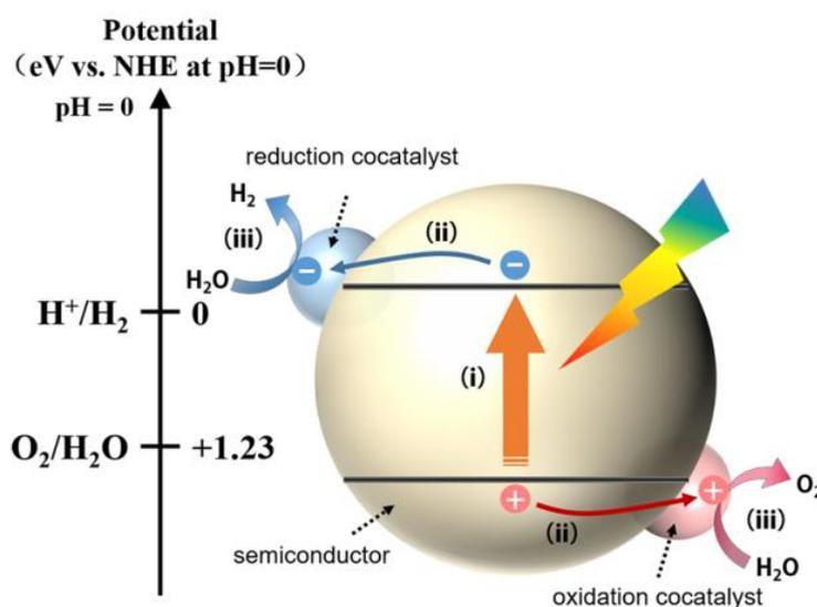
**Fig. 1** Schematic diagram of the mechanism of photocatalytic water splitting containing 2 parts (semiconductor photocatalysts and cocatalysts loaded on the photocatalysts) and 3 steps ((1) light absorption; (2) separation and transfer of charge carriers (electrons and holes); (3) photo-induced hydrogen and oxygen evolution reactions on the surface).<sup>[7]</sup>
