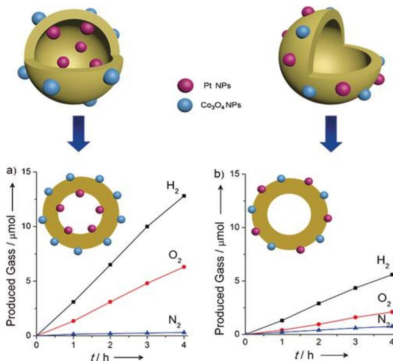
**Fig. 4** Comparison of time courses of photocatalytic evolution of H<sub>2</sub> and O<sub>2</sub> using **a)** Co<sub>3</sub>O<sub>4</sub>/HCNS/Pt and **b)** (Co<sub>3</sub>O<sub>4</sub>+Pt)/HCNS under UV irradiation ( $\lambda > 300$  nm) in Wang's group<sup>[42]</sup>.
