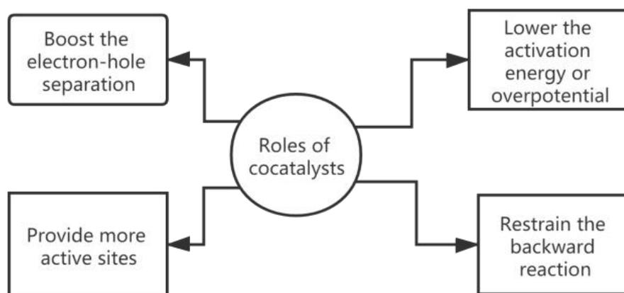
**Fig. 2** Four roles of cocatalysts in photocatalytic H<sub>2</sub>/O<sub>2</sub> generation via water dissociation on the semiconductor surface
