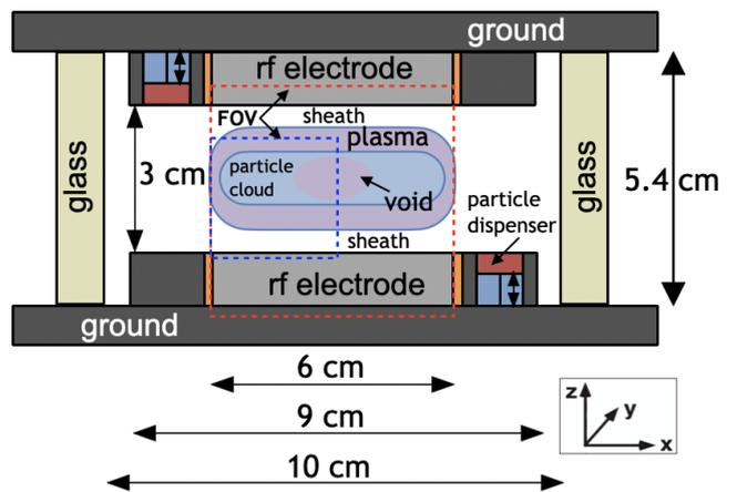
FIG. 2. Sketch of the PK-3 Plus chamber seen from the side [20]. The fields of view (FOV) of the overview (red dashed line) and quadrant view (blue dashed line) cameras are shown which were used for the analysis of our experiments: Fig. 1 (overview) and Figs. 5, 6, 3 (quadrant view). Typically a particle free region (the so-called “void”) formed almost at the center of the particle cloud under microgravity conditions.
