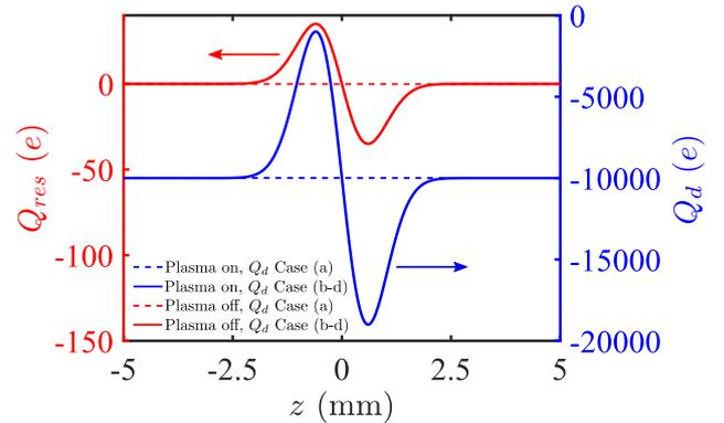
FIG. 8. Dust particle charges as a function of their position at plasma extinction (blue curves) and after decharging (red curves). The decharging time was set to  $\tau_D = 1$  ms.
