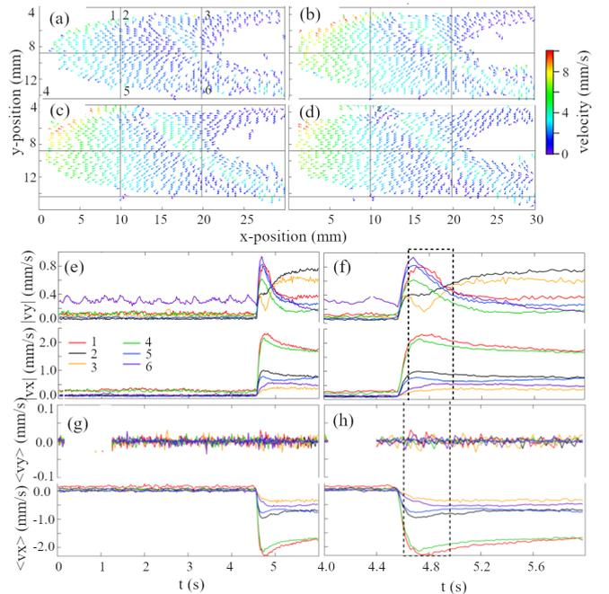
FIG. 6. (a)-(d) PIV analysis for the uni-directional pulse in Exp. I at different times after the plasma switched off. The time step between panels (a)-(d) is 0.1 s. For display purposes, only every third vector is shown. All vectors are drawn with the same length, and their color represents their velocities. The field of view is divided into 6 regions, indicated by solid lines. (e)-(h) Absolute and average horizontal and vertical velocities in the regions defined above as a function of time.
