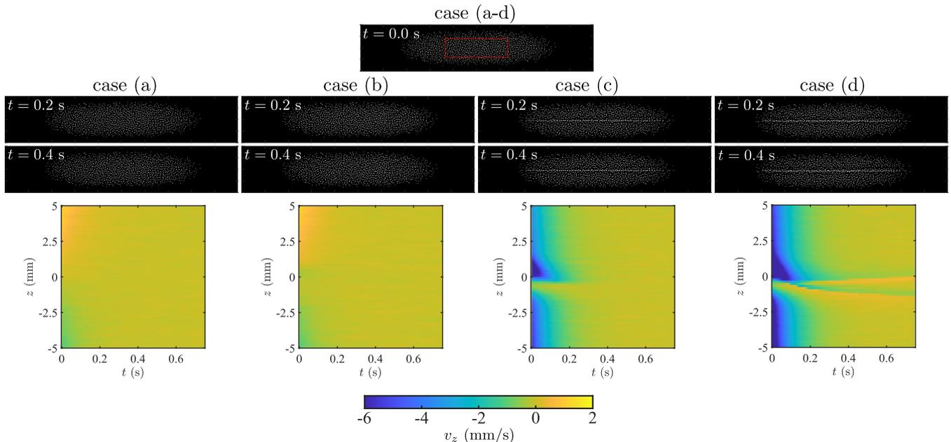
FIG. 9. Snapshots of the simulated microparticle cloud configuration at different times in the post-discharge and average vertical velocity map as a function of vertical position and time for the different investigated post-discharge scenarios. In the upper snapshot at  $t = 0.0$  s, the dashed red rectangle represents the region used to average velocity maps.
