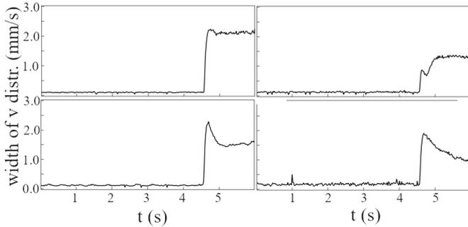
FIG. 7. Time evolution of the width of the PIV velocity distributions for Exp. I for Regions 2, 3, 5 and 6 (corresponding to Fig. 6). In Regions 1 and 4, the leftmost regions of the images, we were unable to obtain reliable fits to the distribution function.
