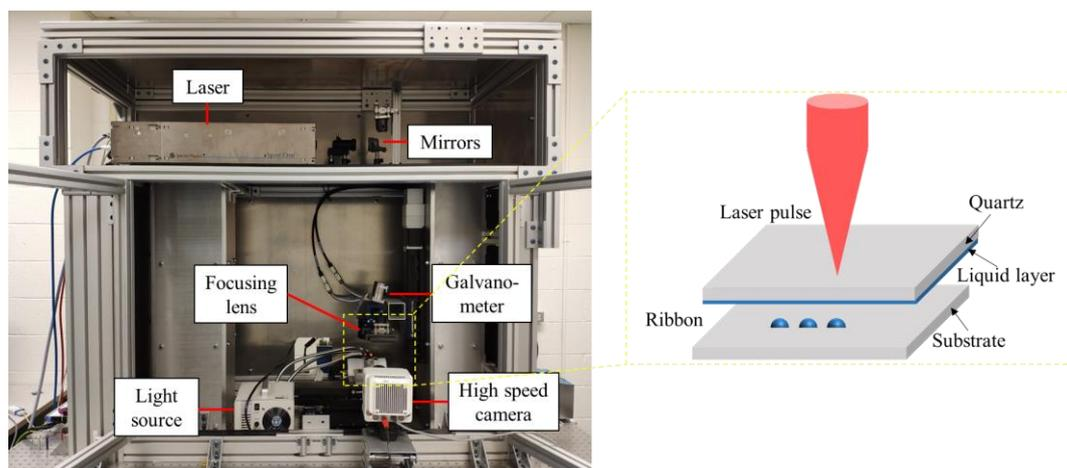
*Fig. 2. Experimental platform of LIFT process*
