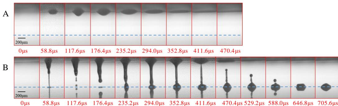
Fig. 7. Liquid transfer with different thickness liquid layer and pulse laser energy. (A) Jet flow of 150 $\mu\text{m}$  thick liquid layer with 40 $\mu\text{J}$  pulse laser energy. (B) Jet flow of 100 $\mu\text{m}$  thick liquid layer with 40 $\mu\text{J}$  pulse laser energy.
