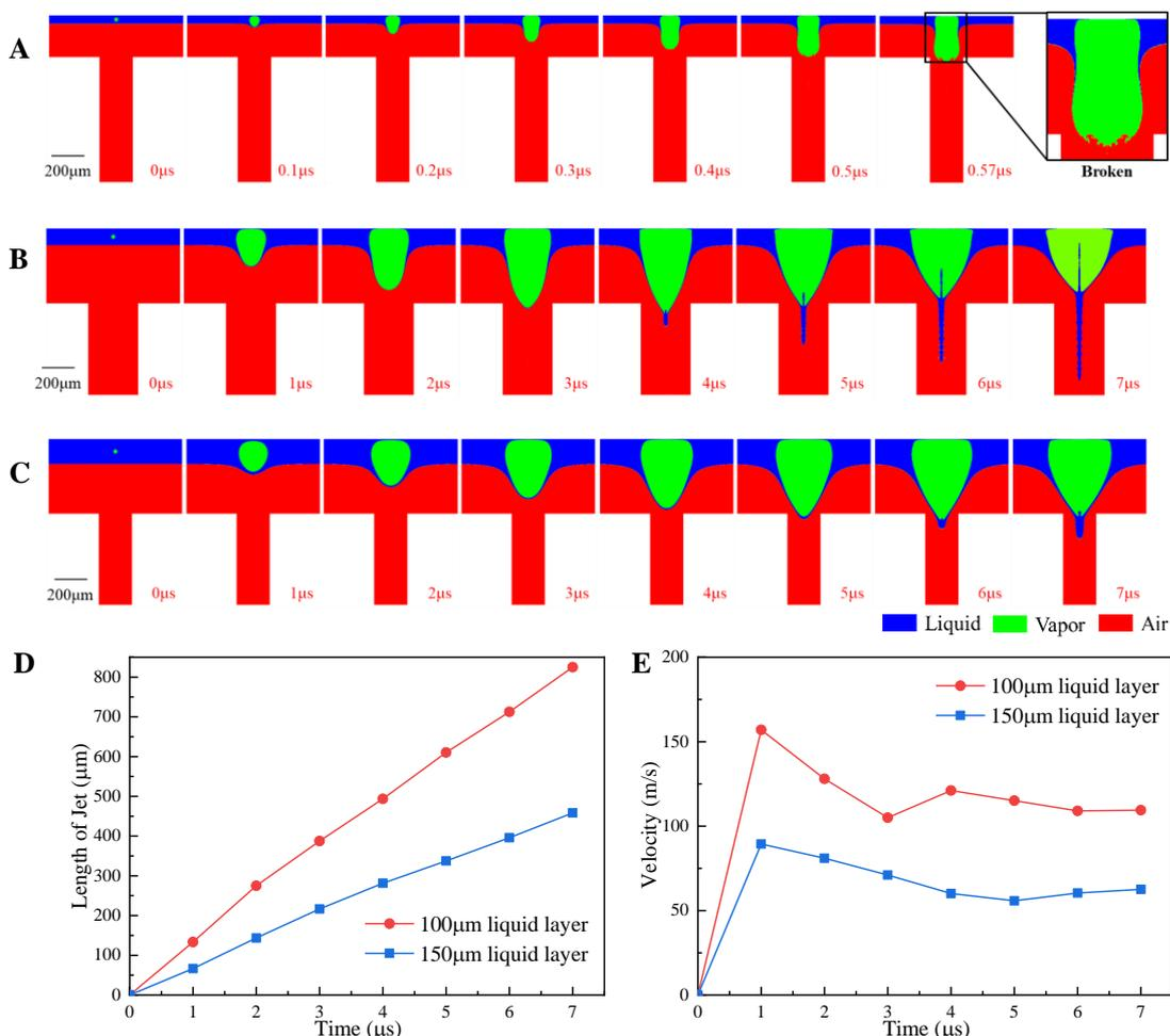
Fig. 5. Simulation of jet flow. (A) Jet flow with 50 $\mu$ m thick liquid layer and 40 $\mu$ J pulse laser energy. (B) Jet flow with 100 $\mu$ m thick liquid layer and 40 $\mu$ J pulse laser energy. (C) Jet flow with 150 $\mu$ m thick liquid layer and 40 $\mu$ J pulse laser energy. (D) The length of jet flow with different liquid layer thickness. (E) The maximum velocity of jet flow with different liquid layer thickness.
