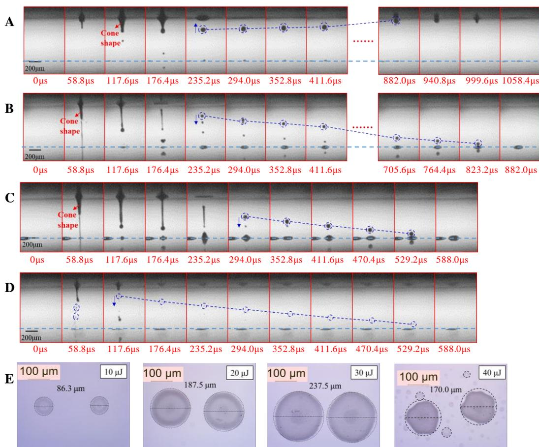
**Fig. 3.** Liquid transfer and printing patterns with 50 $\mu$ m thick liquid layer. (A) Jet flow with 10 $\mu$ J pulse laser energy. (B) Jetflow with 20 $\mu$ J pulse laser energy. (C) Jetflow with 30 $\mu$ J pulse laser energy. (D) Jetflow with 40 $\mu$ J pulse laser energy. (E) Printing patterns of 50 $\mu$ m thickness liquid layer with different pulse laser energies.
