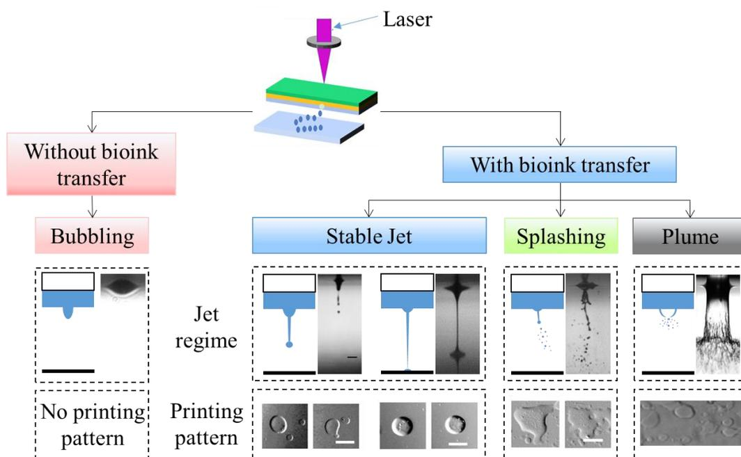
Fig. 1. Different Jet regime and corresponding printed pattern (17, 19, 22, 27)
