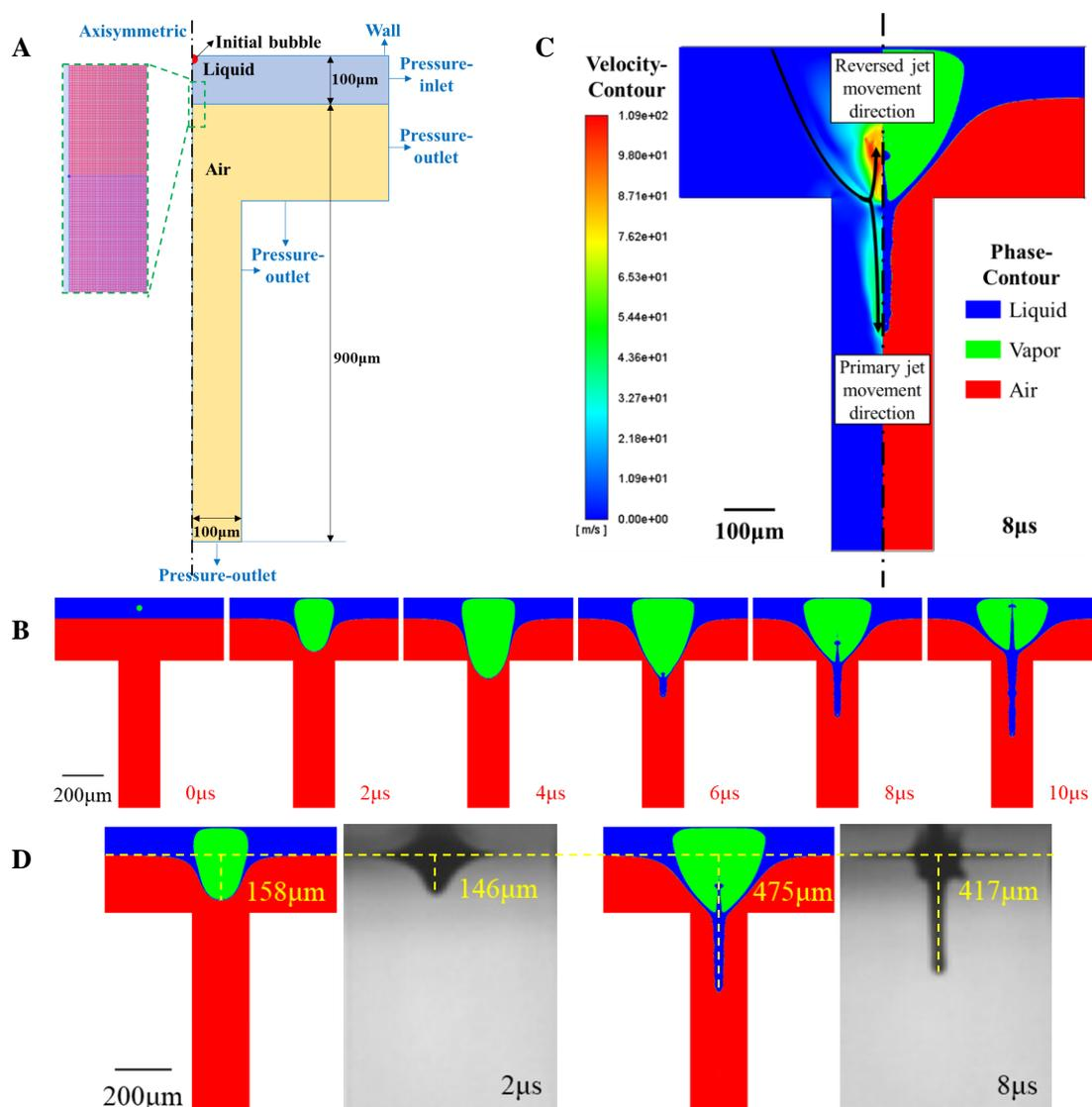
Fig. 4. Simulation of jet flow. (A) Simulation model geometry and meshing configuration. (B) Jet flow with 100 $\mu\text{m}$  thickness 65% glycerol layer and 717  $\text{mJ}/\text{cm}^2$  laser fluence. (C) Velocity of jet flow at 8 $\mu\text{s}$ . (D) Comparison with experimental results (17).
