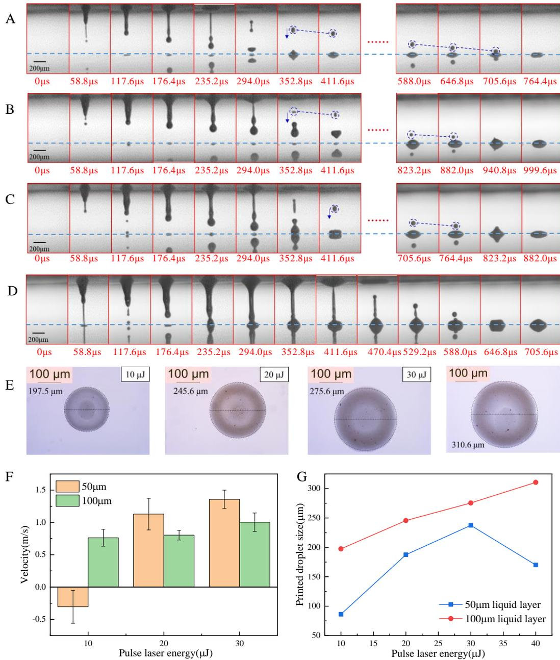
*Fig. 8. Liquid transfer and printing patterns with 100 μm thick liquid layer. (A) Jet flow with 10 μJ pulse laser energy. (B) Jetflow with 20 μJ pulse laser energy. (C) Jetflow with 30 μJ pulse laser energy. (D) Jet flow with 40 μJ pulse laser energy. (E) Printing patterns with different pulse laser energies. (F) The movement velocity of the dropped droplet. (G) Printed droplet size of different liquid layer thickness with different pulse laser energy.*
