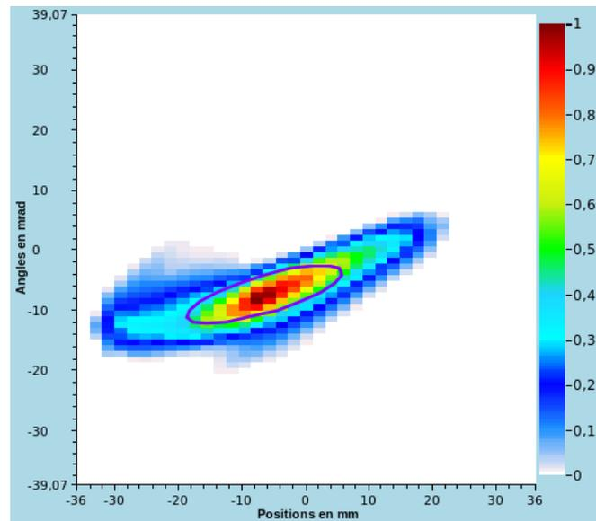
**Figure 5.** Example of emittance-meter measurement in x of a beam of  $O^{6+}$  at the SPIRAL2 LBE beamline. The non-normalized emittance measured is  $39.15 \pi \cdot \text{mm} \cdot \text{mrad}$  (60 keV beam kinetic energy).
