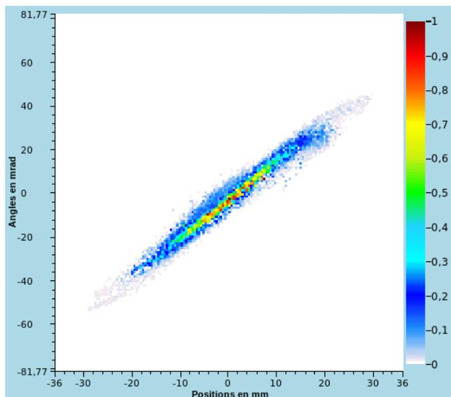
**Figure 6.** Example of emittance-meter measurement in y of a beam of  $H^+$  at the SPIRAL2 LBE beamline. The non-normalized emittance measured is  $27.77 \pi \cdot \text{mm} \cdot \text{mrad}$  (20 keV beam kinetic energy).
