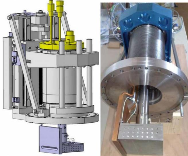
**Figure 2.** Technical drawing and picture of the IPHC emittance-meter.
