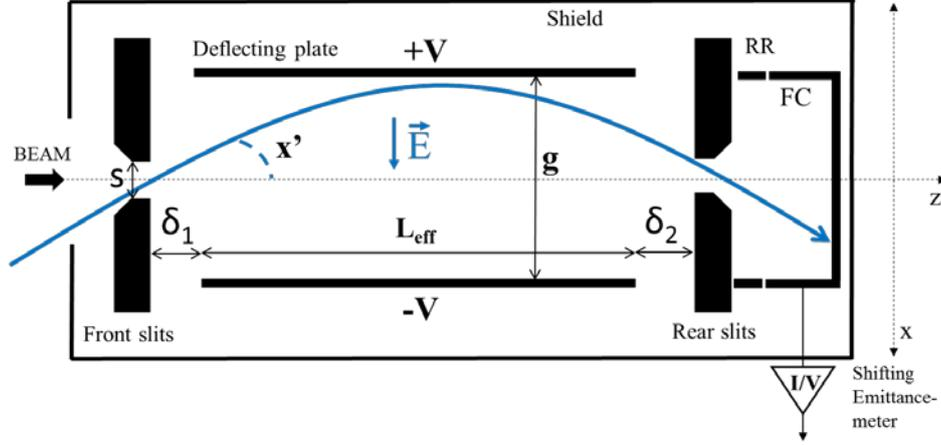
**Figure 1.** Schematic of the Allison principle. +V and -V are the potential of the plates. S is the aperture of the front slit.  $L_{eff}$  is the effective length of the plates.  $\delta_1$  and  $\delta_2$  are the distances between the plates and the front and rear slits respectively. FC means Faraday Cup.  $g$  is the gap between the plates.  $E$  is the electrical vector induced by the voltage between the plates. RR is the electron repelling ring.
