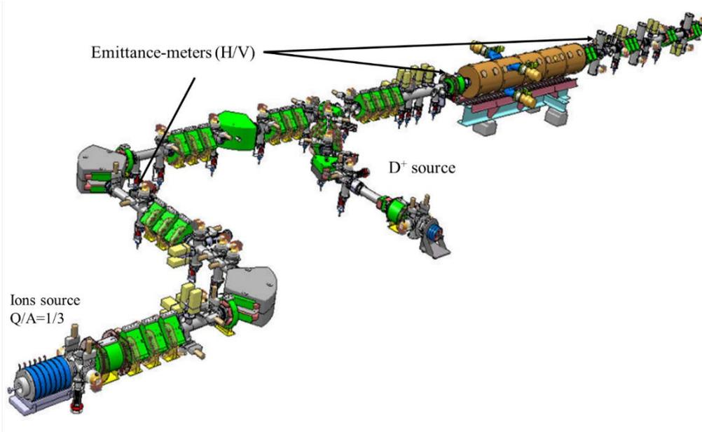
**Figure 4.** Location of the three pairs of IPHC emittance-meters on the LEBT and MEBT sections of SPIRAL2.
