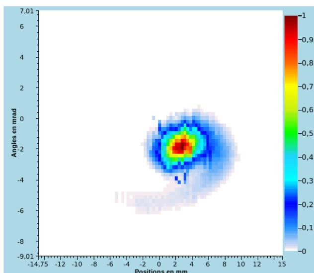
**Figure 7.** Example of emittance-meter measurement in y of a beam of  $H^+$  at the SPIRAL2 LME beamline. The non-normalized emittance measured is  $1.92 \pi \cdot \text{mm} \cdot \text{mrad}$  (730 keV beam kinetic energy).
