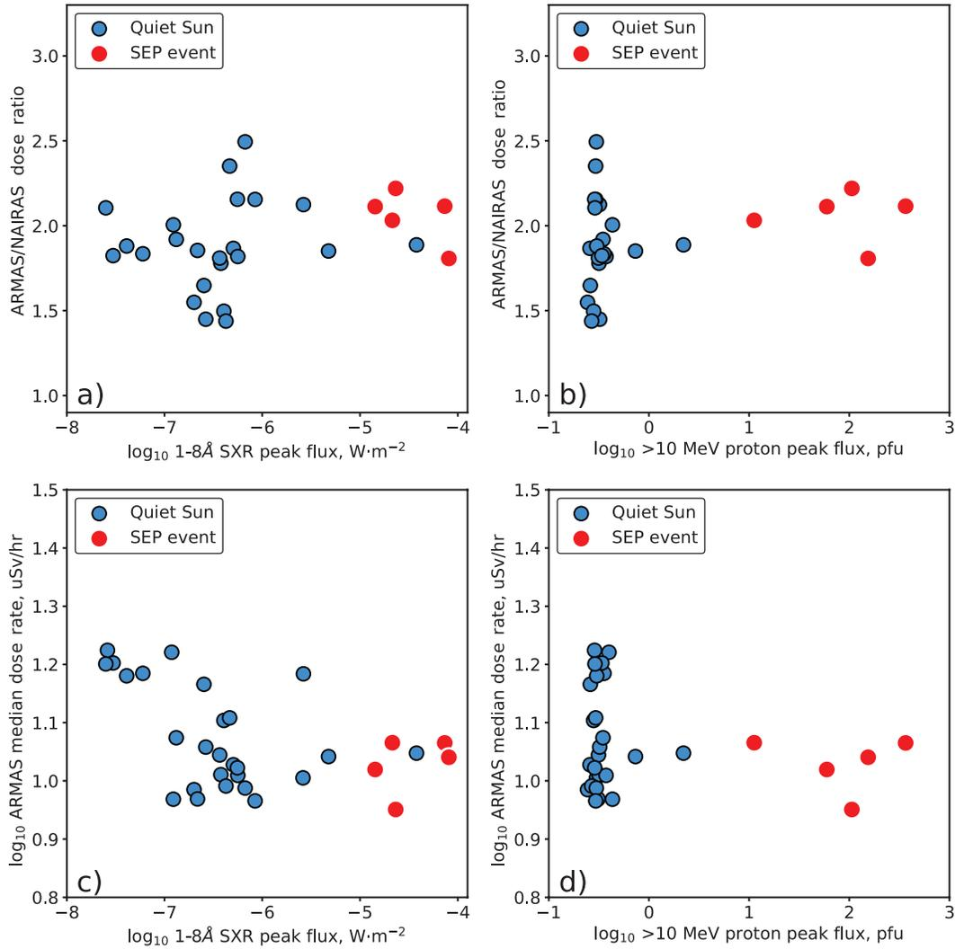
**Figure 3.** Correlations between the total dose ratios of ARMAS to NAIRAS v1 to X-ray flux (panel a) and proton flux above 10 MeV (b). Dependence of the ARMAS median effective dose rate from X-ray flux (panel c) and proton flux above 10 MeV (d). Red circles correspond to flights when the peak value of > 10 MeV proton flux exceeded 10 pfu, and blue circles indicate the flights when the > 10 MeV proton flux was less than 10 pfu.
