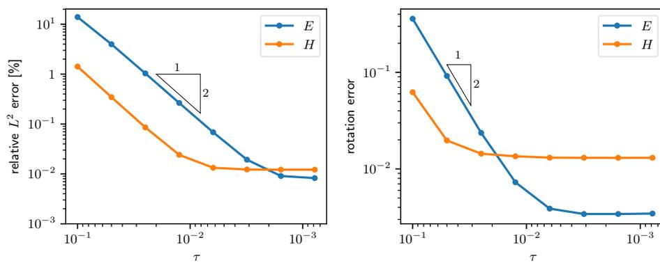
Figure 2: Order of the time integration scheme as measured in L2 (left) and H-curl (right) norms for electric (blue) and magnetic (orange) vector fields resulting from the solution of the problem with manufactured solution over the computational mesh with  $16 \times 16 \times 16$  elements.
