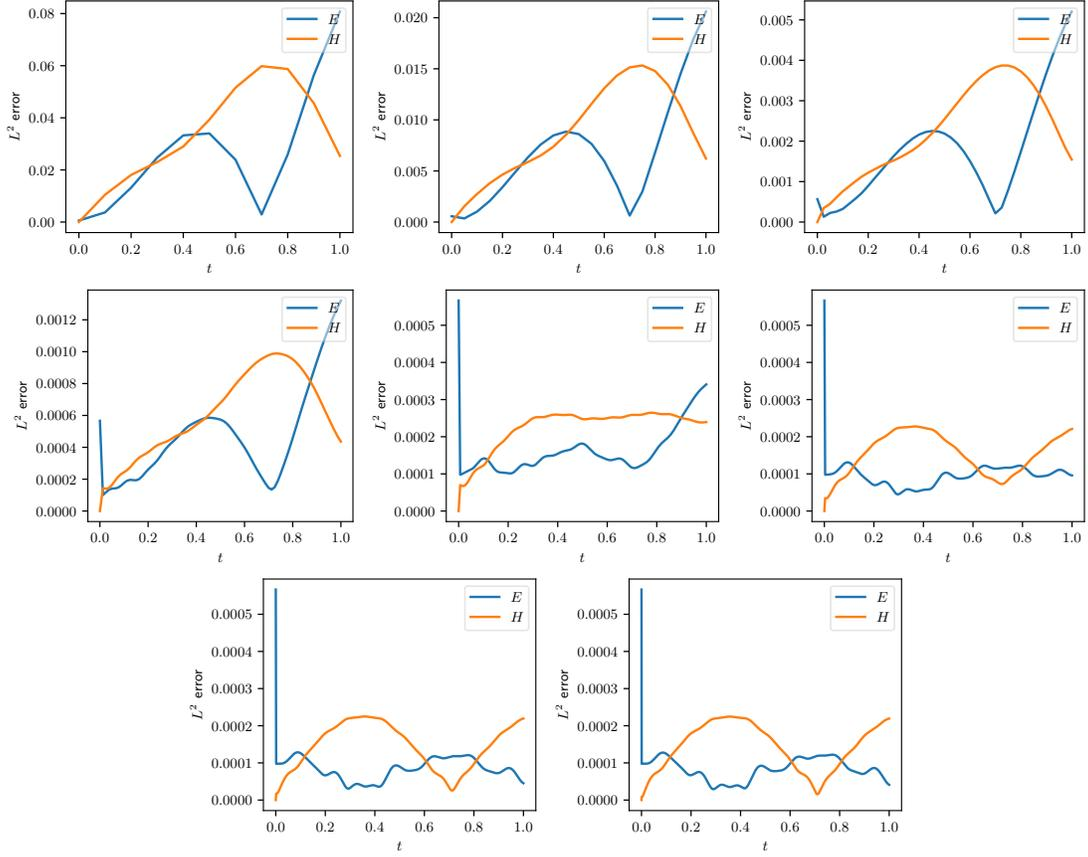
Figure 3: L2 norm error of electric (blue) and magnetic (orange) vector fields resulting from the solution of the problem with manufactured solution over the computational mesh with  $16 \times 16 \times 16$  elements, for the time interval  $[0,1]$ , with number of time steps within  $[0,1]$  interval varying from 10,20 (first row), 40,80 (second row), 160,320 (third row), 640 and 1280 (last row).
