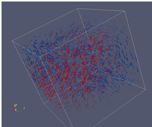
Figure 1: Electric (red) and magnetic (blue) vector fields, resulting from the problem with manufactured solution.
