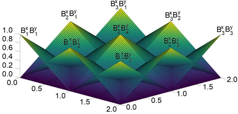
Figure 10: Simple mesh with linear B-splines defined by tensor product of two knot vectors  $[0 \ 0 \ 1 \ 2 \ 2] \times [0 \ 0 \ 1 \ 2 \ 2]$ .
