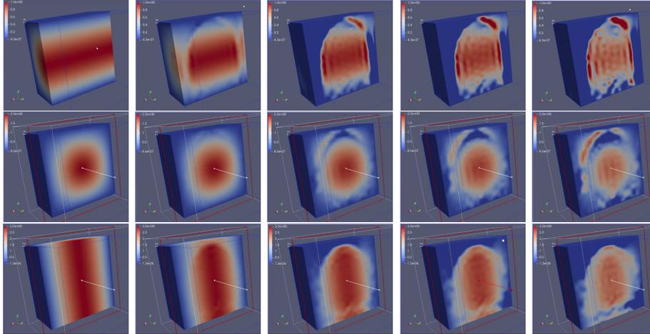
Figure 6: Electromagnetic waves propagation on the human head. First row:  $x$  component of the electric vector field. Second row:  $y$  component of the electric vector field. Third row:  $z$  component of the electric vector field. Columns - cross section along OYZ plane, time moments: 0, 0.25, 0.5, 0.75, 1.0s. Mesh size  $32 \times 32 \times 32$ , quadratic  $C^1$  B-splines.
