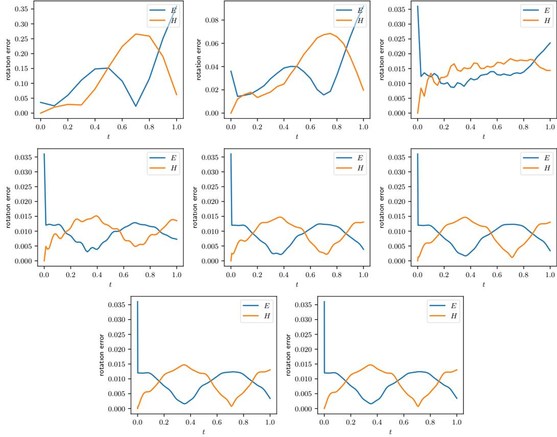
Figure 4: H-curl norm error of electric (blue) and magnetic (orange) vector fields resulting from the solution of the problem with manufactured solution over the computational mesh with  $16 \times 16 \times 16$  elements, for the time interval  $[0,1]$ , with number of time step varying from 10,20 (first row), 40,80 (second row), 160,320 (third row), 640 and 1280 (last row).
