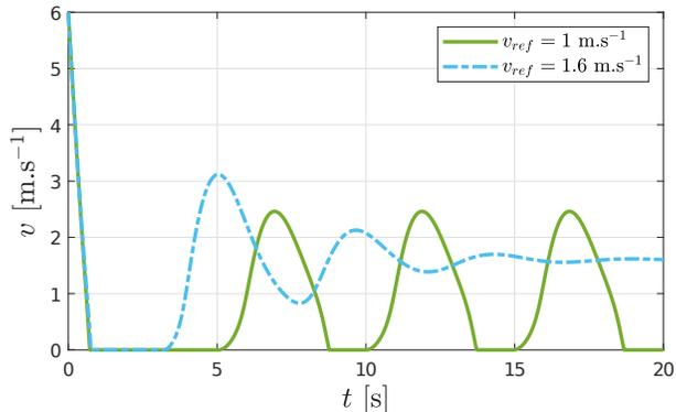
Figure 5: Numerical simulation of (4) for  $v_{ref} \in \{1, 1.6\}$  m.s<sup>-1</sup>,  $v_0 = 6$  m.s<sup>-1</sup> and  $z_0 = 0$  m.
