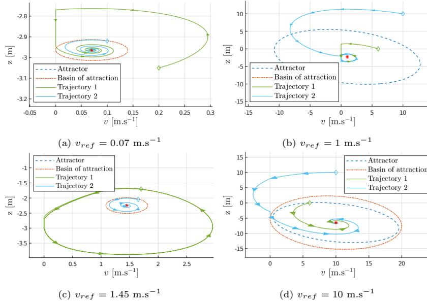
Figure 6: Phase portraits of (4) for four values of  $v_{ref}$ . The inner-approximation of  $\mathcal{A}_{v_{ref}}$  is in dash-blue and the outer estimation of  $\mathcal{D}_{v_{ref}}$  is in dash-dot-red. The equilibrium point is the red star and the two trajectories initiate from the diamond points.
