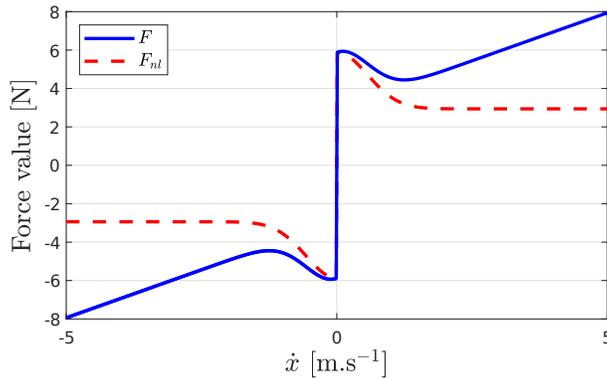
Figure 2: Chart of the friction force (in solid blue) and static and Coulomb forces (in dashed red) in our problem. Note that the friction force is not a monotonous function of the speed, inducing the famous stick-slip effect.
