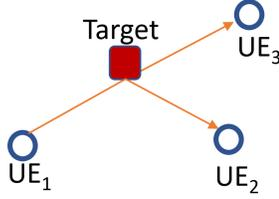
Fig. 1: The co-linear node pair (UE<sub>1</sub>-UE<sub>3</sub>) is more sensitive to measurement errors than (UE<sub>1</sub>-UE<sub>2</sub>), due to a greater geometric dilution of precision (GDOP).
