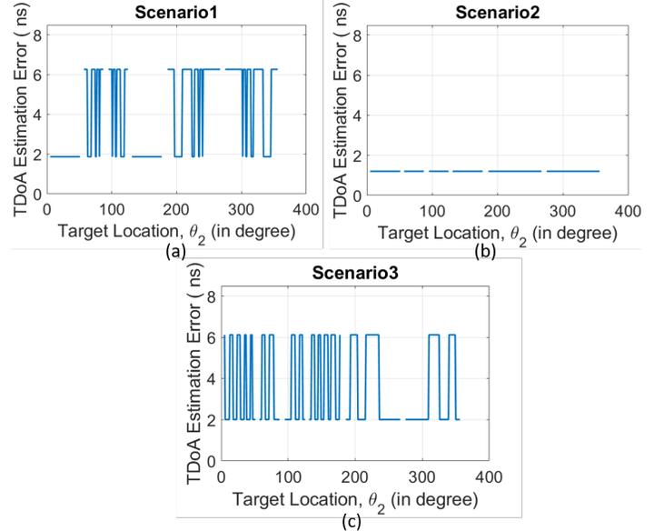
Fig. 4: The TDOA estimation error for target localization along the iso-range contour with signal BW = 100 MHz.
