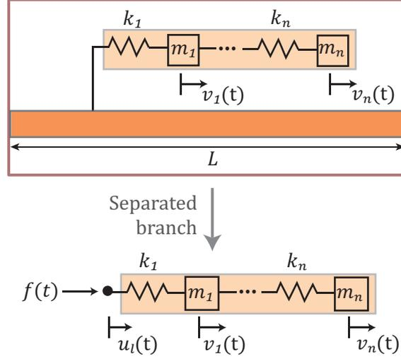
Fig. 5: **(Top)** A branched metamaterial unit cell with a continuum base modeled as a 1D rod connected to an  $n$ -degrees-of-freedom resonating branch, which is inspected separately **(bottom)** with a point force applied at the previous connection node to the base.
