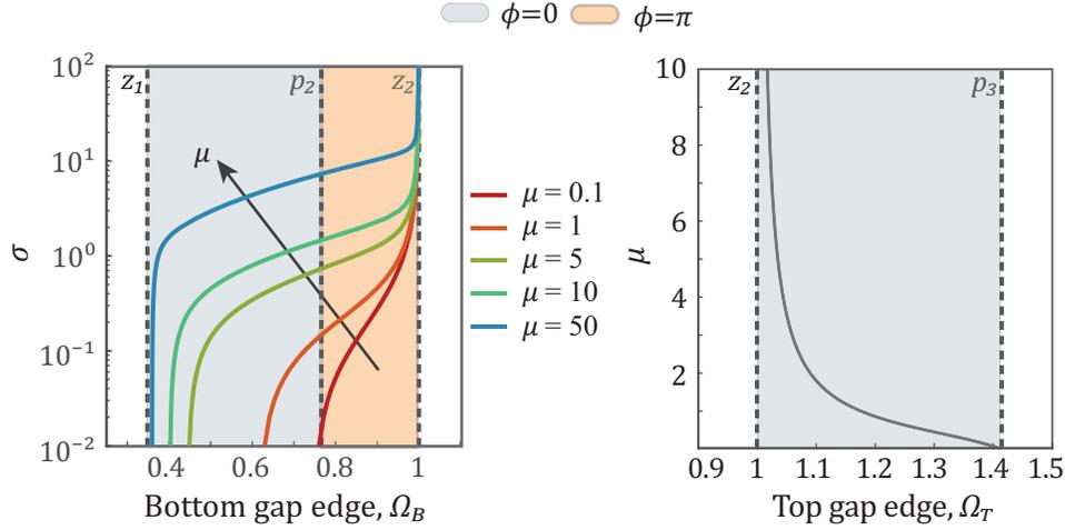
Fig. 3: Variation of the bottom band-gap edge  $\Omega_B$  (left) and top band-gap edge  $\Omega_T$  (right) with mass and stiffness ratios  $\mu$  and  $\sigma$ , as computed in a numerical parametric study for the second LR band gap. In all cases, a 4-DOF resonating branch with mass ratios  $m_{f,j} = 1$  and stiffness ratios  $k_{f,j} = 1$ , with  $j = 1, \dots, 4$ , is connected to the base chain.
