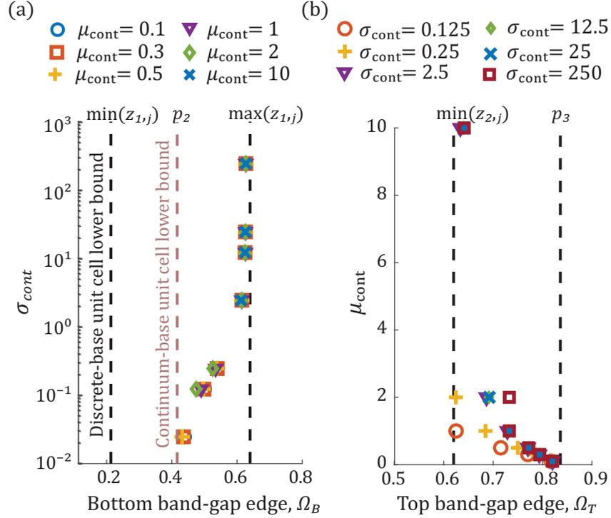
Fig. 9: (a) FEM-calculated second band-gap bottom edges plotted against the modulus ratio  $\sigma_{\text{cont}}$  for different density ratios  $\mu_{\text{cont}}$ . (b) FEM-calculated second band-gap top edges plotted against density ratio  $\mu_{\text{cont}}$  for different modulus ratios  $\sigma_{\text{cont}}$ . In all cases, the branch Young's modulus  $E_{\text{branch}} = 4\text{GPa}$ , density  $\rho_{\text{branch}} = 1000\text{kg/m}^3$  and Poisson ratio  $\nu = 0.34$ .
