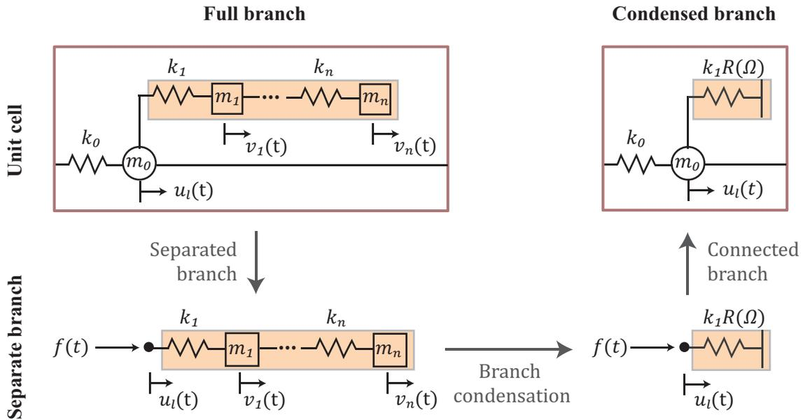
Fig. 1: **(Top left)** A branched metamaterial unit cell with a base mass  $m_0$  connected to an  $n$ -degrees-of-freedom resonating branch, which is inspected separately below **(bottom left)** with a point force applied at the previous connection node to the base. **(Bottom right)** The branch is condensed into an effective stiffness  $R(\Omega)$  experienced by the point force and is replaced into the unit cell **(top right)**.
