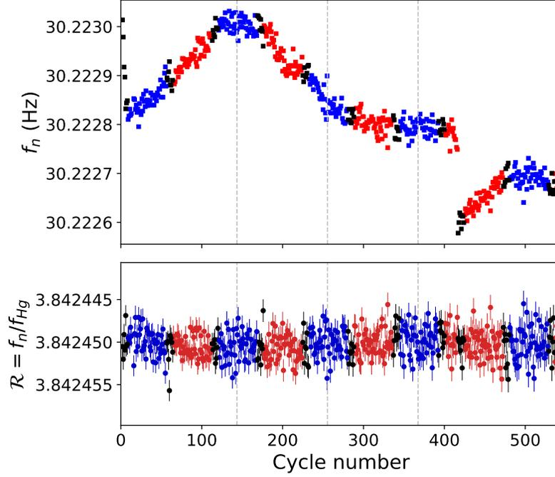
Figure 27.4: Plot of neutron frequency (top),  $f_n$ , and frequency ratio (bottom),  $\mathcal{R}$ , for a full sequence of nEDM data. Red data points indicate a positive voltage, while negative are marked blue. Black is used for cycles without electric field. A single EDM value is extracted for each sub-sequence, indicated by vertical dashed lines, before a weighted EDM average is calculated for the entire sequence. Figure reused from [12].
