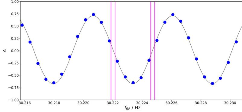
Figure 27.2: Measurement of the asymmetry  $A = (N_{\uparrow} - N_{\downarrow}) / (N_{\uparrow} + N_{\downarrow})$  as a function of the applied frequency  $f_{\text{RF}}$  of the pulses. Each point is a measurement cycle with a precession time of  $T = 180$  s performed with the single chamber apparatus in 2017. The vertical bars show the position of the four “working points” used in the nEDM data-taking to maximize the sensitivity. The line is a fit of (27.3) to the data.
