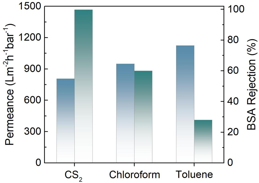
**Figure S7.** Separation performances of the PS-*b*-P2VP-*m*UPCFs/AAO composite membranes prepared with different solvent.
