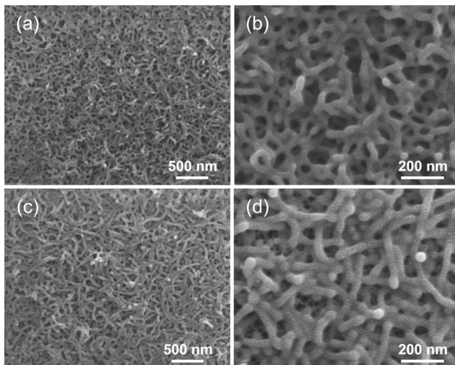
**Figure S5.** Surface SEM images of the PS-*b*-P2VP-*m*UPCFs/AAO composite membranes prepared with a concentration of 0.05 wt%. (a) 65°C for 1 h. (b) 75°C for 1 h.
