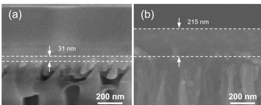
**Figure S4.** Cross-sectional SEM images of the PS-*b*-P2VP-UPCFs/AAO composite membranes. (a) 0.03 wt%. (b) 0.1 wt%.
