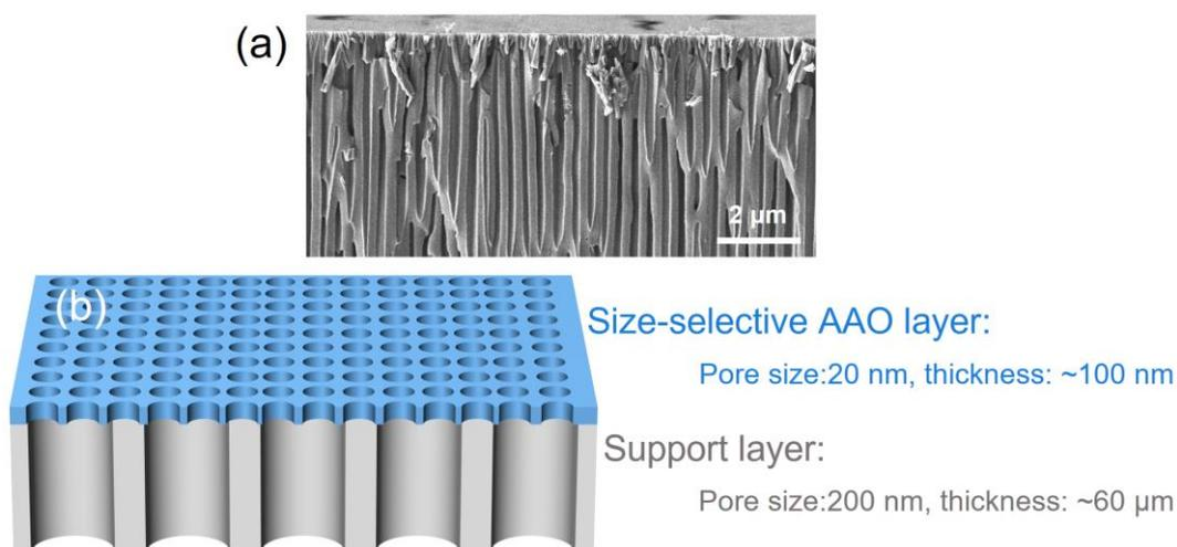
**Figure S1.** Cross-sectional SEM image (a) and illustration (b) of an as-received AAO membrane showing the thin size-selective AAO layer (pore diameter ~20 nm) at the top and the underlying AAO membrane with pore diameters scattering about 200 nm.
