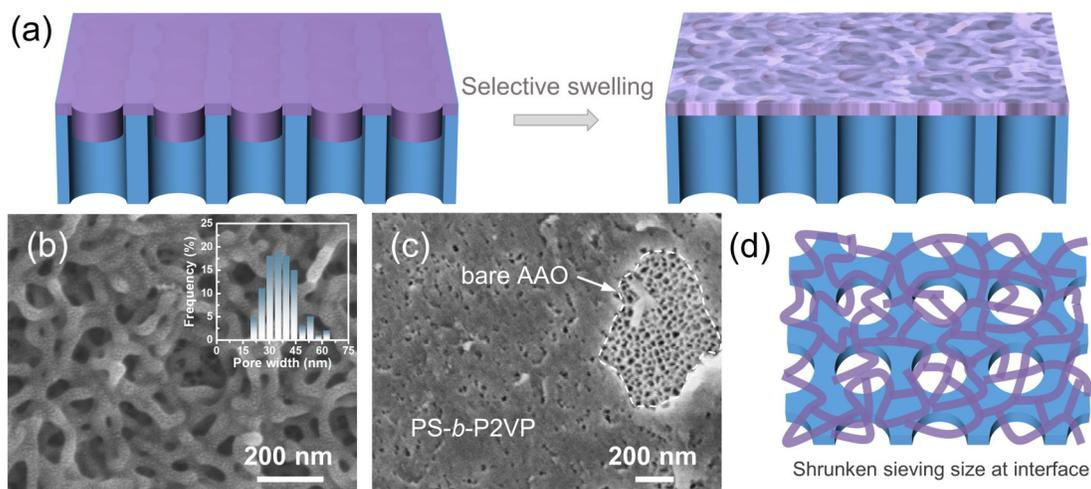
**Figure 2.** Selective swelling of PS-*b*-P2VP-UPCF/AAO composite membranes. (a) Schematic diagram of the selective swelling. Surface SEM images of the pristine (b) and polished (c) PS-*b*-P2VP-*m*UPCF/AAO membranes. The membrane was prepared with a 0.05 wt% precursor solution followed by swelling in 70°C ethanol for 1 h, and the inset in (b) shows the pore size distribution. (d) Illustration of the shrunken sieving sizes induced by stagger stacking.
