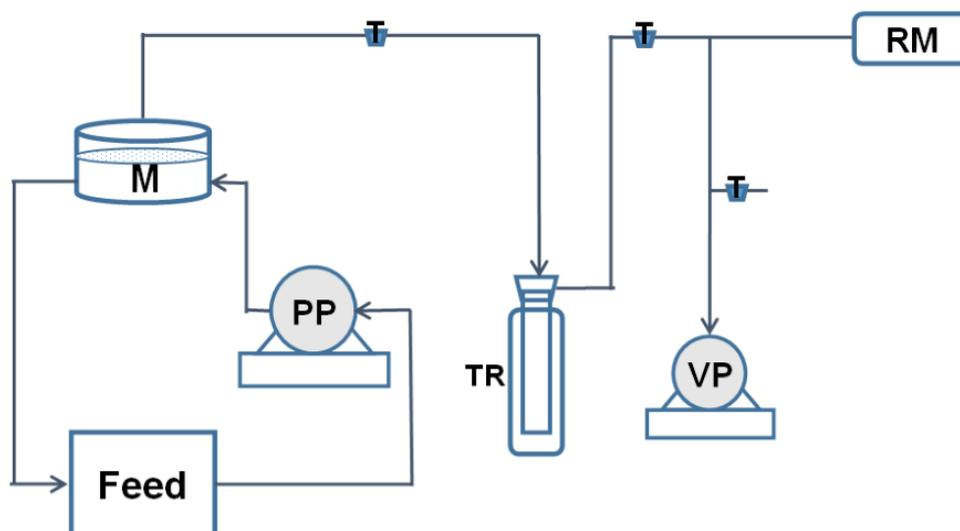
M: Membrane Module; PP: Peristaltic Pump; TR: Cold Trap;
