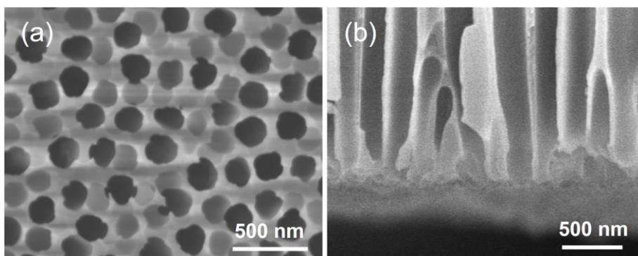
**Figure S3.** SEM images of the PS-*b*-P2VP-UPCFs/AAO composite membrane prepared with a concentration of 0.05 wt%. (a) Bottom surface. (b) Bottom cross section.
