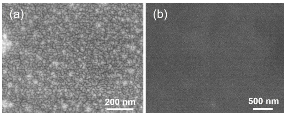
**Figure S2.** Surface SEM images of the PS-*b*-P2VP-UPCFs/AAO composite membranes. (a) 0.03 wt%. (b) 0.1 wt%.
