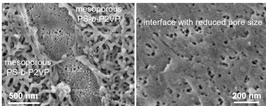
**Figure S6.** Surface SEM images of the PS-*b*-P2VP-*m*UPCFs/AAO composite membrane after removing the top mesoporous PS-*b*-P2VP layer. The membrane was prepared with concentration of 0.05 wt% followed by swelling at 70°C for 1 h.
