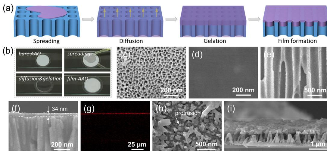
**Figure 1.** Fabrication of PS-*b*-P2VP UPCFs. (a) Schematic diagram for the film preparation. (b) Digital images during the film preparation. Surface SEM images of the bare AAO substrate (c) and UPCF (d). (e, f) Cross-sectional SEM images of the UPCF. (g) Cross-sectional fluorescent image. Bottom (h) and cross-sectional SEM images of the UPCF after removing AAO substrates. The UPCF was prepared by coating a 0.05 wt% PS-*b*-P2VP/CS<sub>2</sub> solution.
