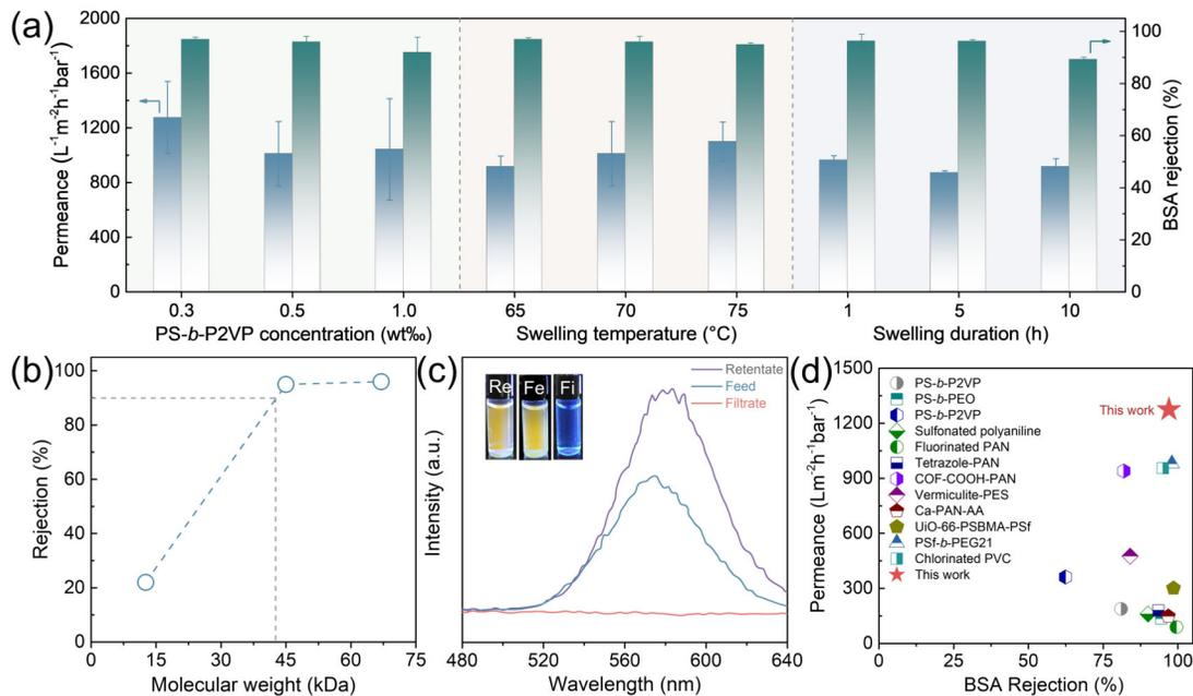
**Figure 3.** Separation performance of PS-*b*-P2VP-*m*UPCF/AAO composite membranes. (a) Performances with various PS-*b*-P2VP concentrations, swelling temperatures, and durations. (b) Rejections to various objects with different molecular weight. (c) Emission spectra of the feed, filtrate and retentate obtained by concentrating CdTe QDs. (d) Comparison on the separation performance of various membranes. Inset in (c) shows fluorescent photographs of the feed (Fe),
