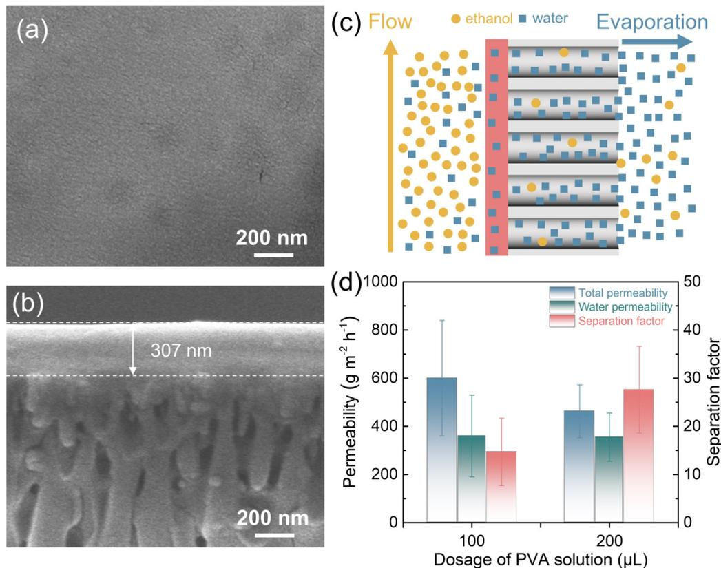
**Figure 4.** Cross-linked PVA-UPCF/AAO composite membranes for the dehydration of ethanol by pervaporation. Surface (a) and cross-sectional (b) SEM images of the membrane prepared with 100  $\mu\text{L}$  PVA solution. (c) Schematic diagram for the pervaporation. (d) Permeabilities and separation factors of membranes prepared with various dosages of PVA solution.
