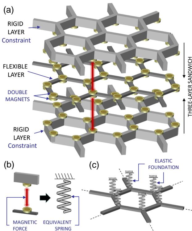
FIG. 1. Magneto-mechanical multi-layer analog of graphene bilayer. (a) Three-layer sandwich stacking. (b) Equivalent spring models for the magnetic interactions (c) Inner layer modeled as single layer on elastic foundation.
