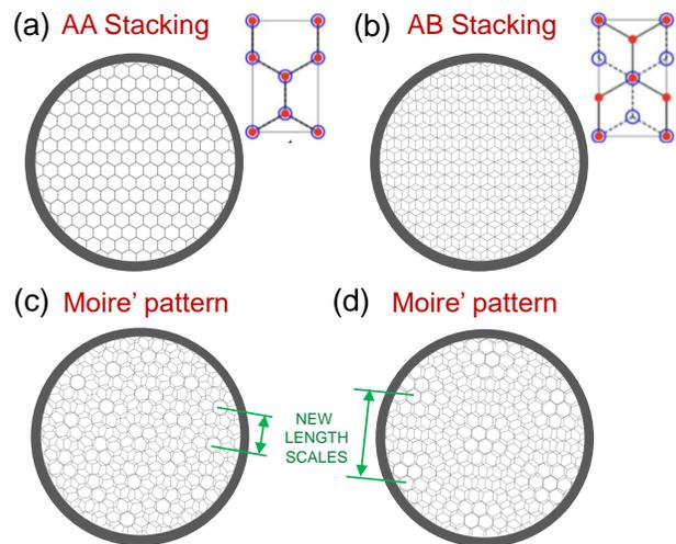
FIG. 2. Schematic illustration of the opportunities for reconfiguration available via twisting. (a) AA stacking for twist angle  $\theta = 0^\circ$  and perfectly overlapping layers (two lattice sites overlapping per unit cell). (b) AB stacking for  $\theta = 60^\circ$  with one lattice site overlapping per unit cell. (c-d) Examples of Moiré patterns obtained with intermediate twist angles.
