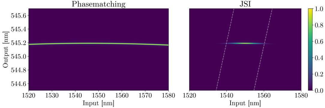
Figure 1: Phase-matching function and JSI of a QPG at 200 °C. The pump field used to obtain the JSI is a gaussian pulse centered around 841 nm with 2.12 nm  $\sigma$  bandwidth, in dashed lines on the plot.
