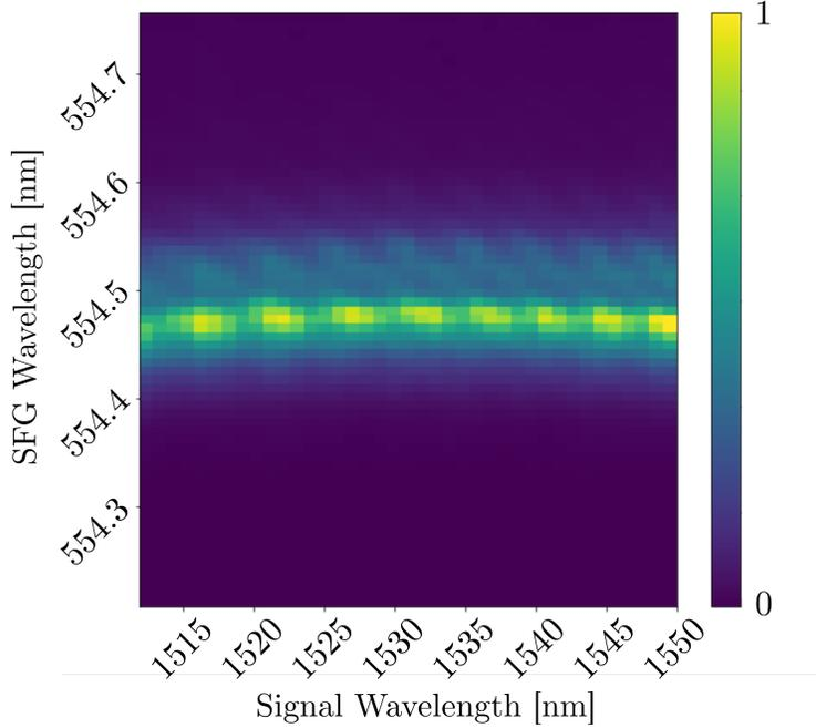
Figure 6: 2D phase-matching of the QPG process measured at 200 °C. The intensity beating seen is an artifact of the experimental measurement.
