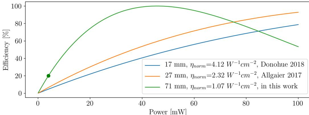
Figure 7: Comparison between the conversion efficiencies calculated from the  $\eta_{norm}$  in [13, 14] and in this paper with equation 3. The green dot marks the value measured experimentally.
