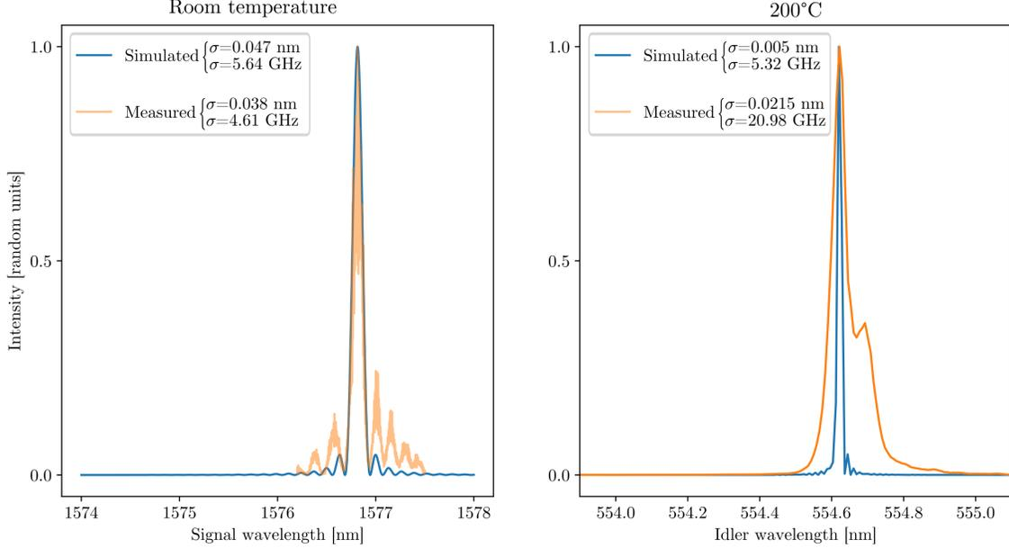
Figure 5: Simulated and measured phase-matchings of the sample at room temperature ( $\approx 21^\circ\text{C}$ ) and at  $200^\circ\text{C}$ . At  $200^\circ\text{C}$  the simulation was performed with the spectrometer’s resolution. The  $1/e$  bandwidth ( $\sigma$ ) of each spectra is annotated in the legend in wavelength and frequency units.
