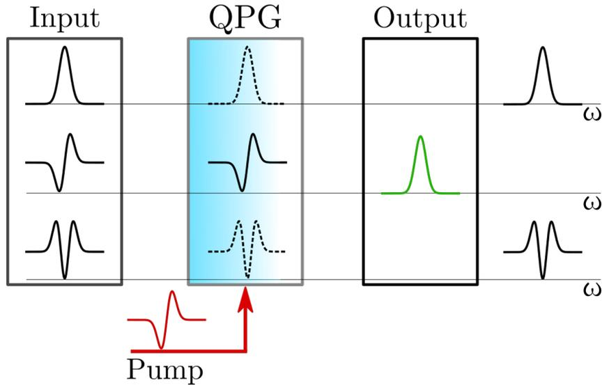
Figure 2: The QPG performs SFG on the input modes that overlap with the pump modes, the remaining modes propagate unperturbed.
