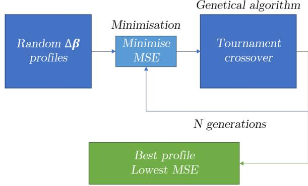
Figure 8: Flowchart of the optimisation algorithm.
