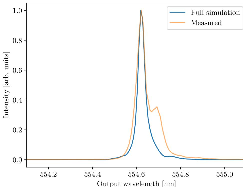
Figure 10: The simulated phase-matching function fits the main feature of the measured one.
