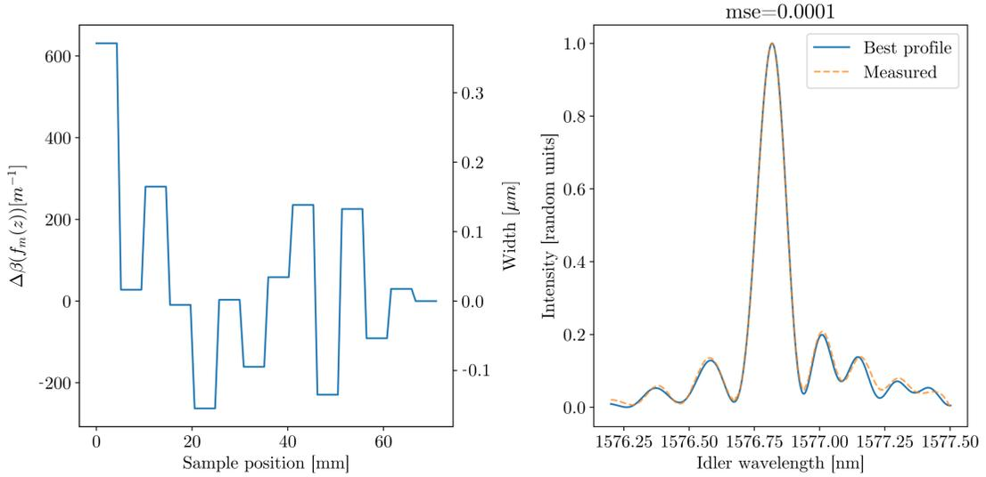
Figure 9: The resulting  $\Delta\beta(f_m(z))$  profile after running the genetic algorithm is on the left. The y axis on the right are the equivalent waveguide width deviation for the profile. The best profile's phase-matching function is plotted against the measured one at room temperature on the right. The MSE is 0.0001.
