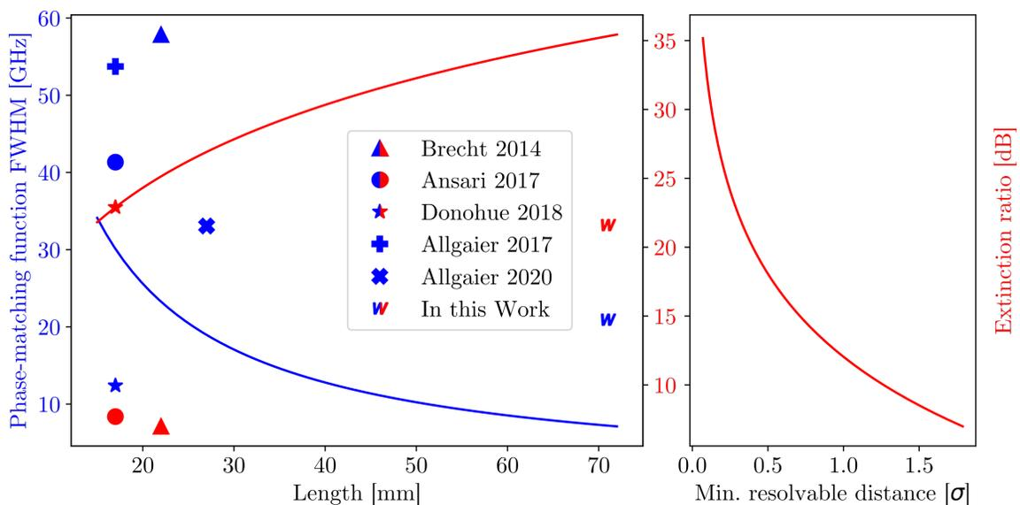
Figure 3: a) Expected phase-matching function full width at half maximum (FWHM) (blue) and extinction ratio (red) for the length of the device. The reviewed articles and the results presented in this paper are shown for comparison. b) Minimum resolvable distance in terms of the  $1/e$  bandwidths ( $\sigma$ ) of two close signals expected for the extinction ratio.
