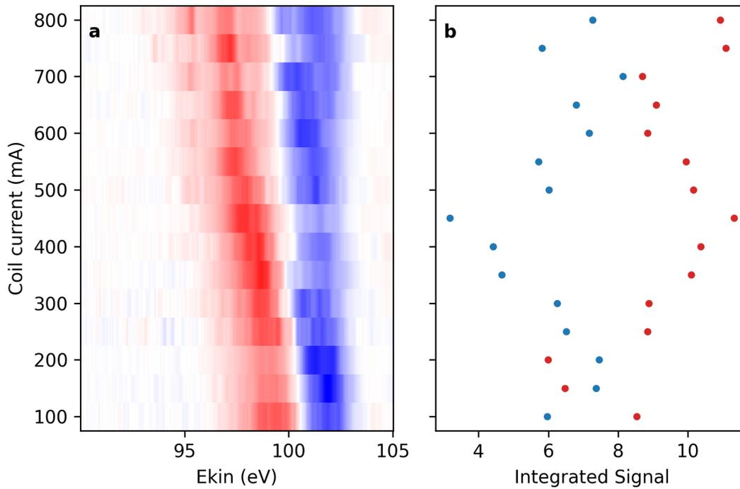
Figure S2: Scan of the coil current on the flight tube at 272 eV x-ray photon energy and -80 V retardation. a: false-color representation of the difference spectra of the photoline. b: integrated signal of positive (red) and negative (blue) contributions.
