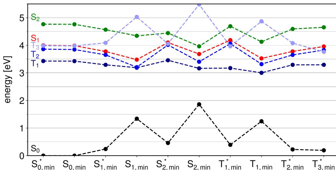
Figure S8: EOM-CCSD/6-311++G\*\* electronic energies of the lowest singlet and triplet states of 2-thiouracil, calculated at the planar and non-planar minima of the different states.
