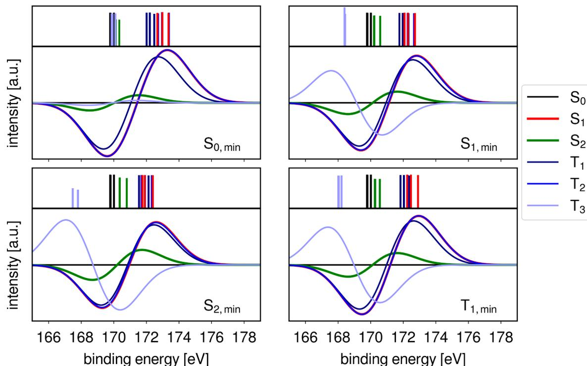
Figure S10: Binding energies of the 2p electrons (top panels) and pump-probe spectra (bottom panels) evaluated for different electronic states and different fully optimized geometries. The ionization intensities are estimated using Dyson orbital norms.
