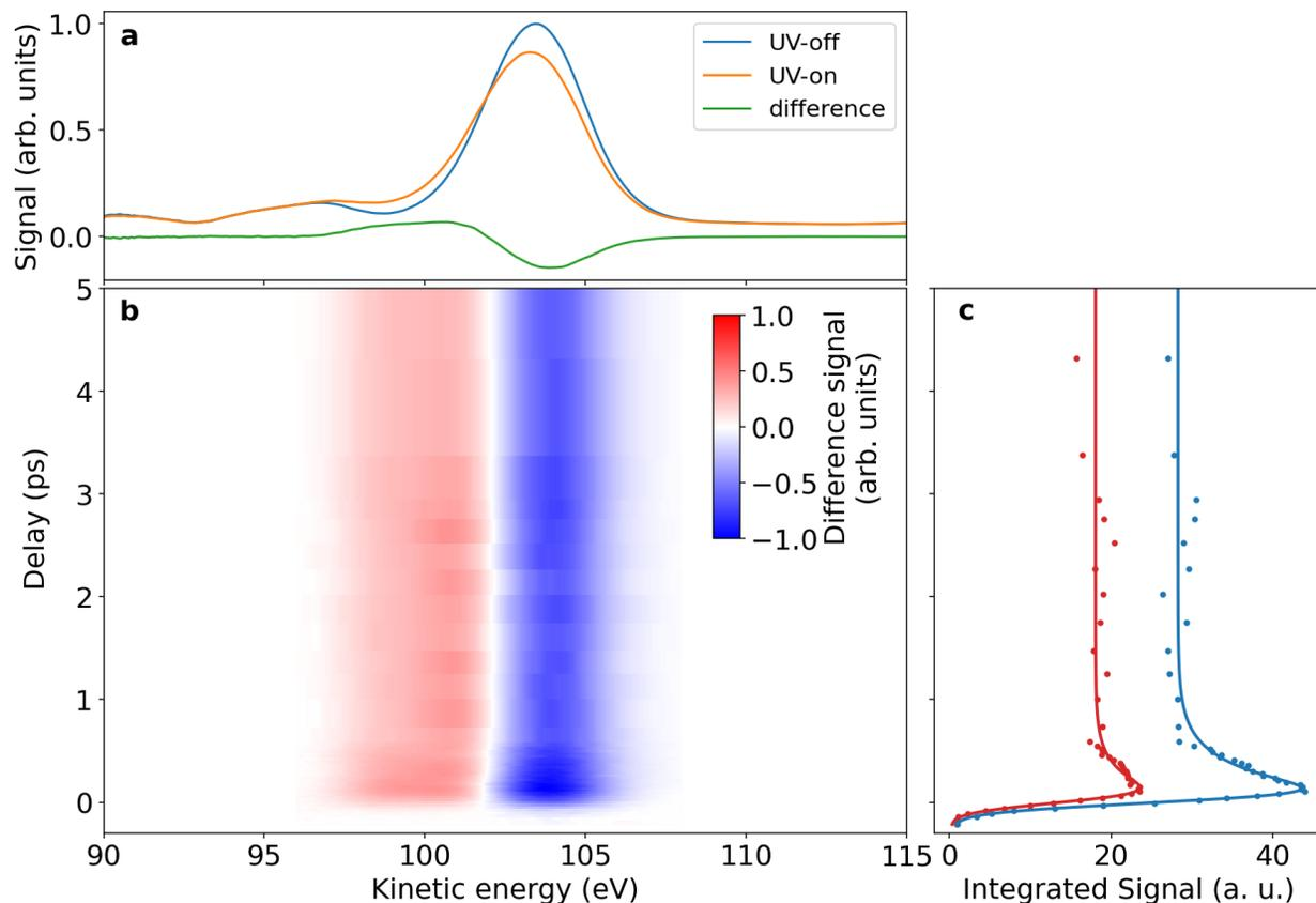
Figure 2: Experimental time-resolved XPS spectra of 2-thiouracil. (a) UV-on (orange) and UV-off (blue) photoelectron spectra as well as the difference spectrum (green) between UV-on and UV-off at a delay of 200 fs. (b) False-colour plot of time-dependent difference XPS with red indicating UV-induced increase of the photoelectron spectrum and blue a UV-induced decrease. (c) Integrated signal of the positive and negative parts of the difference spectra (dots) and fit to the data (solid line).
