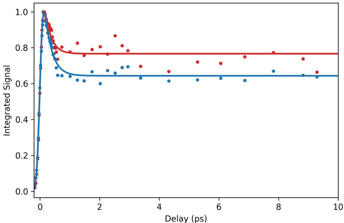
Figure S1: Integrated (absolute) signal for positive (red) and negative lobe (blue) of the S2p difference spectrum normalized on the maximum.
