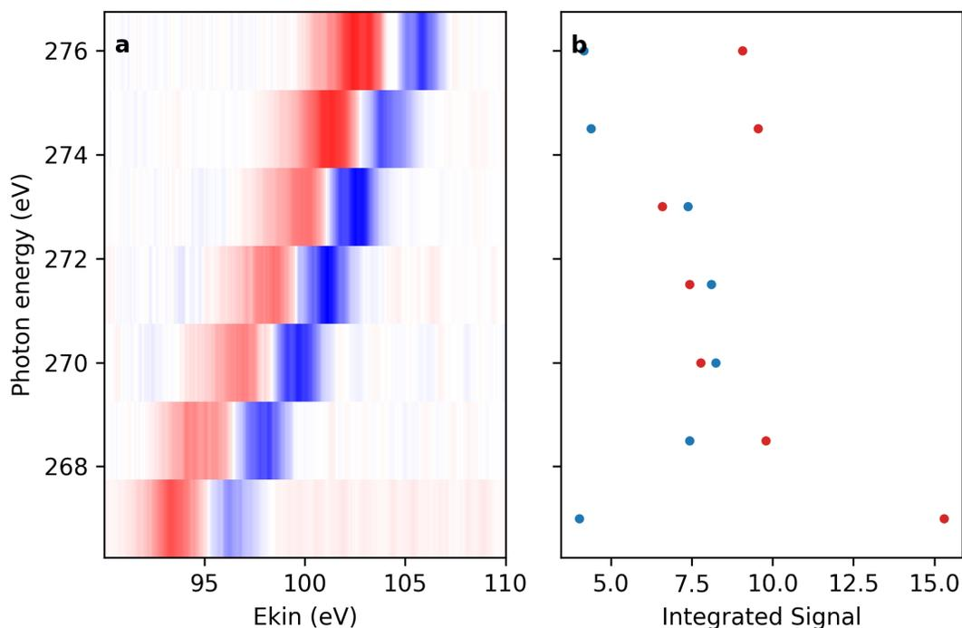
Figure S4: Scan of the photon energy at 80V retardation and 200mA coil current. a: false-color representation of the difference spectra of the photoline. b: integrated signal of positive (red) and negative (blue) contributions.
