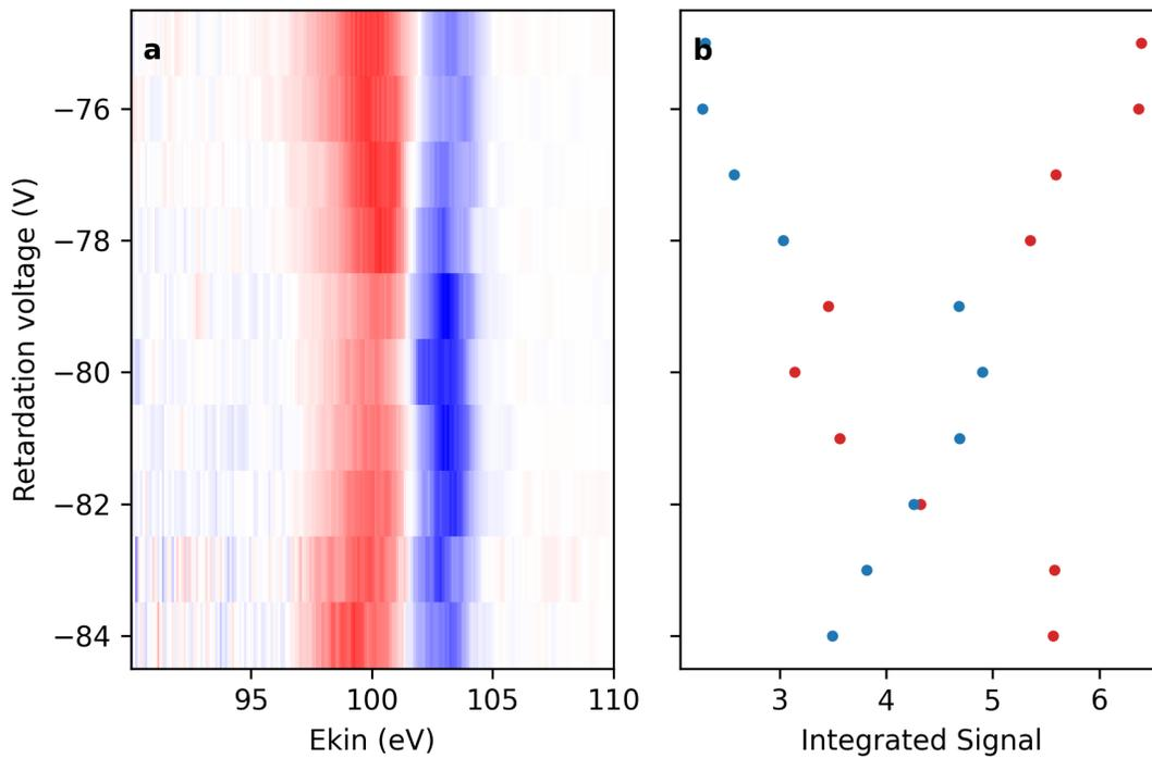
Figure S3: Scan of the retardation voltage at 272 eV and 200 mA coil current. a: false-color representation of the difference spectra of the photoline. b: integrated signal of positive (red) and negative (blue) contributions.
