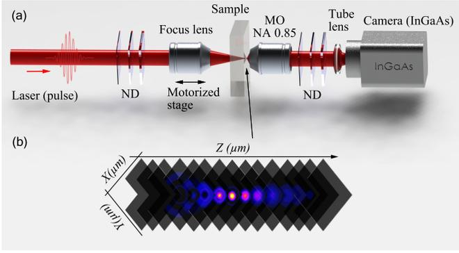
**Fig. 2.** Illustration of in-bulk propagation imaging process. (a) Experimental setup, MO: microscope objective, ND: neutral density filters. (b) Intensity distribution near the focal region reconstructed from the stack of recorded images.
