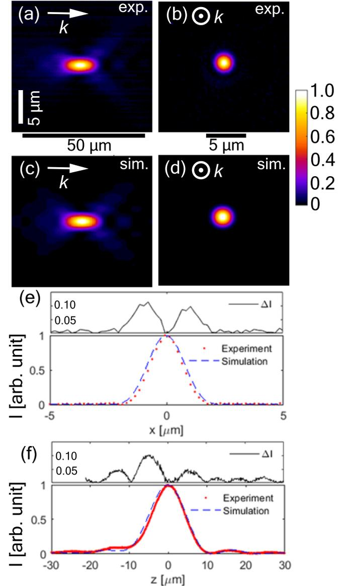
**Fig. 3.** Intensity distribution near the focus of an aspherical lens in air with a Gaussian beam as the input. (a) Experimentally measured intensity along  $xz$  plane; (b) experimentally measured intensity at the focal plane; (c) simulated intensity along  $xz$  plane; (d) simulated intensity at the focal plane. (e) Comparison of the intensity profiles at the focal plane along the  $x$ -axis, (f) along the  $z$ -axis.
