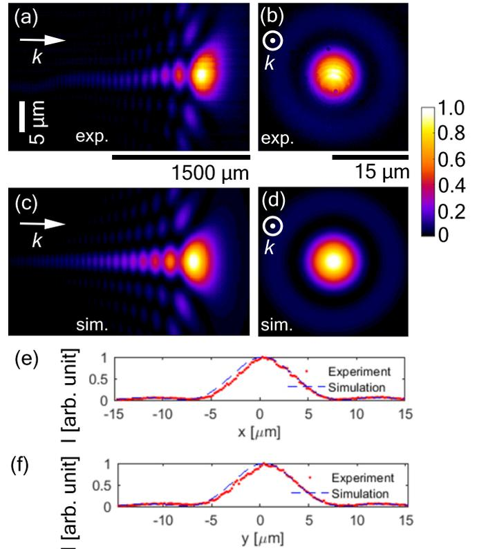
**Fig. 4.** Intensity distribution near the focus of a plano-convex lens in air with a Gaussian beam as the input. (a) Experimentally measured intensity along  $xz$  plane; (b) experimentally measured intensity at the focal plane; (c) simulated intensity along  $xz$  plane; (d) simulated intensity at the focal plane. Comparisons of the intensity profiles at the focal plane (e) along the x-axis; (f) along the y-axis.
