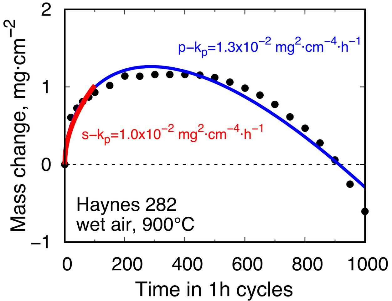
Figure 3 Schematic diagram of fitted mass change curve. The mass gain curve of Haynes 282 in wet air at  $900^\circ\text{C}$  in 1 hour cycle was fitted with the  $s-k_p$  and  $p-k_p$  models, respectively.
