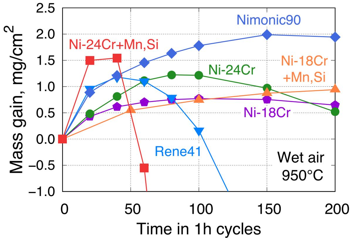
Figure 2 **Snapshot of ORNL cyclic oxidation dataset.** Mass gain of select alloys as a function of oxidation time in 1 hour cycles. The cyclic oxidation of alloys can be significantly altered by minor alloying elements.
