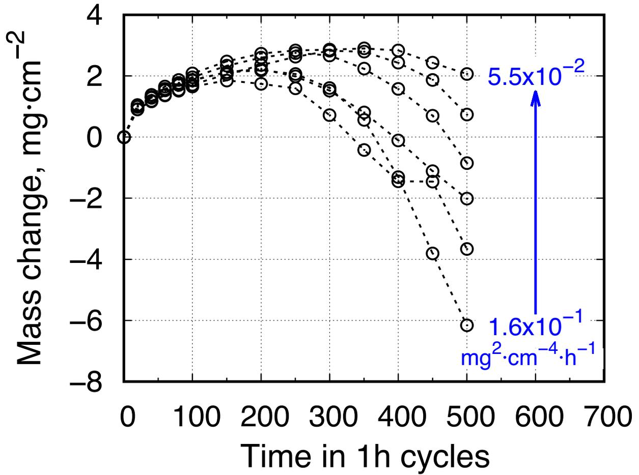
Figure 7 **Oxidation of Nimonic 80A at 950 °C in wet air in 1 hour cycle.** The  $k_p$  determined by the  $p-k_p$  model largely varies from six tests under the same condition, whereas the one from  $s-k_p$  does not.
