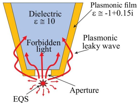
Fig. 23. Geometry of the problem of EQS radiation in the presence of a nanohole in a scanning microscope (SNOM) tip.
