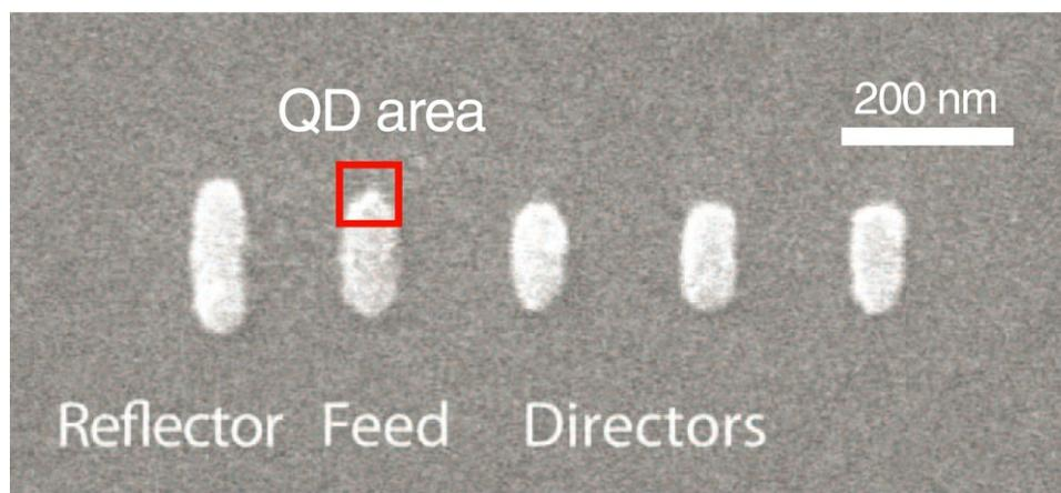
Fig. 19. An optical nanoantenna of the Yagi-Uda type based on gold nanoparticles. The red square shows the region where the emitting CdSeTe/ZnS quantum dots were deposited [132].
