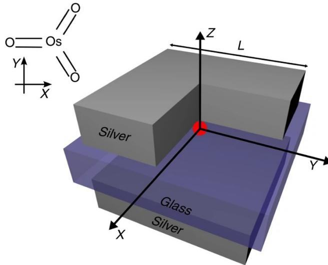
Fig.24. A patch nanoantenna to control allowed and forbidden transitions in  $\text{OsO}_3$ . The nanoantenna consists of two silver cuboids 50 nm thick and edge  $L$ . The cuboids are separated by a dielectric spacer ( $\epsilon = 2.25$ ) 30 nm thick and side  $L + 20$  nm. The emitting  $\text{OsO}_3$  molecule is located in the center of the antenna [144].
