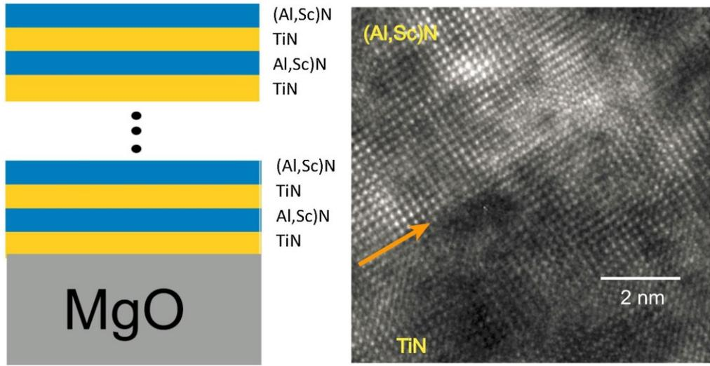
Fig. 46. A hyperbolic metamaterial formed by 5 nm thick TiN-Al<sub>0.72</sub>Sc<sub>0.28</sub>N layers. a) Geometry of the sample, b) HRTEM image of the interface between the layers. Adapted from [191].
