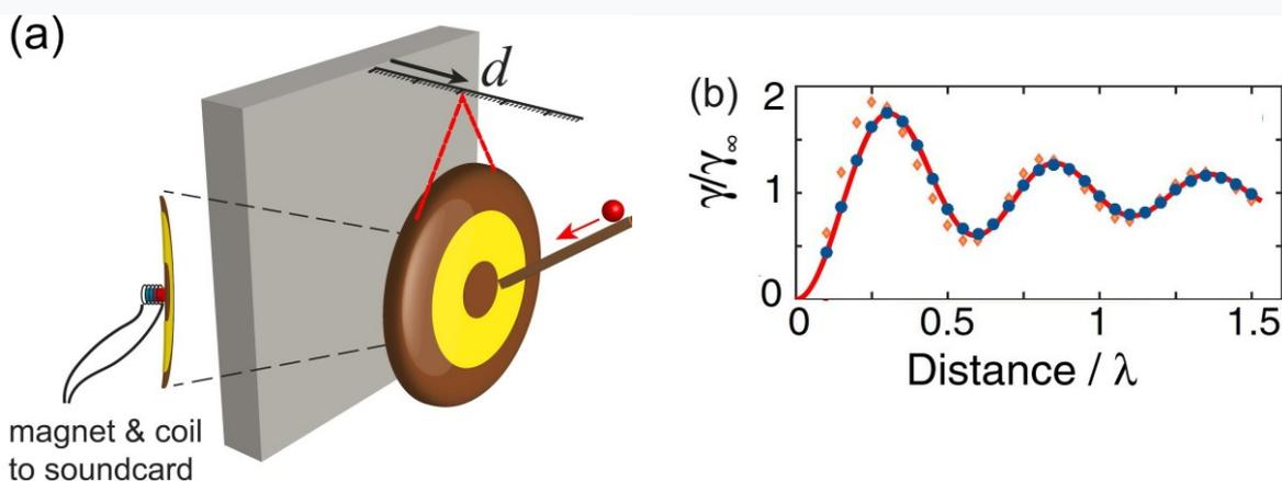
Fig. 53. A schematic of an experiment to measure the linewidth of the sound of a Chinese gong made of brass with the radius of 10 cm and the thickness of 0.5 mm, depending on the distance to the wall. b) Linewidth of the 306 Hz mode versus the distance of the gong from the wall. Orange circles - individual measurements, blue dots - averaging over 5 measurements, solid curve – theory [212].
