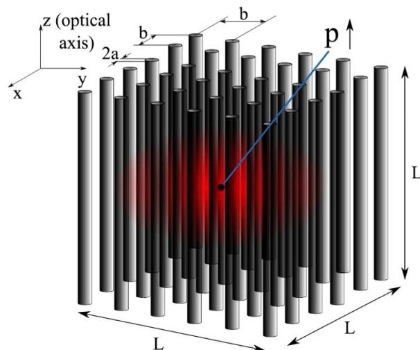
Figure: 50. a) A HMM waveguide of gold nanorods ( $d = 38$  nm,  $H = 150$  nm, period  $P = 80$  nm), the space between the nanorods is filled with one of 4 dyes (R590, R610, R640, LD700) in a PMMA matrix [206]; b) a finite lattice of infinite (in  $z$  direction) LiTaO<sub>3</sub> nanowires with the radius  $a = 32$  nm, the period  $b = 200$  nm [207].
