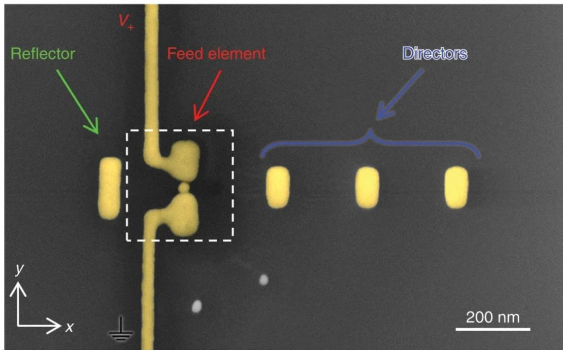
Fig. 2. A nanoscale light source based on an electrically-driven Yagi-Uda nanoantenna [32].
