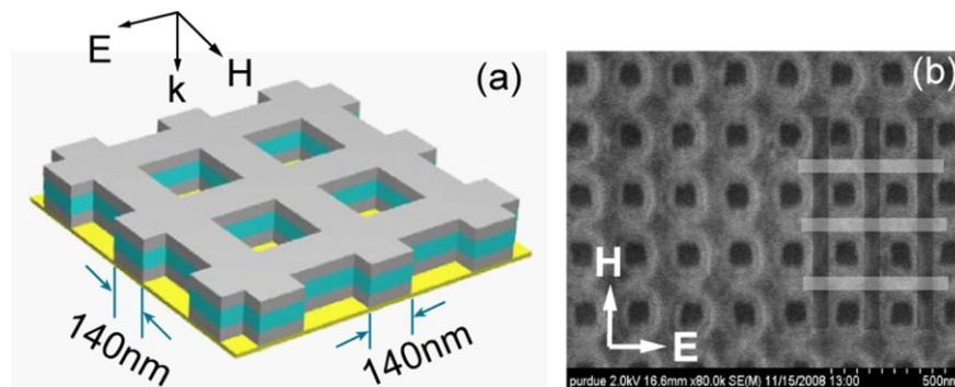
Fig. 36. (a) Schematic and (b) SEM images of a metamaterial formed by perforated layers of  $\text{Al}_2\text{O}_3$  (45 nm, middle) and Ag (43 nm, top and bottom) and having a negative refractive index at  $\lambda = 580$  nm [170].
