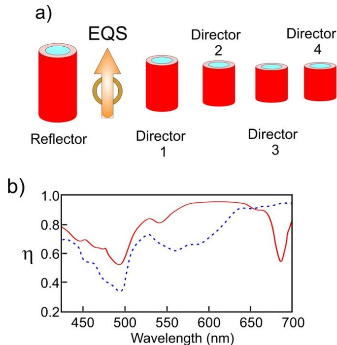
Fig. 20. a) Geometry of a hybrid plasmon-dielectric antenna [136]; b) radiation efficiency  $\eta$  of such a nanoantenna (red curve, [136]) in comparison with that of an all-dielectric nanoantenna (blue dashed curve, [3]).
