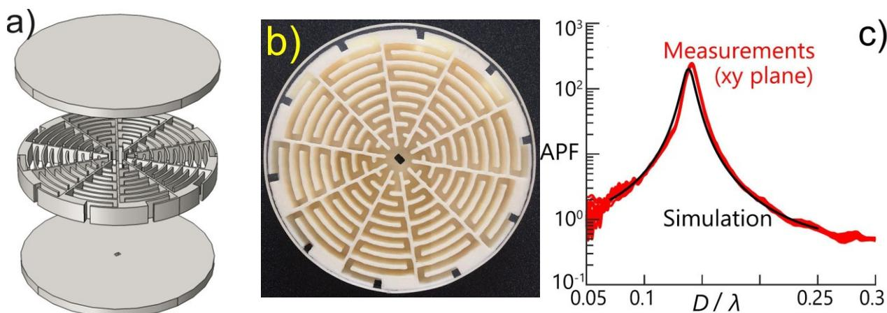
Fig. 54. a) Geometry of the experimental sample, where the main element is a 10 cm diameter nanometadisk made of plastic with zigzag nanochannels, excited by a monopole source of 1 mm in diameter from below (b); c) the dependence of the acoustic Purcell factor (APF) on the wavelength (red - measurements in the plane of the disk at a distance of 15 cm from the center, black - calculation through the imaginary part of the Green's function) [214].
