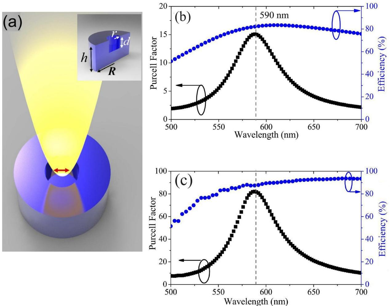
Fig. 34. a) Geometry of a dielectric nanostructure in the form of a silicon cylinder with a void to control the radiation of forbidden transitions; b), c) Purcell factors and radiation efficiencies for *ED* and *MD* transitions, respectively. b)  $R = 110$  nm,  $h = 86$  nm,  $d = 19$  nm,  $r = 25$  nm; c)  $R = 110$  nm,  $h = 80$  nm,  $d = 30$  nm,  $r = 25$  nm [160].
