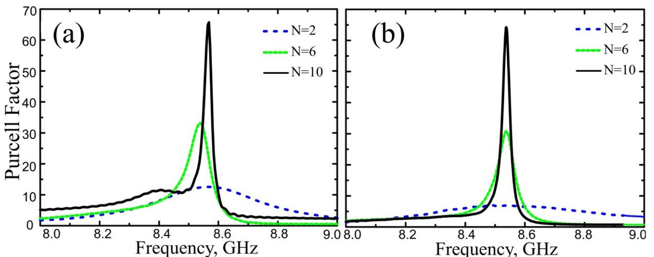
Fig. 31. Purcell factor for a microwave system shown in Fig.30. a) Theory, b) microwave experiment [158].  $N$  is the number of disks in the sample.
