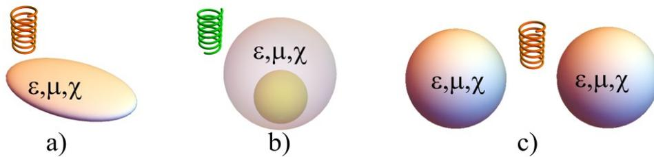
Fig. 44. Geometries of more complex chiral nanostructures for controlling the radiation of chiral molecules: a) a triaxial ellipsoid [87]; b) an asymmetric nanoparticle with a dielectric core and a chiral shell [186]; c) a chiral nanoantenna [88].
