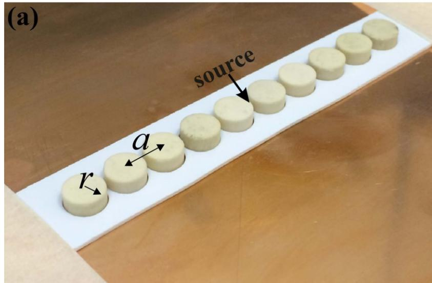
Fig. 30. Geometry of a microwave sample of disks of the radius  $r = 4$  mm, the height  $H = 4$  mm, and the period  $a = 5$  mm for experimental verification of the theory ( $\epsilon = 16$ ) [158].
