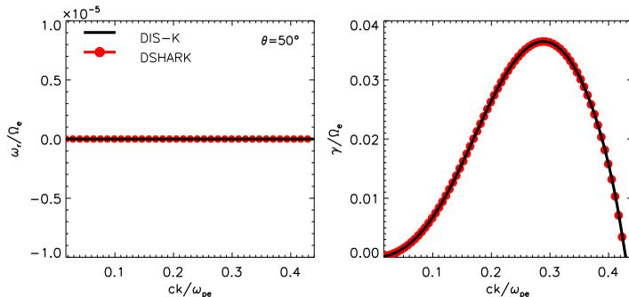
FIGURE 1. Unstable solutions of the aperiodic electron firehose instability at  $\theta = 50^\circ$ . In black are the solutions obtained with the new code, DIS-K, while red dots are obtained with DSHARK. Left panel shows the normalized (real) frequency,  $\omega_r/\Omega_e$  vs. the normalized wave number  $ck/\omega_{pe}$ , and right panel shows the normalized growth rate,  $\gamma/\Omega_e$  vs.  $ck/\omega_{pe}$ .
