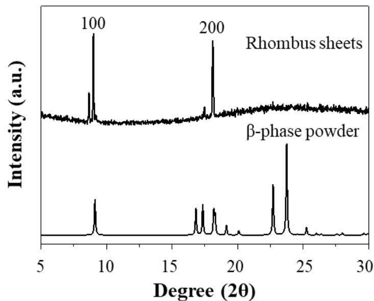
**Figure S1.** X-ray diffraction (XRD) of the  $\beta$ -phase perylene crystals (top) and powder (bottom). Two sharp peaks corresponding to the (100) and (200) crystal-face family for the  $\beta$ -phases perylene in the XRD pattern clearly indicates that the rhombus sheets are the  $\beta$ -phase crystal structure.
