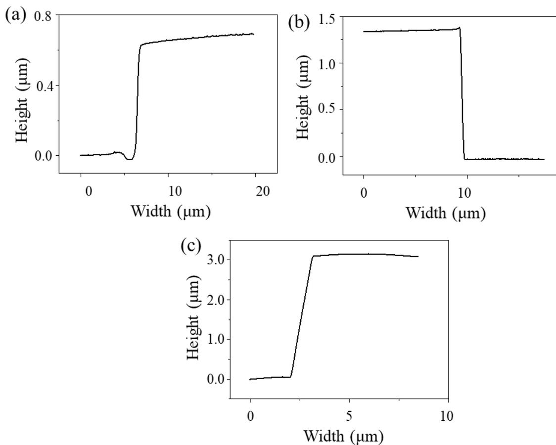
**Figure S3.** Atomic force microscope (AFM) of the  $\beta$ -phase perylene crystals. The thicknesses of these microcrystals were determined to be about 0.2 - 4  $\mu\text{m}$  according to the AFM measurements. (a-c) The typical thicknesses of the  $\beta$ -phase perylene crystals.
