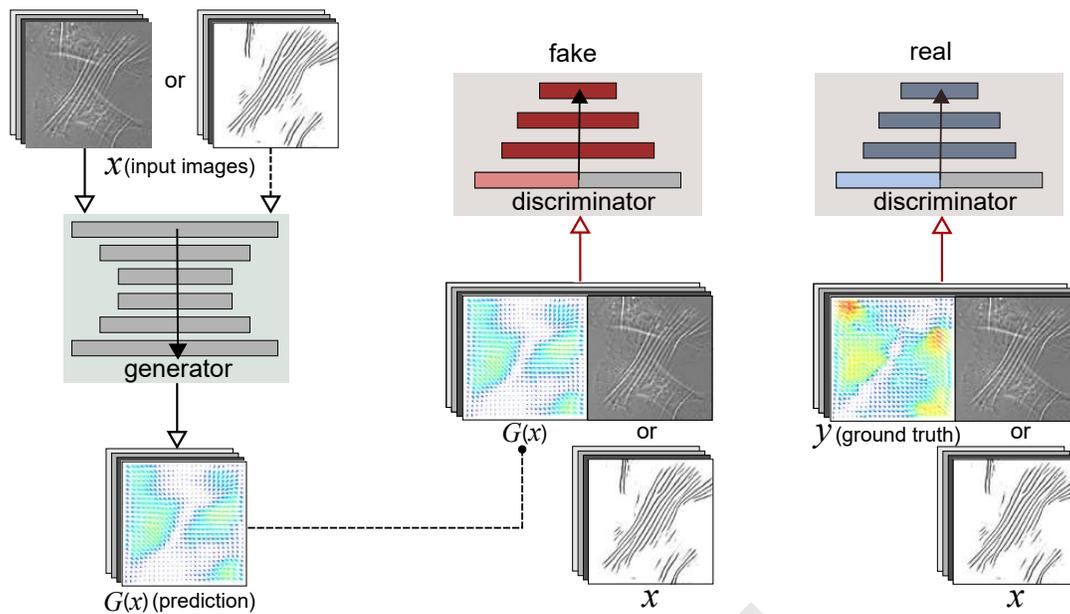
Fig. S1. Schematic showing the structure of GAN (generative adversarial network) utilized in the present work.
