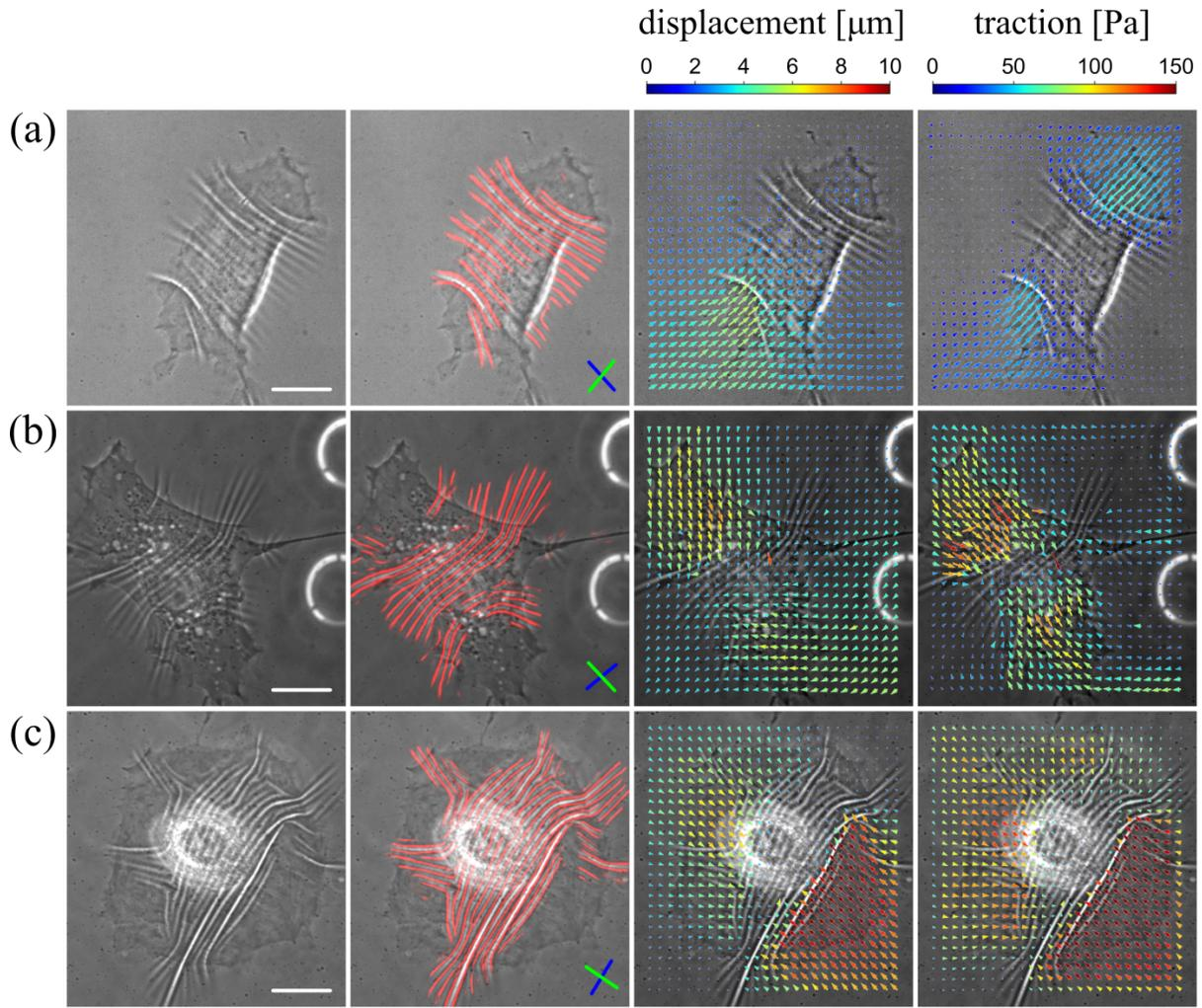
**Fig. 2.** Three examples of the simultaneous measurement of wrinkles and traction forces. Each column describes (from left to right) raw image, wrinkles (red lines), displacement field and traction force field. The white scale bar in the first column images is 20  $\mu\text{m}$ . The blue and green lines inside the second column images describe the principal direction of the wrinkle and the traction, respectively.
