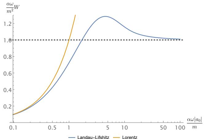
FIG. 1. Momentum transfer  $W$  (14), in a head-on collision with a Sauter pulse with  $a_0 < 0$ . Without RR, the momentum transfer is unbounded. With RR,  $W$  approaches a constant at large  $|a_0|$ , as RR effects dominate over the electric force.
