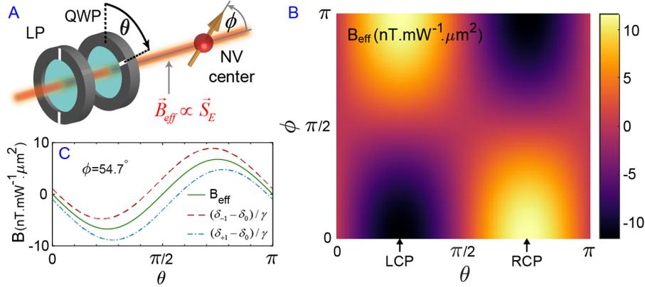
Fig. 2: Effective magnetic field induced by PSD. (A) A linear polarizer and a quarter wave plate control the PSD. (B) The effective field calculated for different QWP angles ( $\theta$ ) and alignment angles ( $\phi$ ). (C) The effective field calculated for an NV center in a (100) cut diamond,  $\phi = 54.7^\circ$ .
