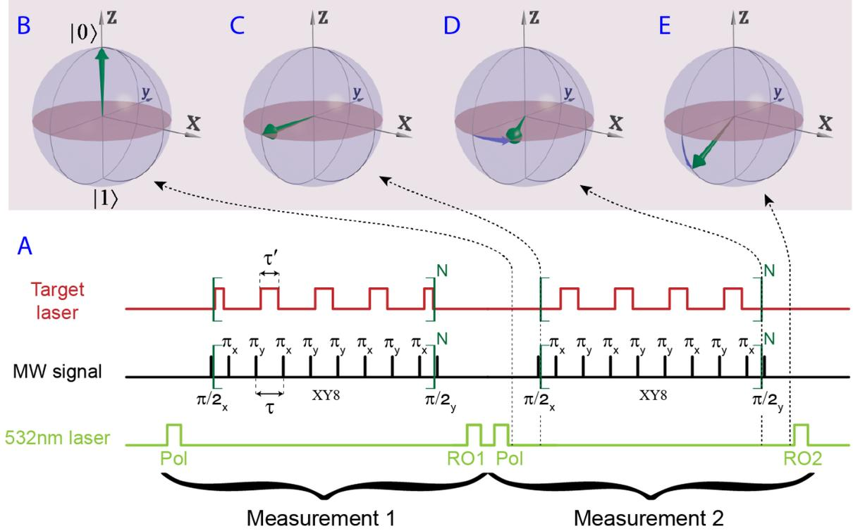
Fig. S4: (A) Pulse sequence used for measuring the PSD. In each measurement a pair of 532nm laser pulses initialize (polarizing) and readout the state of the NV center. During each measurement an XY8 MW pulse performs dynamical decoupling on the spin of the NV center. (B-E) Bloch sphere representation of the state of the qubit after polarization, before the XY8 pulse, after the XY8 pulse, and before readout. The PSD is generated by the target beam. RO, readout; Pol, polarizing.
