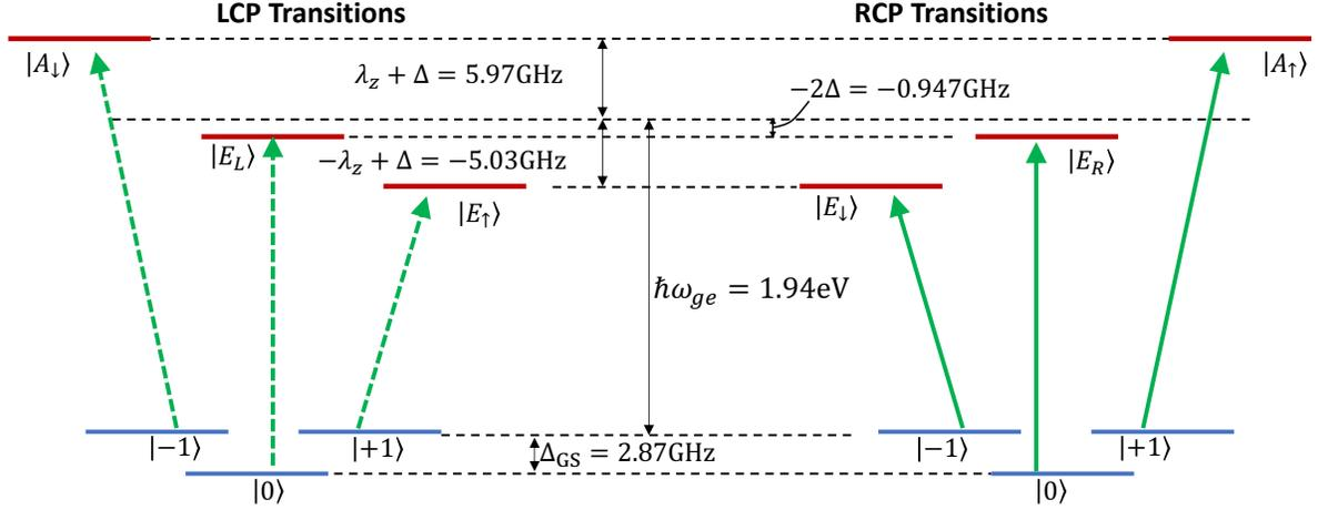
Fig. S1: Schematic of energy levels of the NV center. Here, there are no external magnetic field and strain. Left and right panels show the possible transitions induced by left circularly polarized (LCP) and right circularly polarized (RCP) lights.
