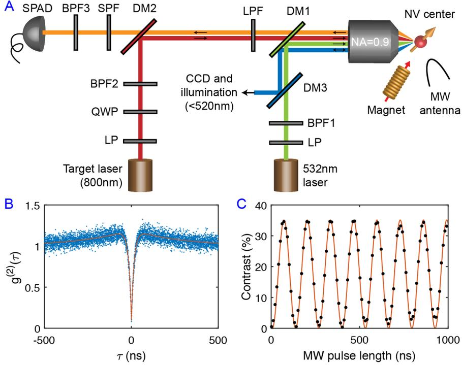
Fig. S3: Schematic of the experimental setup. (A) Schematic of the setup showing the beam paths and filters. (B) Second-order correlation measurement showing that the AFM tip contains a single NV center. (C) Rabi oscillations showing the interaction of the microwave beam (MW) with the NV center. LP, linear polarizer; DM, dichroic mirror; BPF, band-pass filter; LPF, long-pass filter; SPF, short-pass filter; QWP, quarter-wave plate.
