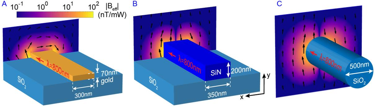
Fig. 4: Effective field sensed by an NV center near optical waveguides. A plasmonic waveguide (A), a ridge waveguide (B), and an optical fiber (C) all producing transverse effective fields due to the PSD of their evanescent fields. The direction of the effective field is shown with black arrows and its amplitude with the colormap. The mode of the ridge waveguide is transverse electric (TE) and the mode of the optical fiber is  $\hat{x}$  polarized  $HE_{11}$ .
