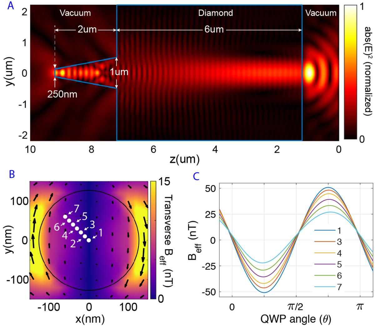
Fig. S5: Numerical simulations for the effective field amplitude in an AFM tip. (A) Amplitude of the electric field in an AFM tip made of diamond. (B) Amplitude and direction of the transverse component of the effective field in the plane of the NV center. (C) The effective field seen by an NV center with direction  $\hat{n} = (\hat{x} + \hat{y} - \hat{z})/\sqrt{3}$  placed at various locations shown in panel B with white dots.
