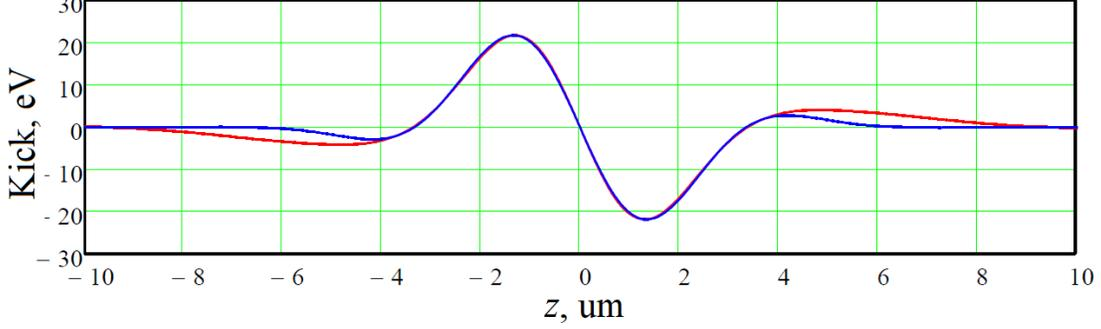
FIG. 3. The energy kick (eV) after the "Kicker" section as a function of the proton's longitudinal position  $z = R_{56}x$  ( $\mu\text{m}$ ) with respect to the reference on-energy proton. The red curve is a calculated wake, based on Ref. [8, Eq. C7]. The blue curve is the proposed approximation, Eq. (1).
