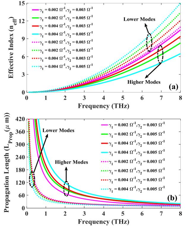
Fig. 8. Analytical results of plasmonic features for the second structure for various chirality values of two chiral layers: (a) the effective index as a function of frequency for lower and higher hybrid modes, (b) the propagation length as a function of frequency for lower and higher hybrid modes. The chemical potential of graphene sheets is  $0.35$  eV.
