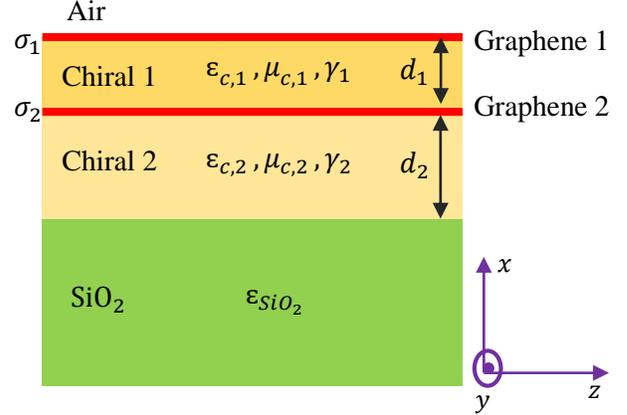
Fig. 7. The cross-section of the hybrid graphene-based waveguide with two chiral layers.
