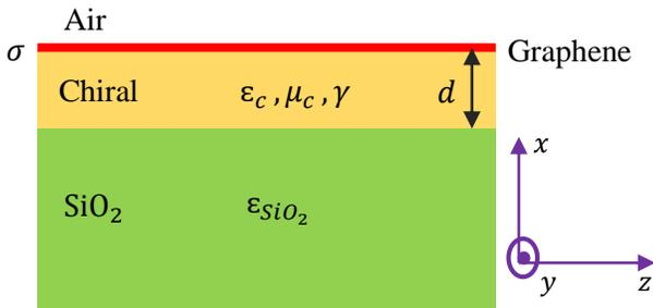
Fig. 3. The cross-section schematic of the first structure. The graphene sheet has been deposited on the chiral-SiO<sub>2</sub> layers.
