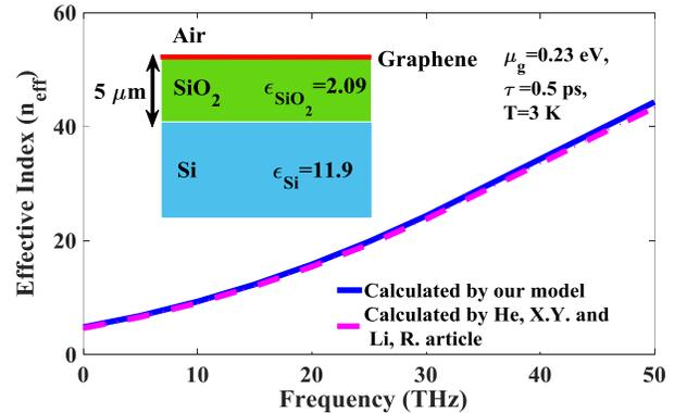
Fig. 2. The effective index of TM mode as a function of frequency for achiral waveguide constituting Air-SiO<sub>2</sub>-Si layers, prepared by our analytical model and the results of [72]. The simulation parameters have been indicated in the diagram.
