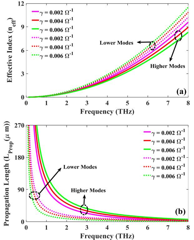
Fig. 4. Analytical results of plasmonic features for the first structure for various chirality values: (a) the effective index as a function of frequency for lower and higher hybrid modes, (b) the propagation length as a function of frequency for lower and higher hybrid modes. The chemical potential of graphene sheets is  $0.35\text{ eV}$ .
