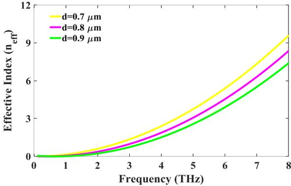
Fig. 6. The effective index of higher mode for the first structure for various chiral thicknesses ( $d = 0.7, 0.8, 0.9 \mu\text{m}$ ). The chemical potential of the graphene sheet is  $0.35$  eV and the chirality of the chiral medium is  $0.002 \Omega^{-1}$ .
