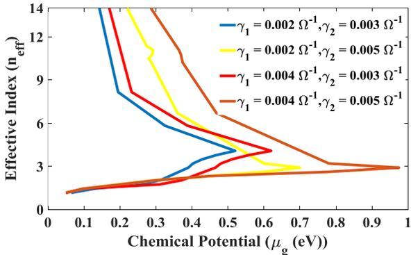
Fig. 9. The effective index of hybrid modes as a function of the chemical potential at the frequency 6 THz.
