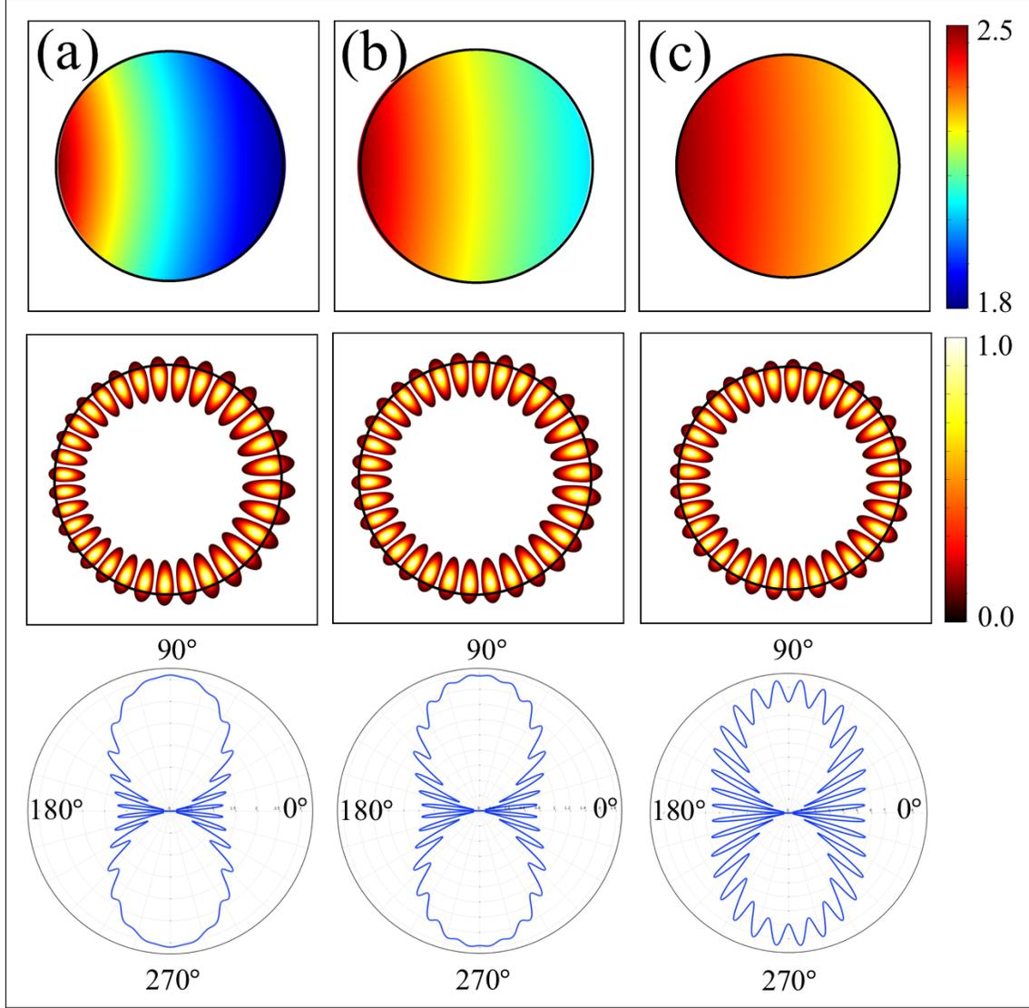
FIG. 3: Refractive indices (top), near field intensity patterns (middle), and far field intensity patterns (bottom) of the resonant modes in limaçon-shaped transformation cavities for (a)  $(r, \epsilon) = (1.0, 0.081)$ , (b)  $(r, \epsilon) = (0.4, 0.125)$ , and (c)  $(r, \epsilon) = (0.2, 0.152)$ .
