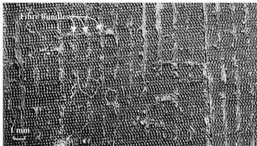
Figure 5 : Macrography of the heat sink after tests at 18 \text{ MW/m}^2 (the defective tile was removed in laboratory)
