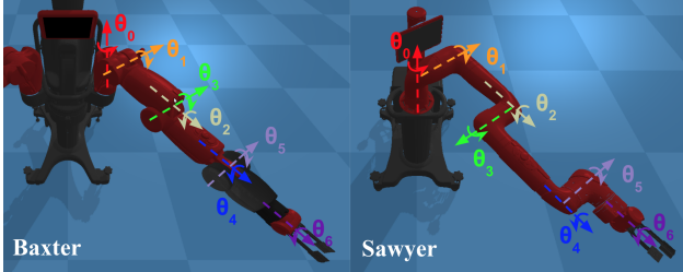
Figure 5: The arm of the Baxter robot and the Sawyer robot, used in the MIME dataset and Roboturk dataset respectively. They share a similar structure, 7 joints and one end effector.
