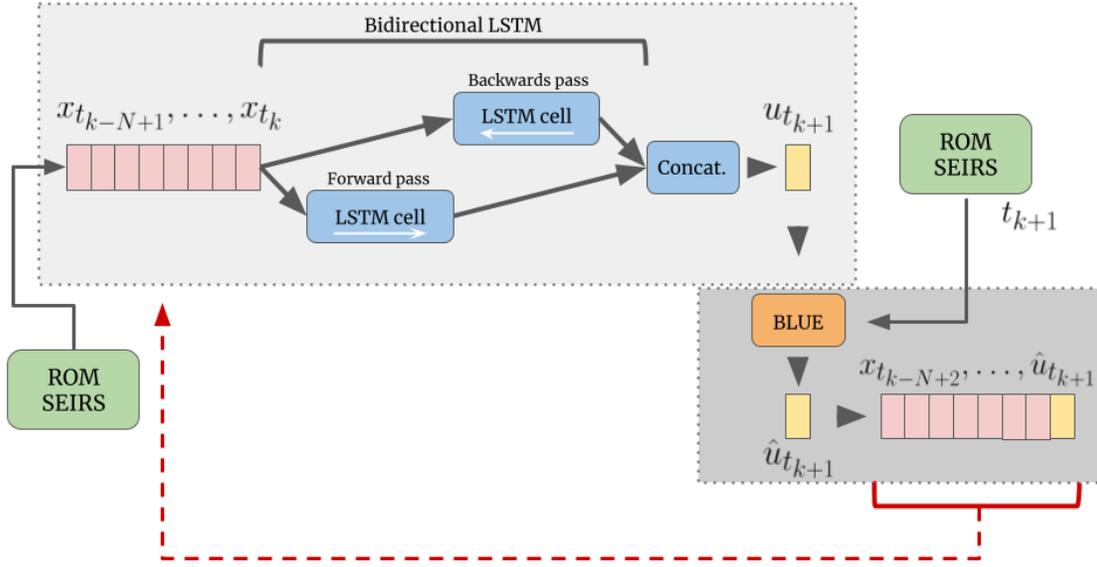
Figure 3: Predictive LSTM  $f^{BDLSTM+BLUE}$  for a sequence of two time levels. Top-left: off-line bidirectional LSTM network. Bottom-right: data-correction of the prediction. The Best Linear Unbiased Estimation (BLUE) is used to data-correct the prediction of the network. One time level corresponds to 10 time-steps of the original SEIRS solution.
