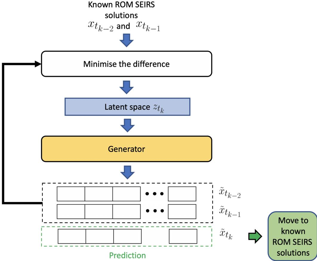
Figure 4: Workflow of  $f^{PredictiveGAN}$  for a sequence of three time levels ( $N = 3$ ). Adapted from Silva et al. [52].
