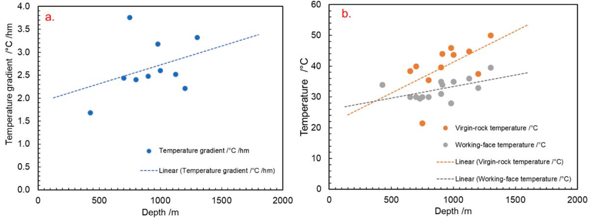
Fig. 10 Evolution of underground temperature over the increase of excavation depth of deep coal mines including (a) temperature gradient of the formation, and (b) virgin-rock temperature, and working-face temperature.
