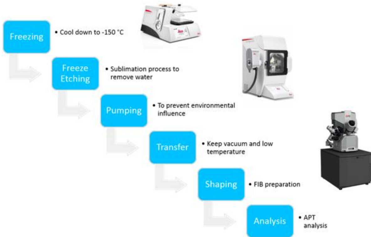
Figure 5: workflow adopted for the analysis of frozen liquids on wire blanks.
