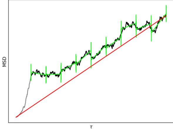
Figure 7. Schematic comparison between the conventional and CHAMPION methods for assessing D from MSD. Conventionally (red) D is based on the MSD for the longest available interval. CHAMPION (green) instead first identifies the diffusive part of the MSD curve (black) and computes D based on averaging the slope of the MSD over the whole range of \tau > \tau_D .
