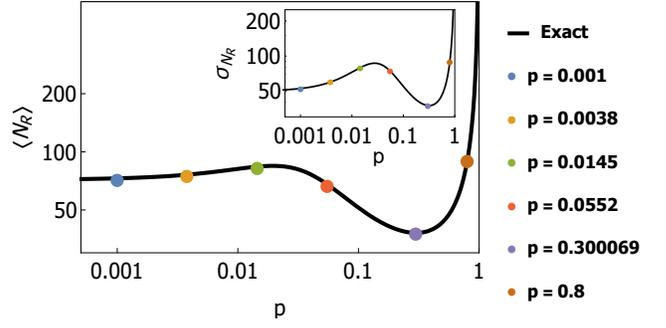
FIG. 7. Comparison between exact and simulation results for mean and standard deviation for a biased RW in confinement subject to restart conducted at a probability  $p$ . Parameters for the current set-up: left boundary  $= 1$ , right boundary  $= 25$ , initial position  $n_0 = 3$ , diffusive parameter  $q = 0.7$ , and bias  $g = 0.3$ .
