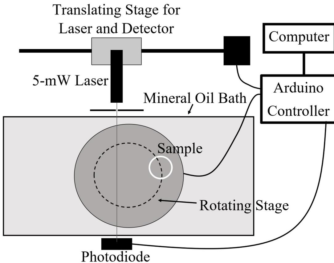
FIG. 2. Diagram of CT Scanner used in this experiment
