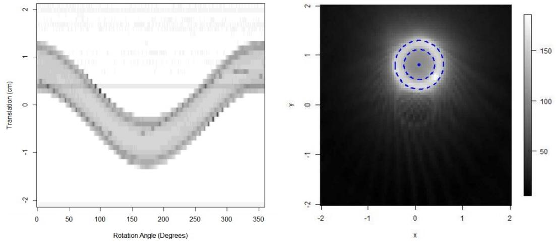
FIG. 4. The left image displays the sinogram while the right image displays the reconstructed image. The tube was imaged with a purple laser using 1 mm, 0.9 degree steps. Dashed lines indicate the detected boundaries of the tube and the point indicates the centroid.
