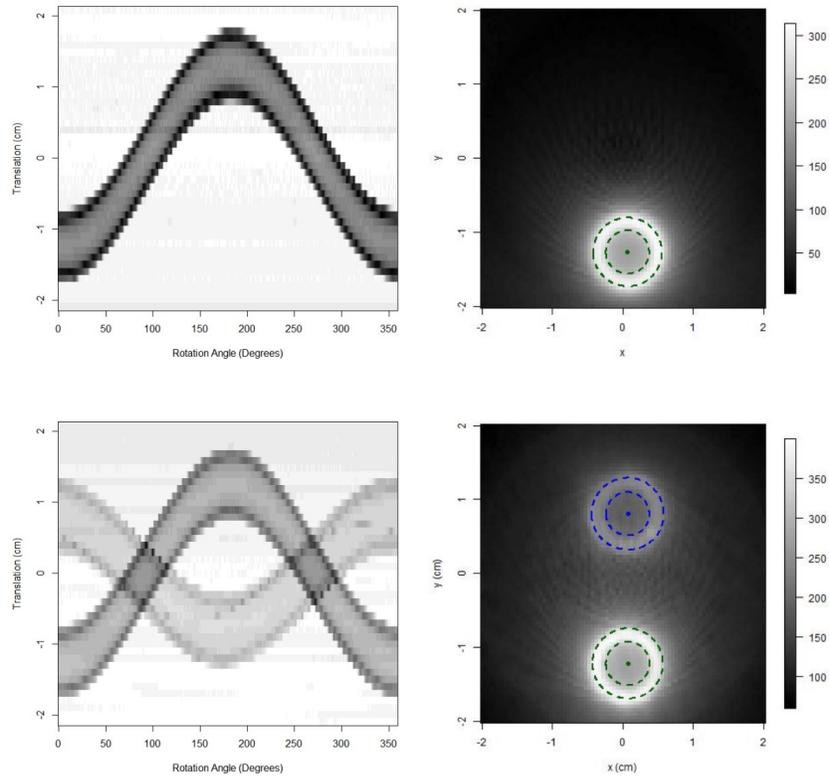
FIG. 5. Dark green and blue Pyrex tubes imaged with 1 mm translations and 0.9 degree rotations. Left shows the sinogram while right indicates detected inner and outer radii on the reconstructed images.
