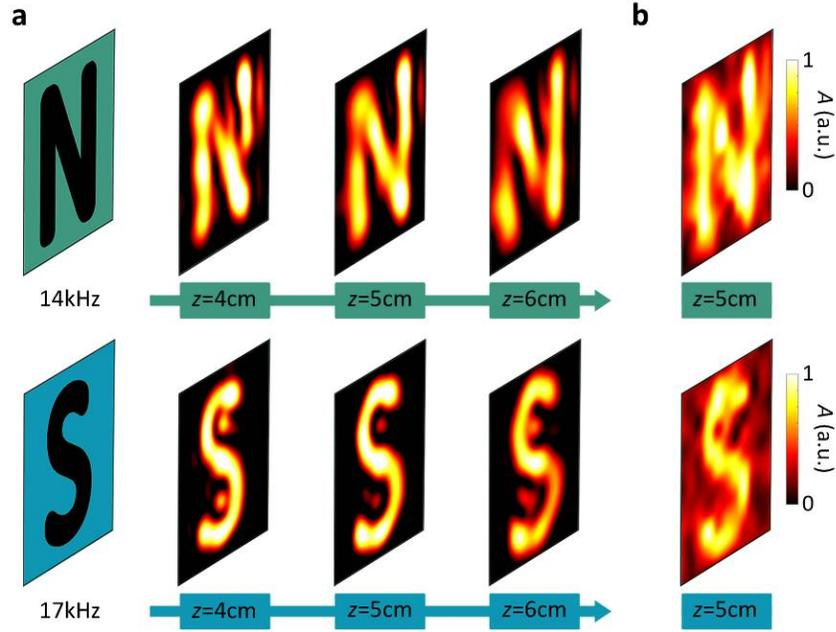
**Fig. 4** Simulated and experimental results of holographic images (letter “N”) at 14 kHz and (letter “S”) at 17 kHz, respectively. (a) The simulated acoustic intensity distributions at the distance of  $z = 4$  cm,  $z = 5$  cm,  $z = 6$  cm, respectively. The arrows indicated the wave is propagating along the  $z$ -direction. (b) The measured acoustic intensity distributions at the predesigned image plane of  $z = 5$  cm.
