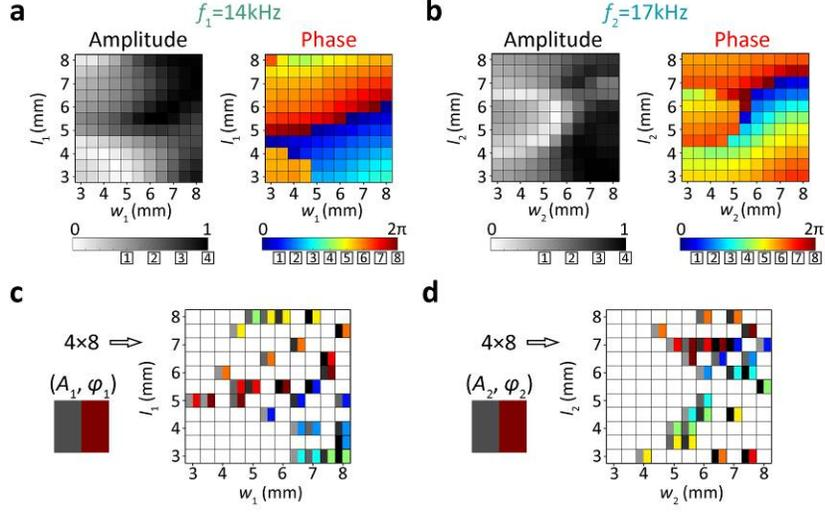
**Fig. 2** Amplitude and phase responses of the unit cell for 14 kHz and 17 kHz. **(a)** The amplitude and phase responses as a function of the parameters  $w_1$  and  $l_1$  for  $f_1 = 14$  kHz. **(b)** The  $4 \times 8$  combinations of  $(A_1, \varphi_1)$  varying with  $w_1$  and  $l_1$ . **(c)** The amplitude and phase responses varying with parameters  $w_2$  and  $l_2$  for  $f_2 = 17$  kHz. **(d)** The  $4 \times 8$  combinations of  $(A_2, \varphi_2)$  varying with  $w_2$  and  $l_2$ .
