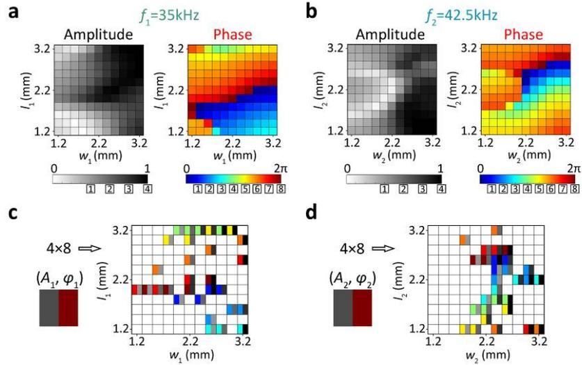
**Fig. 5** Amplitude and phase responses of the unit cell for 35 kHz and 42.5 kHz. (a) The amplitude and phase responses changing with parameters  $w_1$  and  $l_1$  for  $f_1 = 35$  kHz. (b) The  $4 \times 8$  combinations of  $(A_1, \varphi_1)$  varying with  $w_1$  and  $l_1$ . (c) The amplitude and phase responses varying with parameters  $w_2$  and  $l_2$  for  $f_2 = 42.5$  kHz. (d) The  $4 \times 8$  combinations of  $(A_2, \varphi_2)$  changing with  $w_2$  and  $l_2$ .
