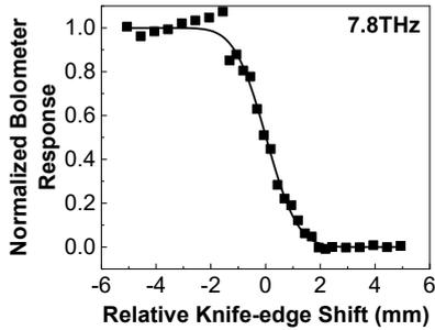
FIG. 2. Knife-edge measurements of the generated THz beam at 3 cm from the exiting Si window. The solid line is a fit to the data (black squares) with the error function, which is the integration of a Gaussian beam profile along the radial direction. The knife edge is placed after the Si window but before any other optics.
