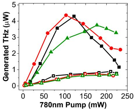
FIG. 4. Generated powers of 3.3 THz (open symbol) and 7.8 THz (filled symbol) as a function of the 780 nm pump power for the 515 nm laser powers of 10 mW (green triangle), 12 mW (red circle), and 15 mW (black square). The input pump beams are in the collimated configuration. The detunings of both pump lasers are kept at the values that produce maximum THz power. The solid lines are a guide for the eye.
