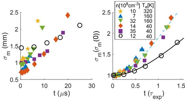
FIG. 5. Evolution of the RMS mean plasma size ( $\sigma_m$ ) with time. Open and closed symbols correspond to Gaussian and exponential plasmas respectively. Initial peak density and electron temperature is indicated in the legend. Size and time are unscaled (left) and scaled (right) by initial size and expansion time (Eq. 8) respectively. Fit lines correspond to Eq. 10 with  $\beta = 1$  (solid) and  $\beta = 0.63$  (dashed).
