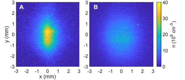
FIG. 3. False color images showing expansion of an exponential plasma with initial peak density  $4.4 \times 10^9 \text{ cm}^{-3}$  and  $T_e(0) = 40$  K. (A)  $t = 350$  ns after plasma creation. (B)  $t = 11 \mu\text{s}$  after plasma creation.
