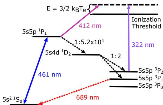
FIG. 1. Levels and transitions for laser cooling of strontium atoms and subsequent photoionization to form an UCNP.
