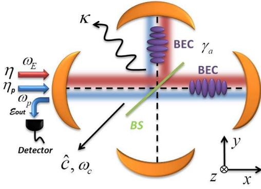
FIG. 1. The schematic diagram of a four mirror cavity with two transversely coupled Bose-Einstein condensates, oriented along  $x$ -axis and  $y$ -axis. Two lasers, an external pump and a probe, drive the cavity and generate coupling between atomic states after splitting from beam splitter (BS).  $\eta$  ( $\omega_E$ ) and  $\eta_p$  ( $\omega_p$ ) correspond to the intensities (frequencies) of the external pump and probe lasers, respectively.
