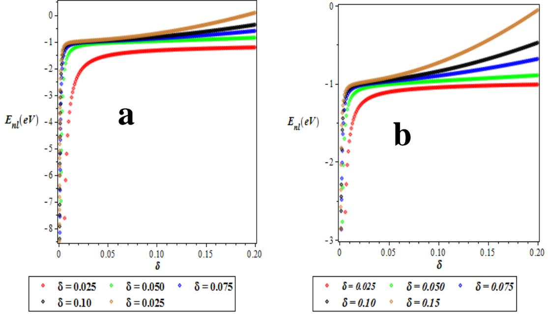
FIGURE 6(a). Variation of the ground state energy spectrum for various  $l$  as a function of the screening parameter( $\delta$ ) (b). A plot of the first excited state energy spectrum for different  $l$  as a function of the screening parameter( $\delta$ ). We choose  $a = b = -1$ ,  $c = 0.025$ , and  $\delta = 0.025$  for the ground and excited states
